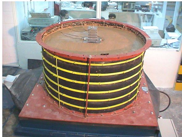
Figure3. Experimental SFSI model installed on the shaking table
