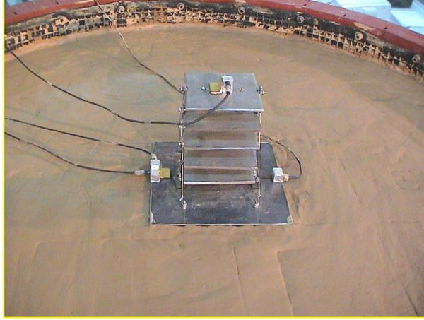
Figure4. Accelerometers arrangement on the top and bottom level of 5 story structural model
