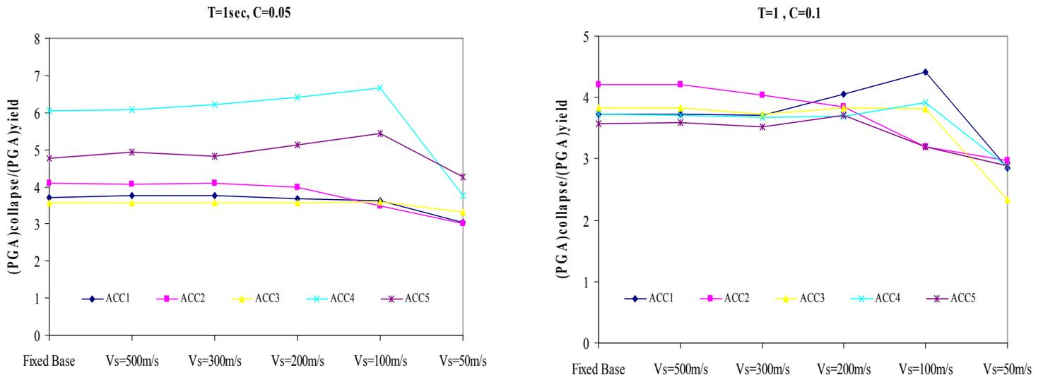
Figure 6. Effect of foundation flexibility on force reduction factor of 5-story generic model a)  $T=1$  sec,  $C=0.05$  ,b)  $T=1$  sec,  $C=0.1$
