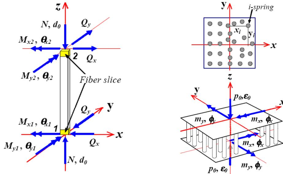
Figure 3. Fiber elements forces and deformations
