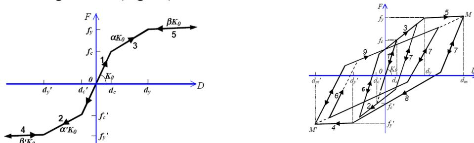
Figure 2. Non-linear behaviour of RC structural elements: a) backbone curve b) hysteretic loop
