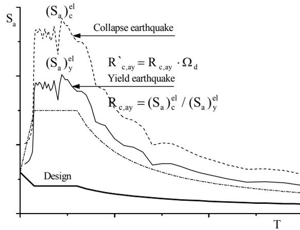
Figure 1. Evaluation of the force reduction factor by definition of  $R_{c,ay}$  and  $\Omega_d$  [Wafi and Elnashai, 2002]
