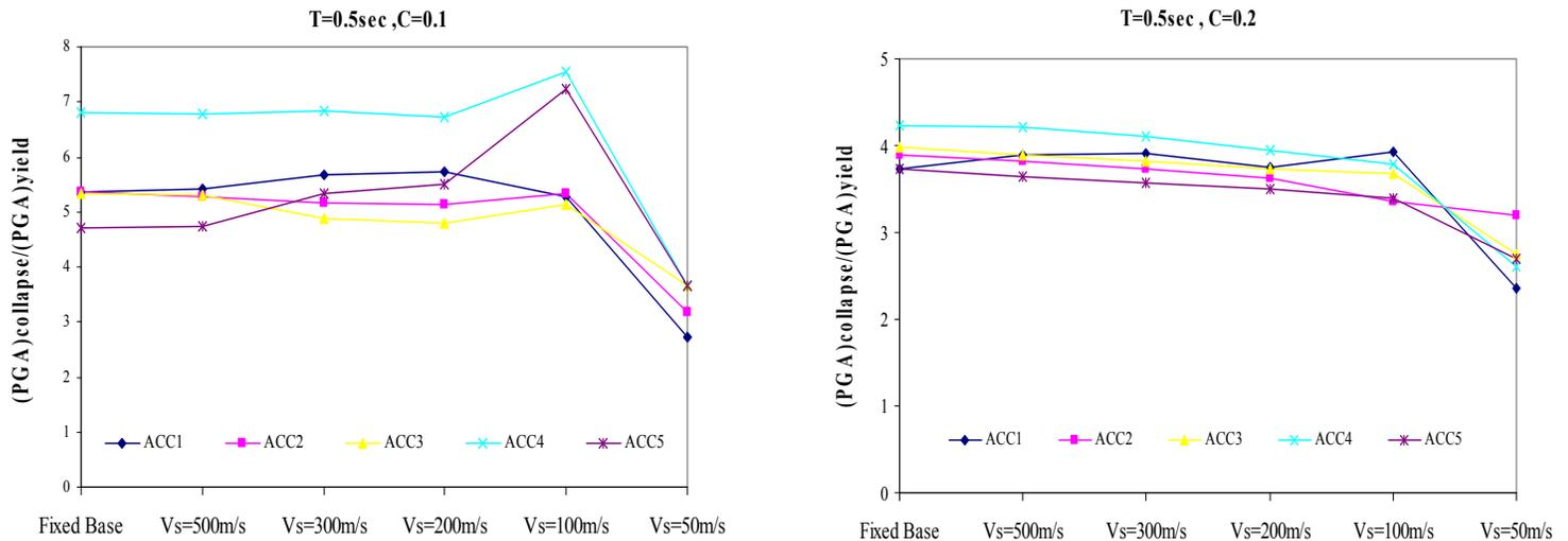
Figure 5. Effect of foundation flexibility on response reduction factor of 5-story generic model a)  $T=0.5$  sec,  $C=0.1$  ,b)  $T=0.5$  sec,  $C=0.2$
