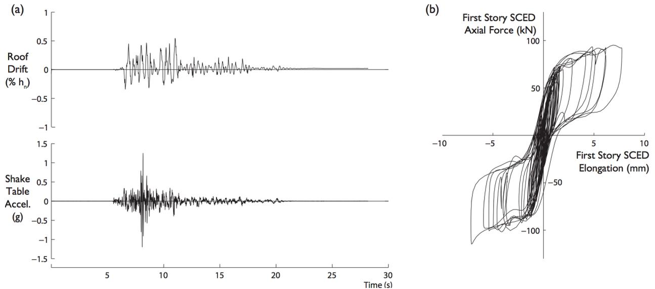
Figure 11. Response from shake table experiments under a DBE record 1-4: 1966 Parkfield - cs08: a) Roof displacement time history and shake table acceleration record b) First-story shear-story drift response.
