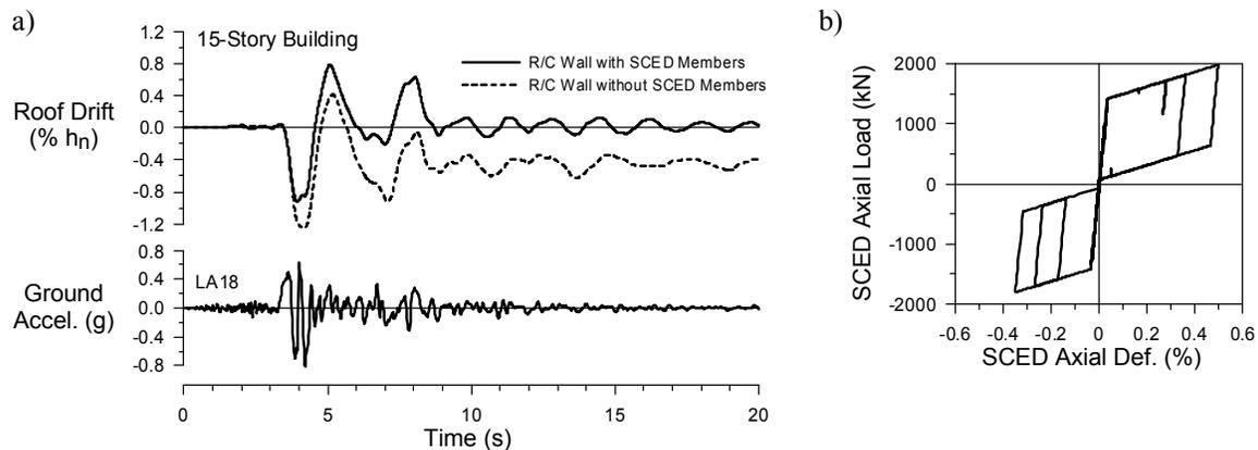
Figure 7. Seismic response of a 15-story R/C wall with and without SCED members: a) Roof displacement time histories; b) SCED member hysteretic response.
