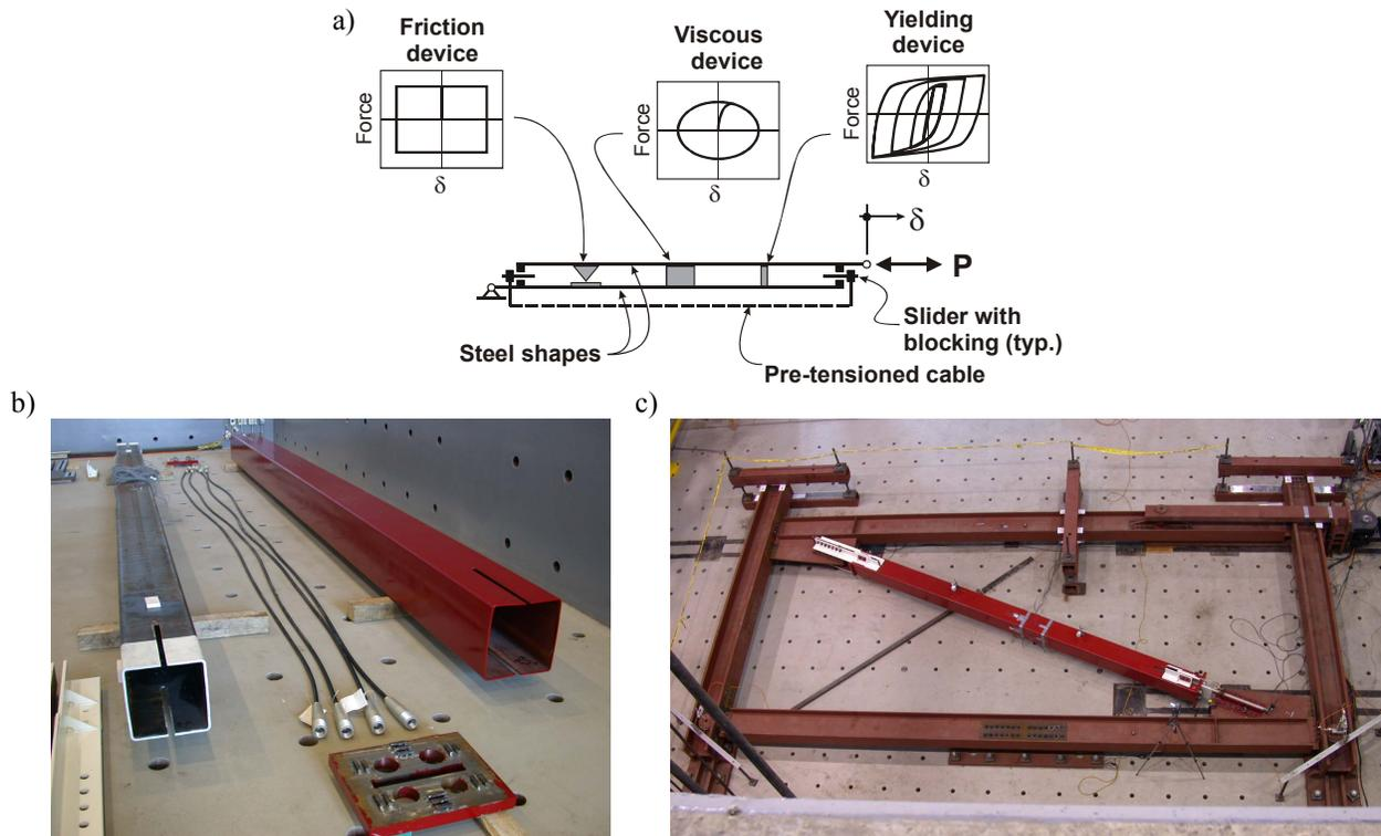
Figure 2. a) Schematic of the SCED bracing member system; b) Components of a SCED brace prior to assembly; and c) SCED brace in a full-scale frame test setup.
