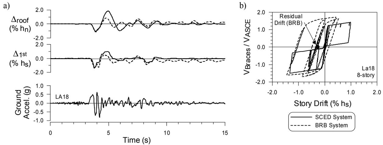
Figure 4. Computed responses of 8-story SCED and BRB frames under a DBE ground motion record: a) Roof displacement and first story drift time histories; b) Story shear-story drift response at Level 1.
