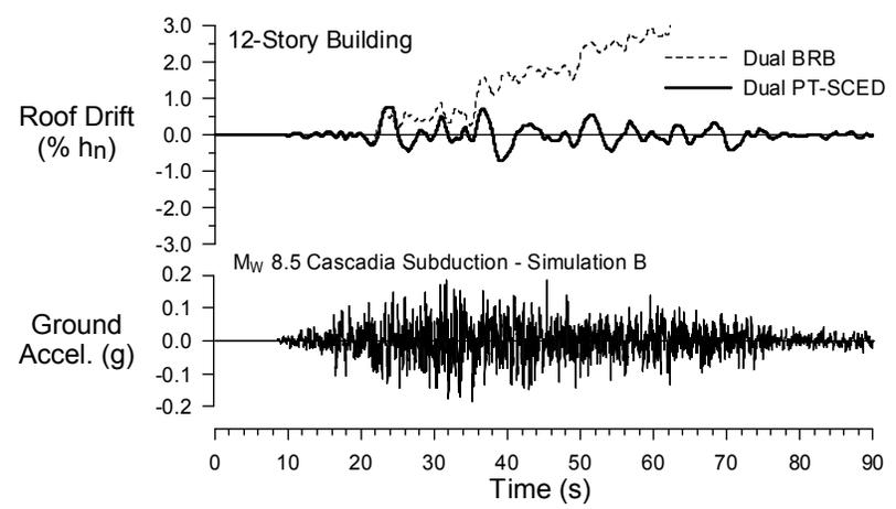
Figure 6. Roof displacement time history of 12-story dual braced frames with BRB and SCED bracing members under a Cascadia subduction earthquake ground motion.
