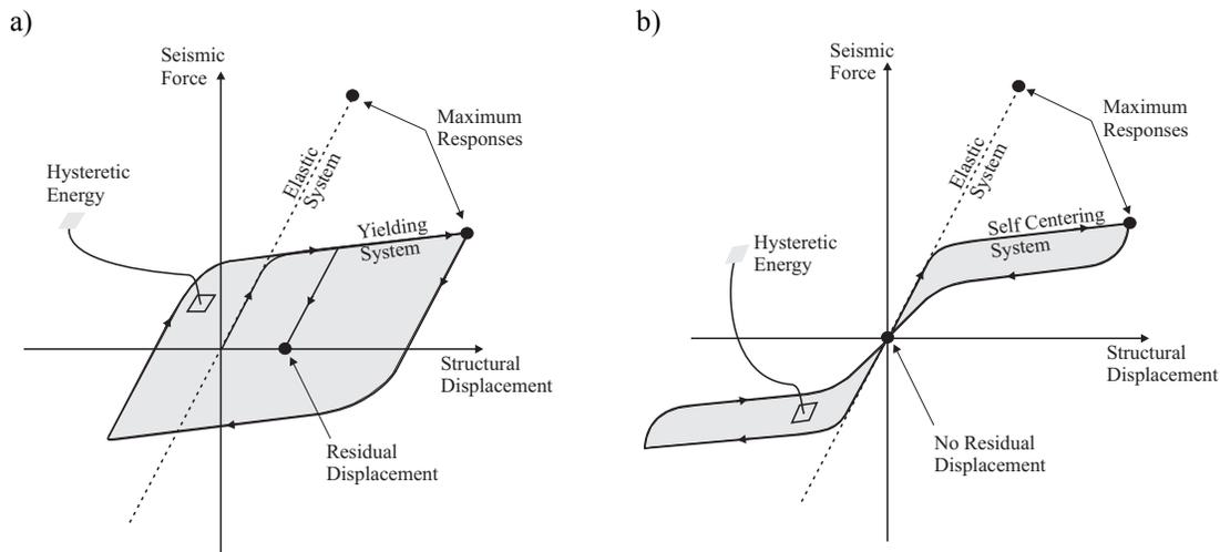
Figure 1. Nonlinear hysteretic response to earthquakes: a) Yielding systems; b) Self-centering energy dissipation systems.
