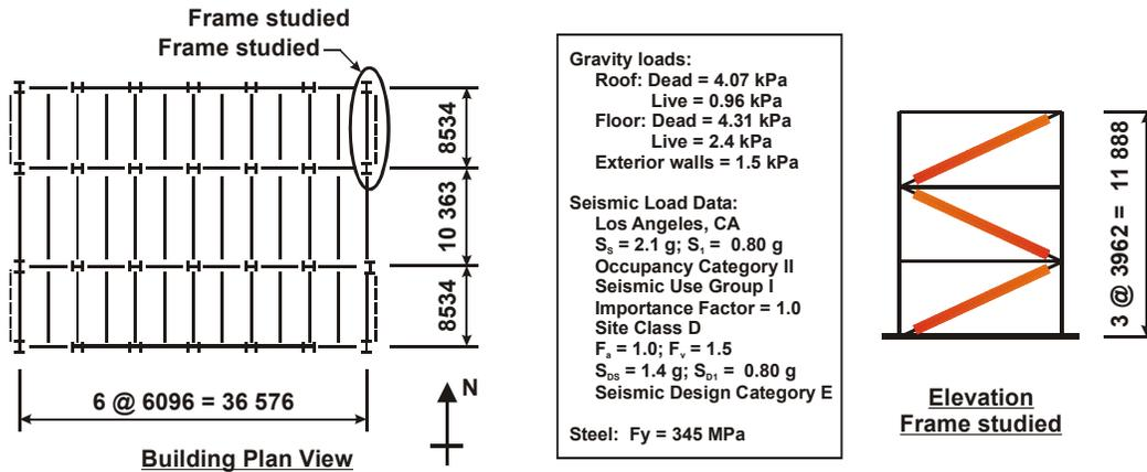
Figure 8. Three-story prototype building and design loads for the shake table test program.
