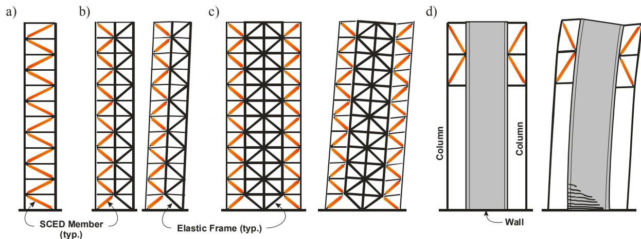
Figure 3. a) SCED braced frame; b) and c) Dual SCED braced frame; and d) SCED bracing acting in parallel with a reinforced concrete shear wall.
