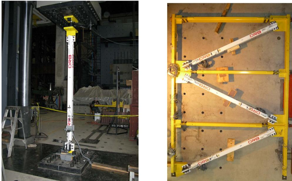
Figure 9. Shake table test program: a) SCED brace specimen subjected to quasi-cyclic characterization test; b) Test SCED braced frame upon assembly.
