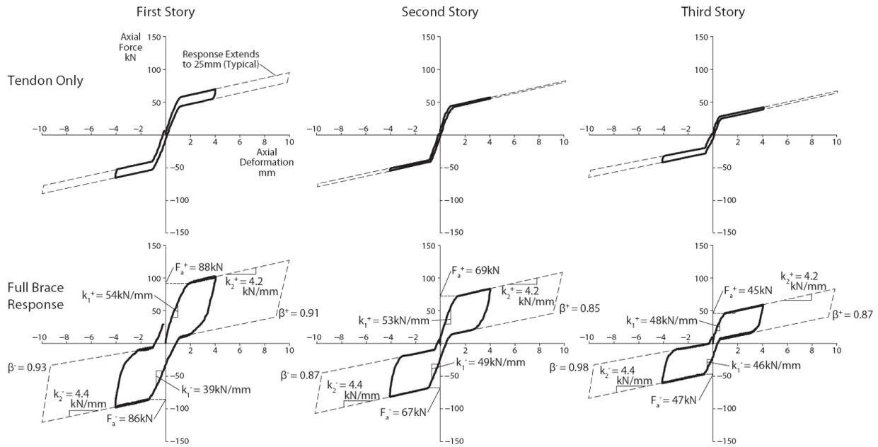
Figure 10. Hysteretic responses of the SCED brace specimens from the characterization tests performed without and with the brace’s internal energy dissipation mechanisms.
