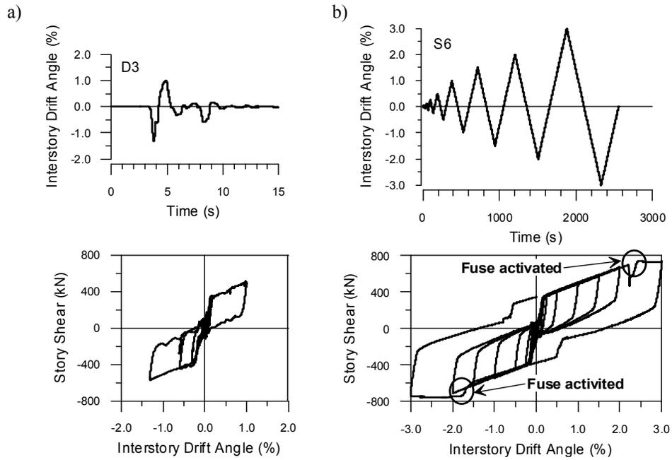
Figure 5 Story shear-drift response of the braced SCED frame in Fig. 2c under: a) Story drift time history at Level 1 of the 8-story structure under DBE ground motion (see Fig. 4); b) Cyclic quasi-static loading with stepwise incremental displacement amplitude.
