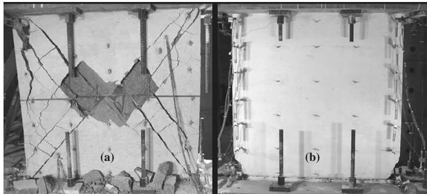
Figure 2. Typical failure mode. (a) Type 1 wall at 2.0% lateral drift (typical for types 1, 2, 3, 5), (b) Type 4 wall at 3.0% lateral drift.
