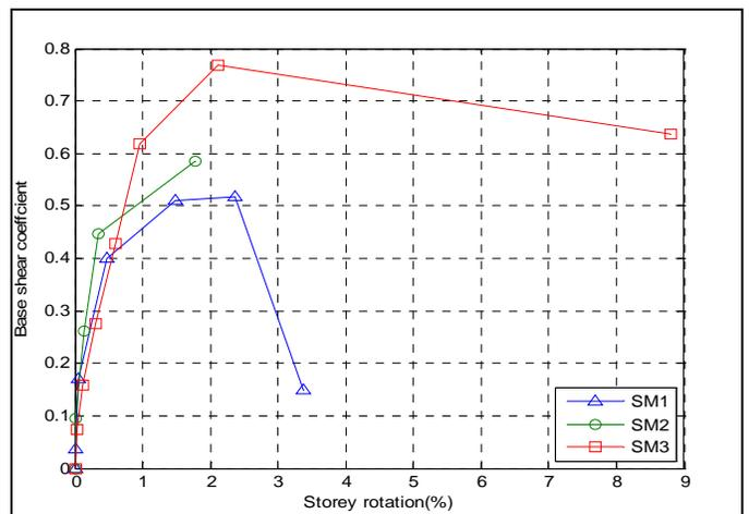
Figure 9: Seismic response envelop curves for models SM1, SM2 and SM3
