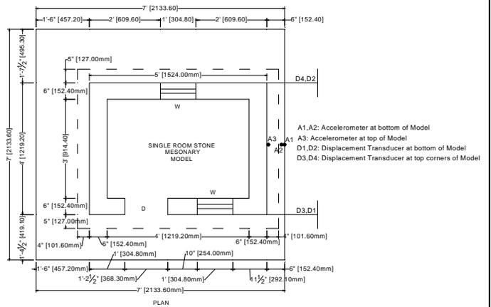
Figure 3 : Reduced scale model SM1 and its instrumentation detail for shake table test
