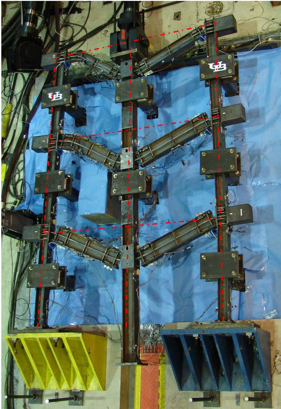
Figure 4. Photograph of the damaged state of the PTED specimen after the end of testing; approximate locations of the un-deformed members' centerlines are marked in red; the current viewpoint is from an oblique angle and has some distortion due to perspective.
