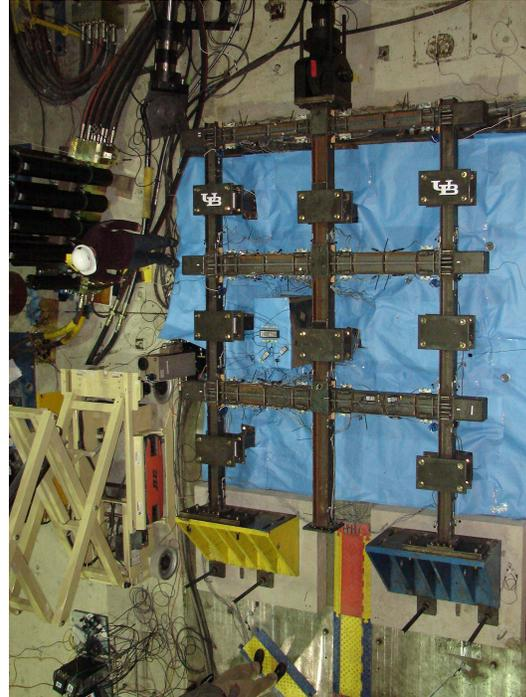
Figure 1. Geometry, loading method and basic features of the PTED specimen (left); general view of the experimental setup on the strong floor of SEESL before the testing (right).
