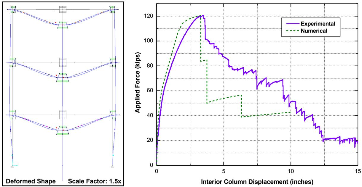
Figure 5. Deformed view of numerical model of the PTED frame (left) and comparison of experimental and numerical global force vs. interior column displacement plots (right).
