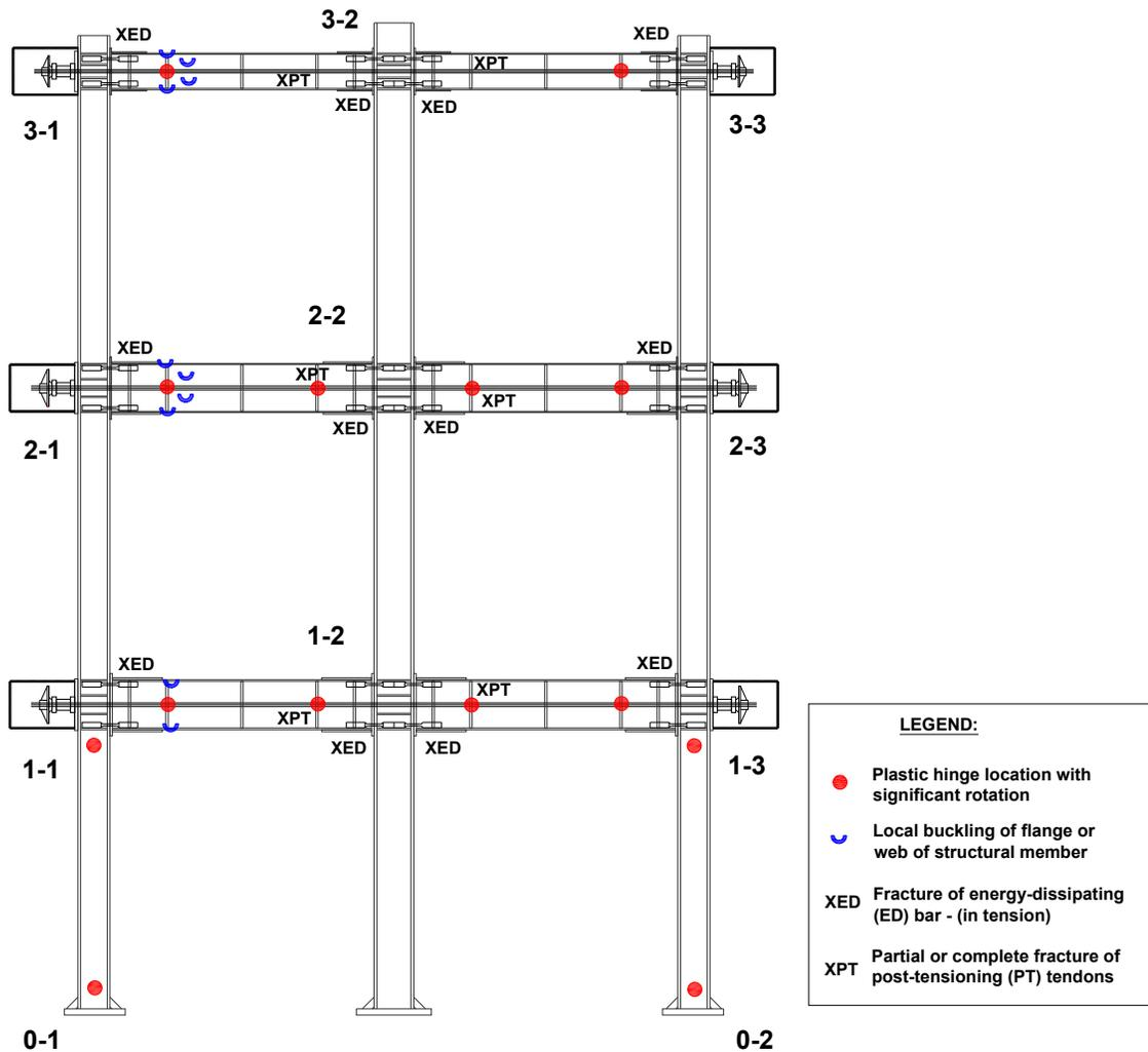
Figure 3. Schematic of the damaged state of the PTED specimen at the end of the collapse test with the spatial distribution of major types of damage (the frame is shown in the original un-deformed geometry for clarity); heavy buckling is observed at the unreinforced beam sections at the north side (left) of the 2<sup>nd</sup> and 3<sup>rd</sup> floor beams; tendon failures are random with tendency to occur near the interior beam column connections; ED-bars break in tension.
