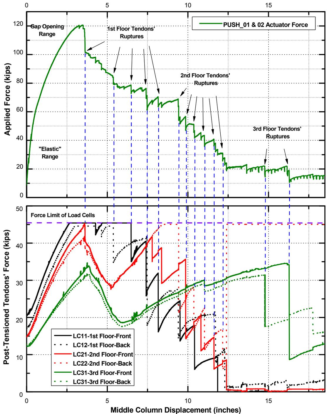
Figure 2. Combined plot of the global force vs. interior column E-W displacement response of the PTED specimen (top) and measured post-tensioning force vs. interior column E-W displacement for all six tendons of the PTED (bottom) correlating the global degradation behavior with single rupture events in the Mono-Strand wire bundles.
