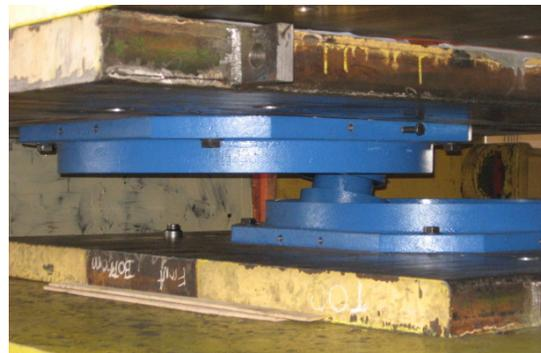
Figure 2. Fully displaced isolator
