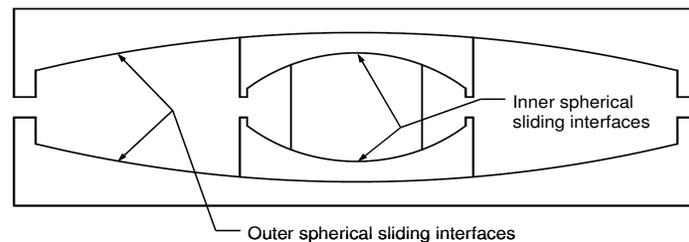
Figure 4: Section through typical Triple Pendulum bearing
