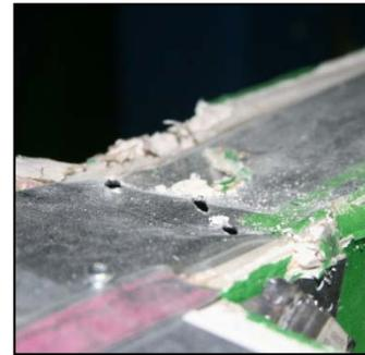
(s) Deformation of top track around brace connection
