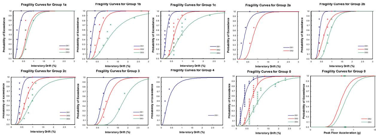
Figure 9. Example fragility curves for partition walls
