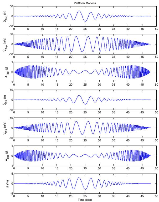
Figure 2. Dynamic fragility testing protocol
