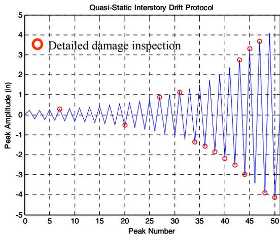
Figure 3. Quasi-static fragility testing protocol
