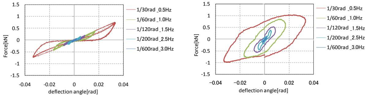
Figure 6. Load-deflection relations of the open frames (left: without dampers, right: with the dampers)
