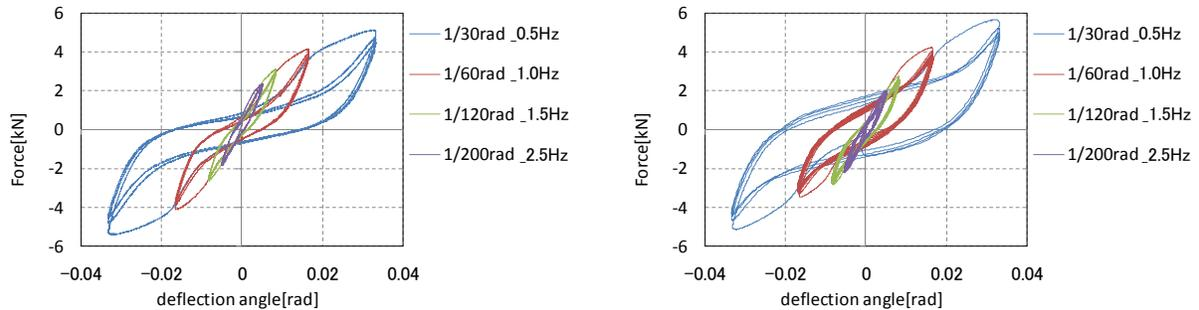
Figure 7. Load-deflection relations of the walled frames (left: without dampers, right: with the dampers)
