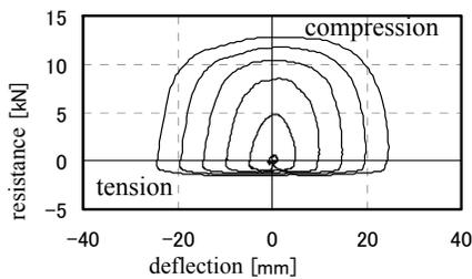
Figure 2. Load-deflection relation of compressive oil damper (1.0Hz)
