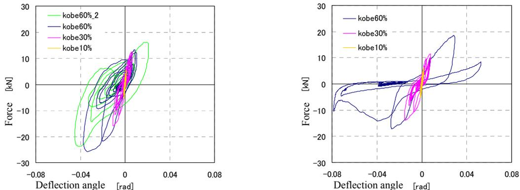
Figure 10. Load-deflection relations for test frames (left: with dampers, right: without dampers)
