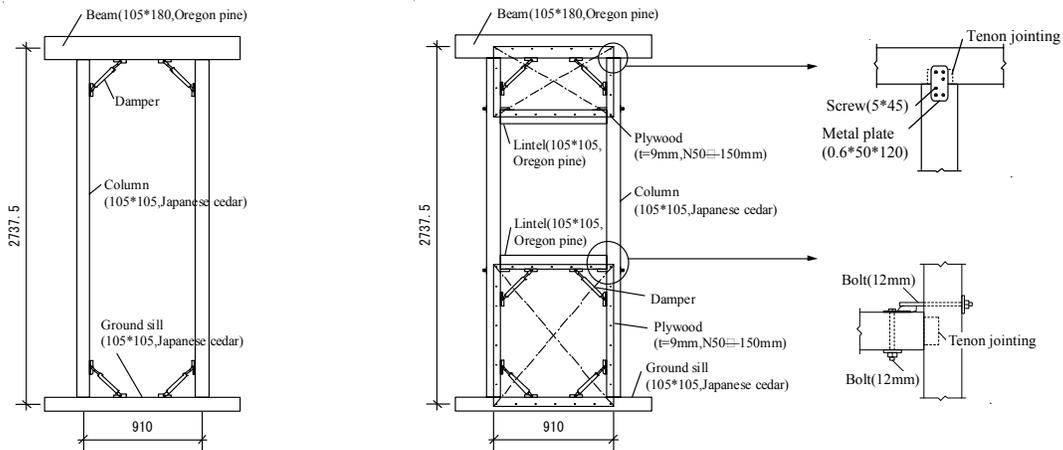
Figure 5. The dimensions of test frames (left: open frame, right: walled frame)
