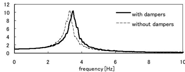
Figure 9. Transfer functions of test frames with/without dampers
