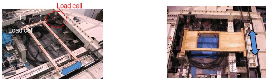
Photograph 2. Dynamic loading test system (left: open frame, right: walled frame)
