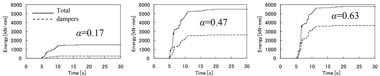
Figure 11. Ratio of absorbed energy in damper to total input energy (left: JMA Kobe 30%, center: JMA Kobe 60%, right: JMA Kobe 60%\_2nd)
