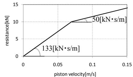
Figure 3. Damping coefficients of the damper
