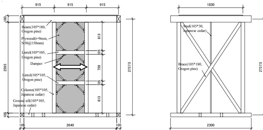
Figure 8. Elevations of the test frame with dampers
