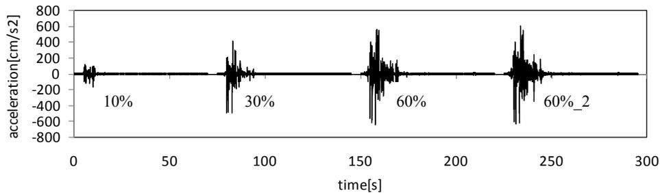
Figure 13. A series of accelerations recorded on the shake table
