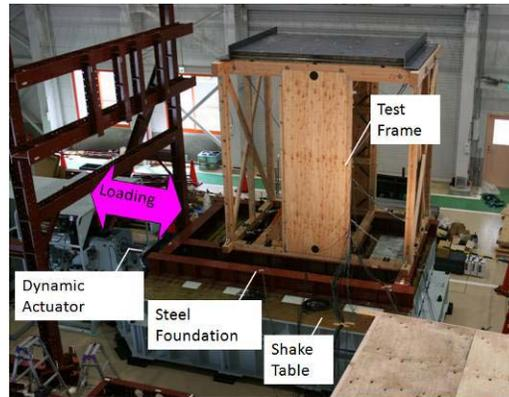
Photograph 3. Shake table test system
