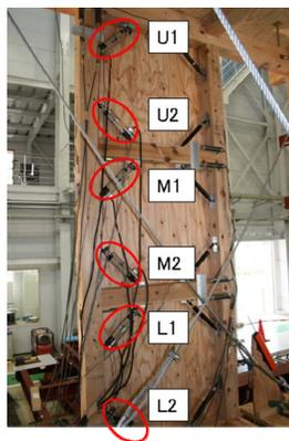
Photograph 4. Arrangement of dampers and deflection gauges
