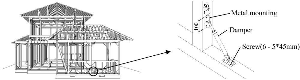
Figure 4. Installment of the damper into wooden house
