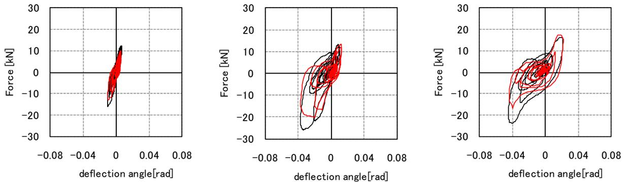
Figure 14. Comparison between experimental results and analytical results (left: JMA Kobe 30%, center: JMA Kobe 60%, right: JMA Kobe 60%\_2nd)
