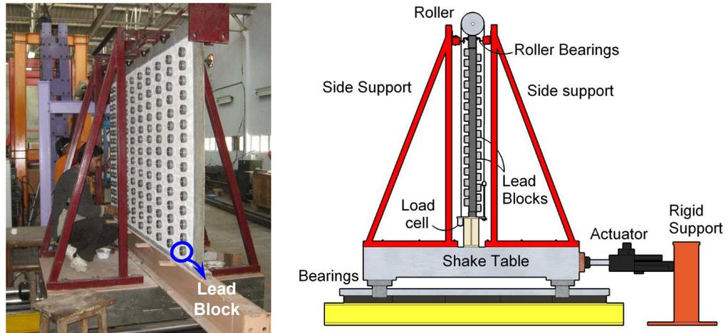
Figure 1. Test setup for shake table test of masonry panel
