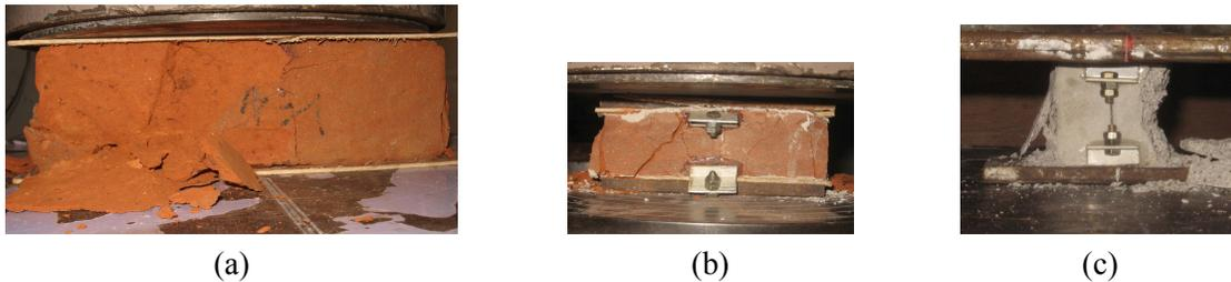
Figure 3. Typical failure modes: (a) prototype brick (b) model brick and (c) mortar cube
