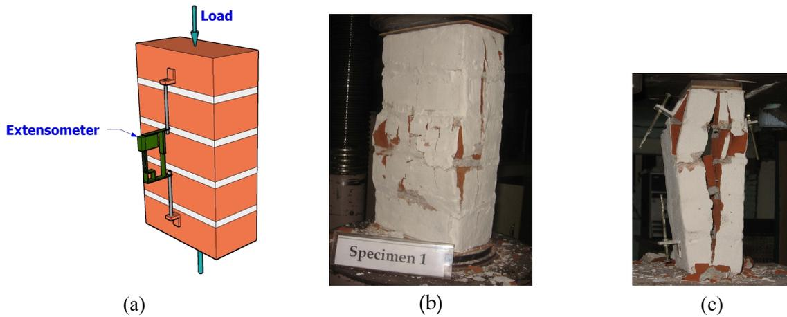
Figure 4. Compression testing and typical failure mode of prototype and model masonry prism.
