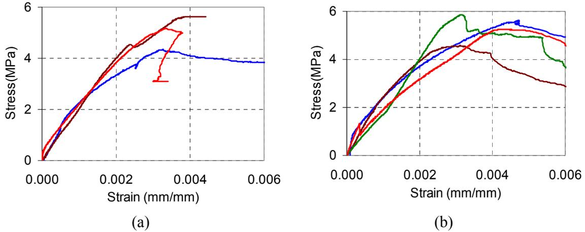
Figure 5. Typical compressive stress-strain curves for (a) full-scaled and (b) half-scaled prism
