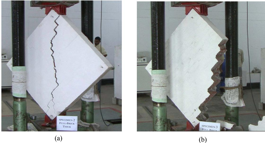
Figure 7. (a) Typical diagonal tension of different specimens (b) 'odd' failure of full-brick thick prototype specimen
