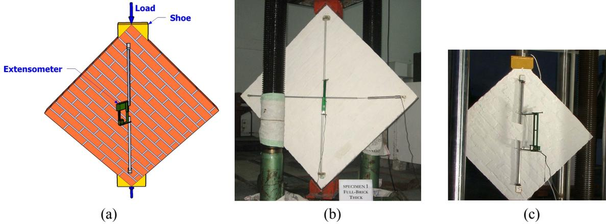
Figure 6. Test setup for diagonal compression test of half-scaled and full-scaled masonry
