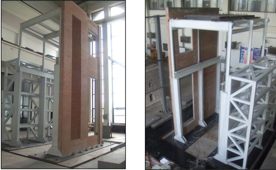
Figure 6. Model of the wall ready for shake-table testing.
