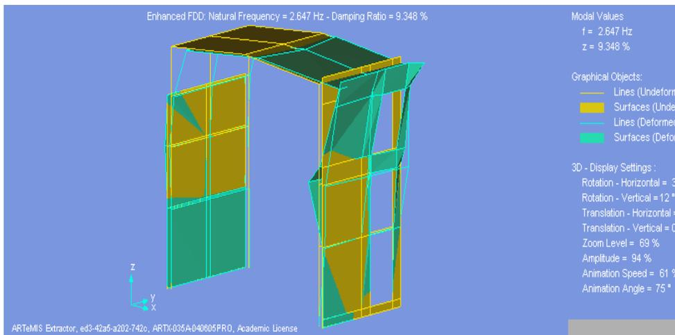
Figure 5. Mode 1 Vibration shape for frequency  $f_1=2.15$  Hz.
