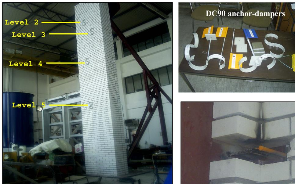
Figure 9. Position of DC90 anchors with dampers and measured levels.
