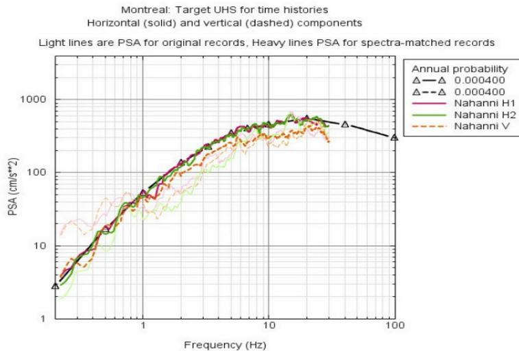
Figure 8. PSA for Nahanni M6.8 earthquake (After Atkinson, 2006).
