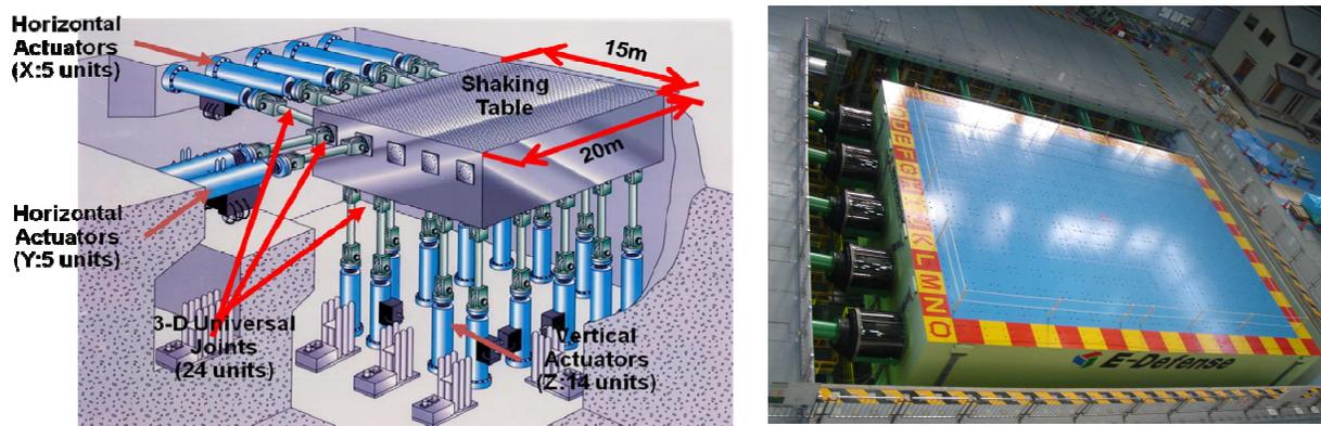
Figure 1. Illustration and photo of the E-Defense shaking table.
