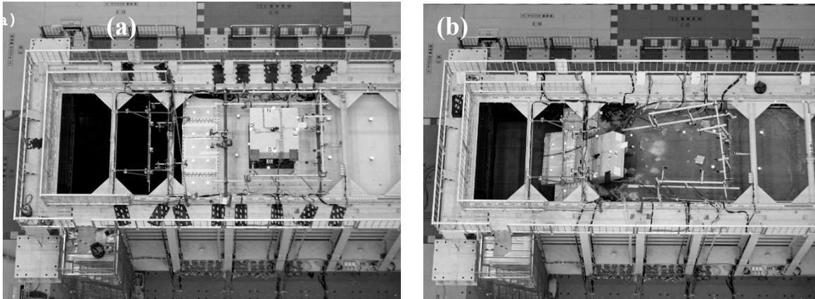
Photo 2. Caisson, pile-supported structure and their surroundings (a) before shaking and (b) after test completion.
