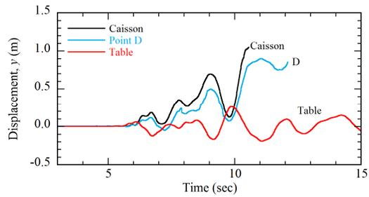
Figure 8. Horizontal displacements of the caisson, point D and shaking table.
