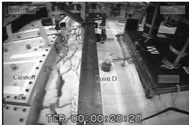
Photo 3. Close view of the caisson, backfill surface and footing during shaking.
