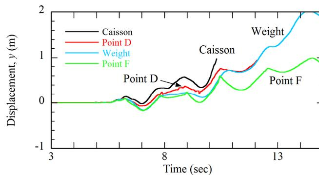
Figure 10. Horizontal displacements of the caisson, weight, and points D and F.
