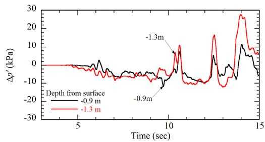
Figure 9. Effective earth pressure changes on the backfill side of the caisson.
