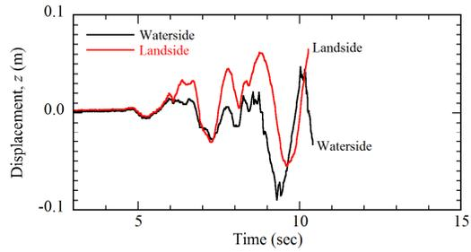
Figure 7. Vertical displacements determined at the waterside and landside tops of the caisson.
