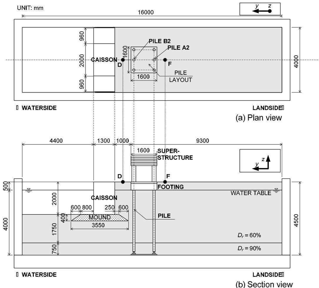
Figure 2. Illustrations of the specimen and the locations of the measurement points D and F : (a) Plan and (b) section views.
