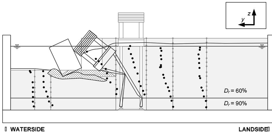
Figure 5. Section of the change of the specimen due to shaking. Gray and black colors indicate the structures and measurement points before and after the test respectively.
