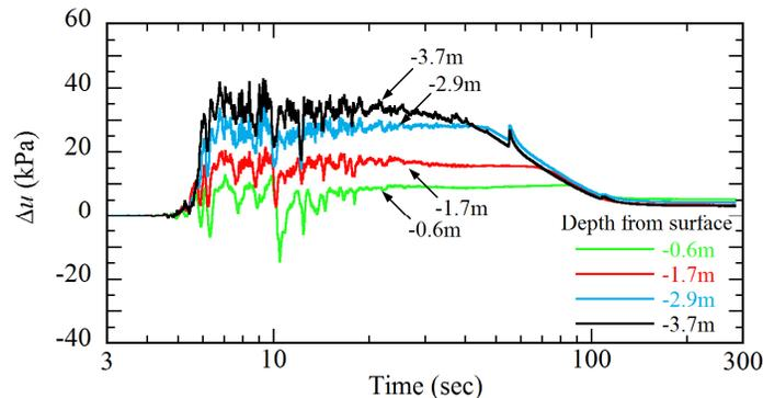
Figure 6. Excess pore water pressure changes at different levels under the point F.
