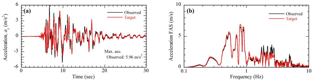
Figure 4. Comparison between the target input motion signaled to the table and actual, observed table motion: (a) Acceleration time histories and (b) acceleration Fourier amplitude spectra.
