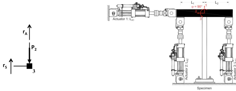
Figure 3. Forces summed up at interface Node 3 at  $n + 1$  (left) and three actuator experimental setup (right).
