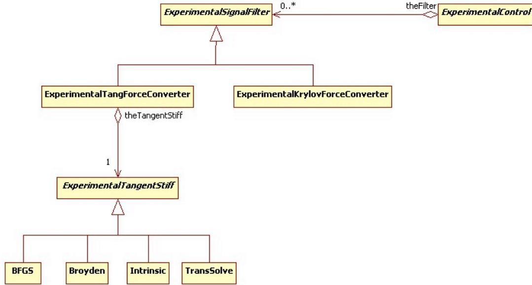
Figure 1. New proposed software architecture for OpenFresco for force control.
