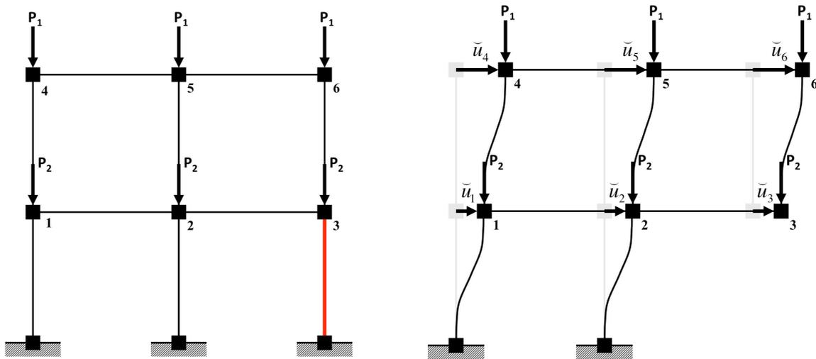
Figure 2. Mixed control example model (left) and deformed model (right) at  $n + 1$ .
