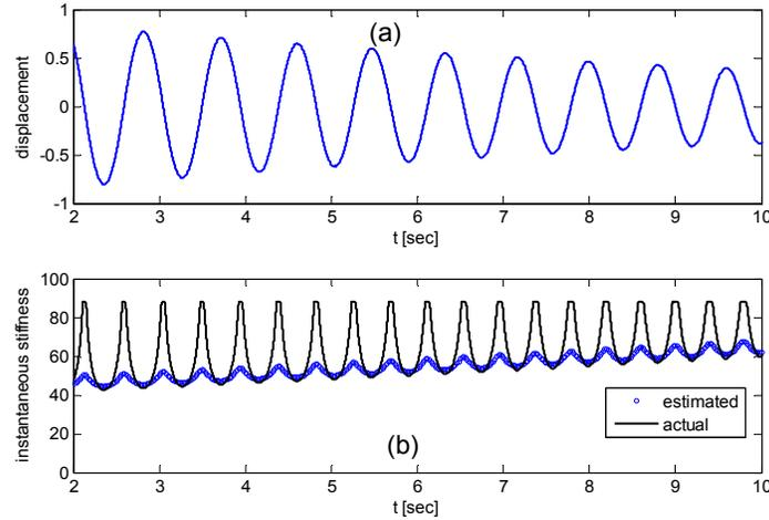
Figure 3. Instantaneous stiffness. (a) Free vibration response. (b) Estimated and actual secant stiffness.
