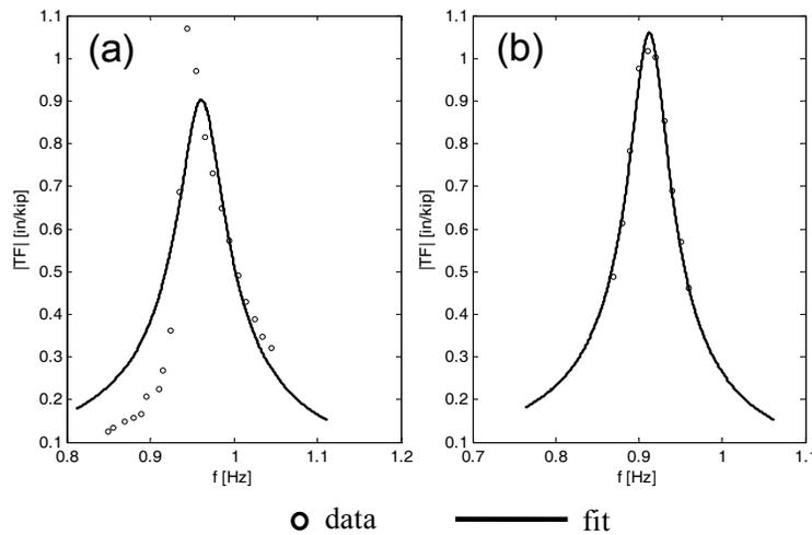
Figure 6. Transfer functions in the full-scale structure. (a) non-constant-displacement-response TF. (b) constant-displacement-response TF.
