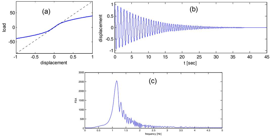
Figure 1. Frequency estimate from free vibration of a nonlinear elastic system. (a) Load-displacement curve. (b) free-displacement response. (c) Fourier spectrum.
