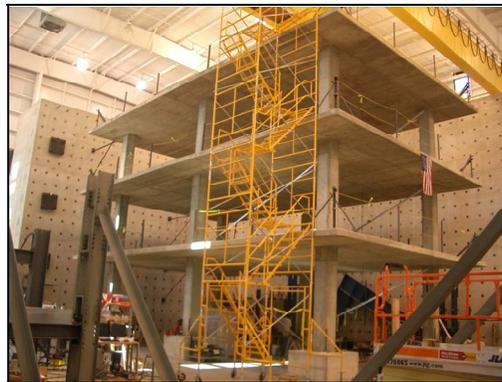
Figure 5. Full-scale three-story reinforced concrete flat-plate building at the Bowen Laboratory of Purdue University.
