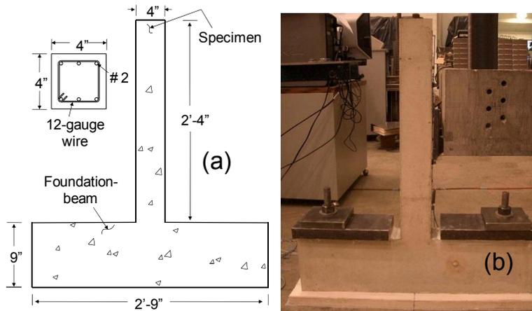
Figure 7. Small-scale cantilever beam. (a) Reinforcing details. (b) General view.
