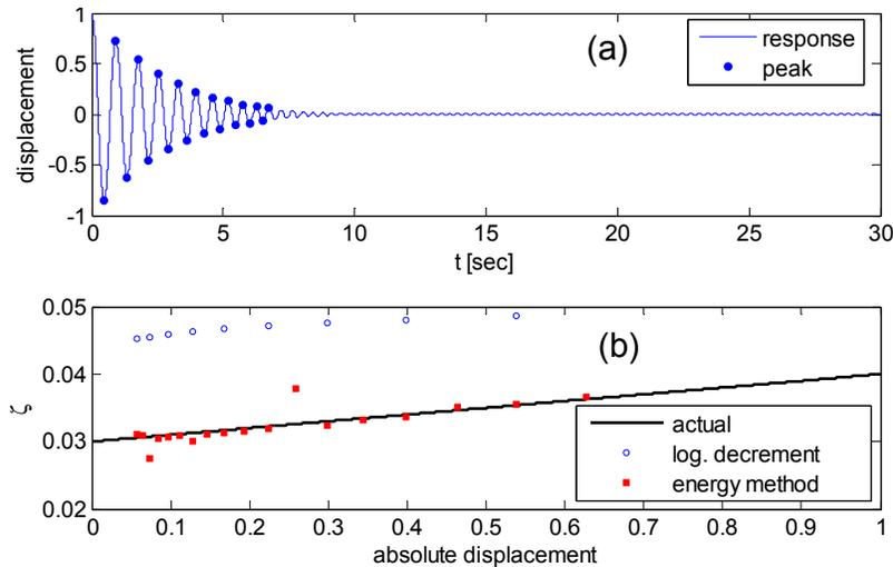
Figure 4. Amplitude-damping obtained estimated through the Energy Method. (a) Free vibration response. (b) Comparison of  $\zeta$  values.
