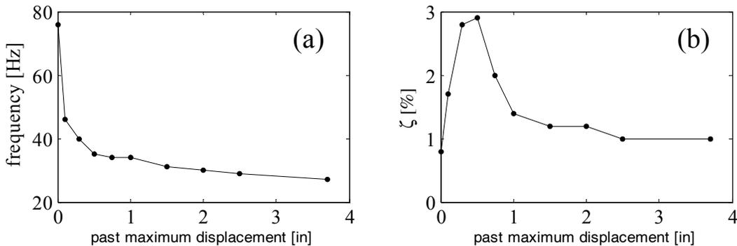
Figure 8. Variation of dynamic properties with the past maximum displacement in a small-scale beam. (a) Frequency. (b) Viscous damping ratio.
