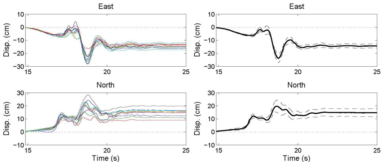
Figure 5. Left: The individual displacement time histories at ICEARRAY stations along the East and North directions at top and bottom, respectively, according to the correction method applied. Right: The mean displacement (right) and its corresponding  $\pm\sigma$ .
