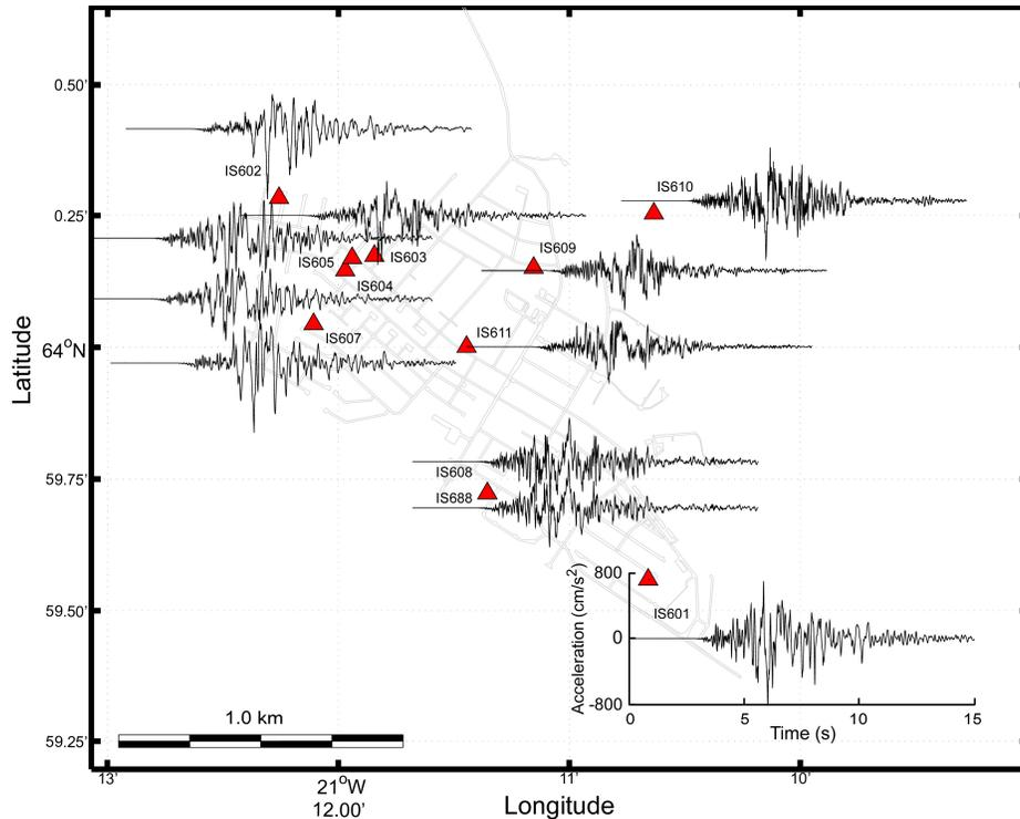
Figure 2. Segments of the east-west (SN) component of recorded acceleration time histories on the ICEARRAY stations during the Ölfus earthquake. The triangles denote the station locations (stations IS608/688 are collocated) and the gray lines show the street layout of Hveragerdi.
