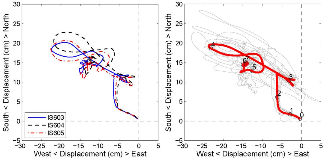
Figure 7. Coseismic particle displacement on stations IS603-5 (left) and on all stations (right, gray lines) along with the average displacement (red, numbers are seconds).
