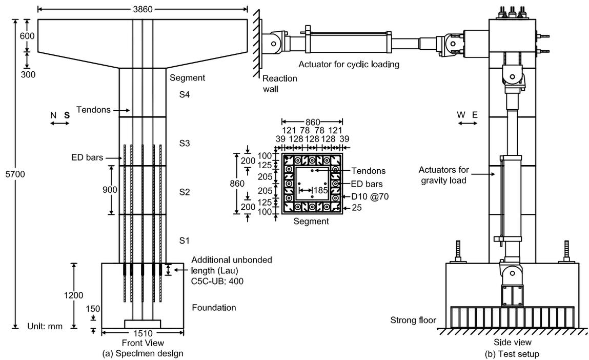
Figure 1. Specimen design and test setup
