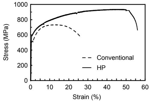
Figure 2. Monotonic tension behavior of conventional and HP ED bars
