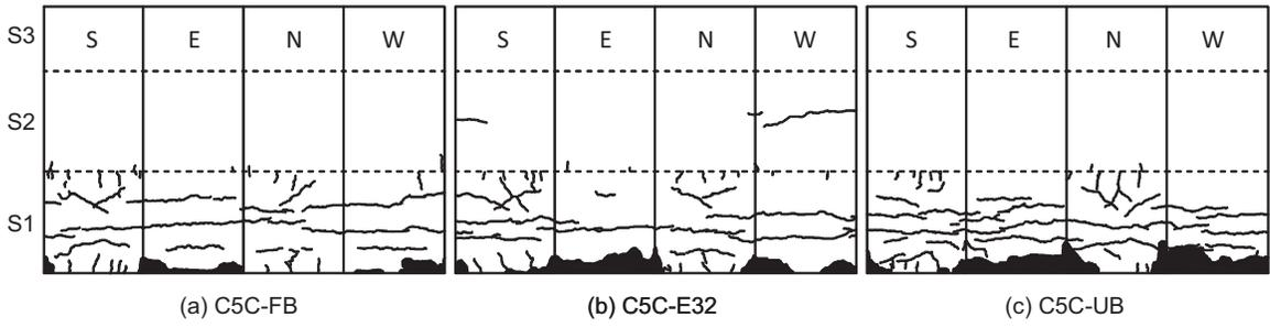
Figure 4. Cracks and spalling of concrete
