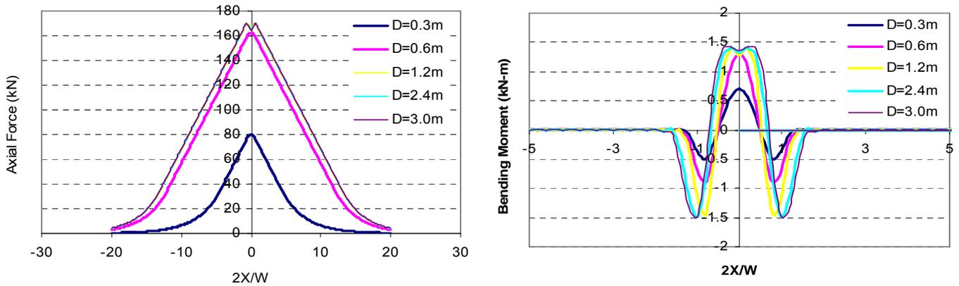
Figure 7. Axial force and bending moment development in the buried cable at different ground deformation levels
