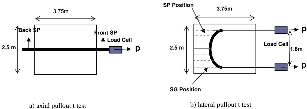
Figure 1 . Schematic diagram showing typical test set up: a) axial pullout test, b) lateral pullout test (SP=String Potentiometer, SG=Strain Gauge)
