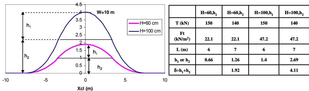
Figure 11. Verification of the proposed formula to predict the maximum cable deformation ( $D_{pl}$ )
