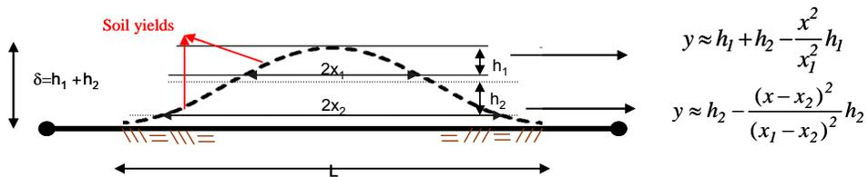
Figure 10. Analytical formula representation of the plateau deformation
