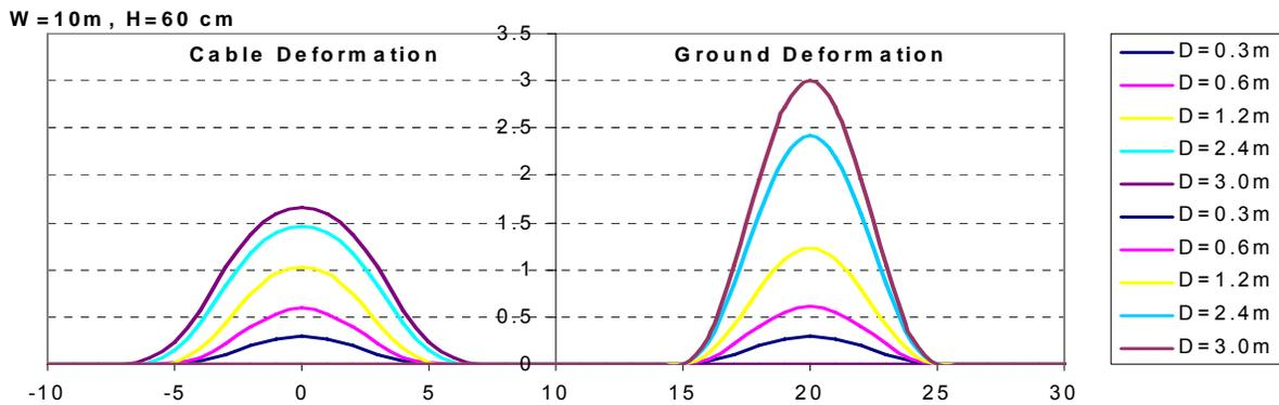
Figure 6. Ground deformation and corresponding cable deformation subjected to the transverse PGD with the width of 10 m ( $W=10m$ )
