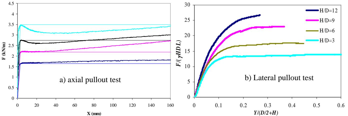
Figure 3. a) load-deformation curves and bilinear representations of the longitudinal soil spring for the buried cable in the axial pullout test and b) load-deformation curves for the buried cable in the lateral pullout tests.
