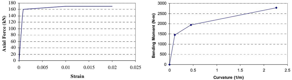
Figure 2: The mechanical properties of the buried power transmission cables, axial-strain behaviour (left), moment-curvature behaviour (right)
