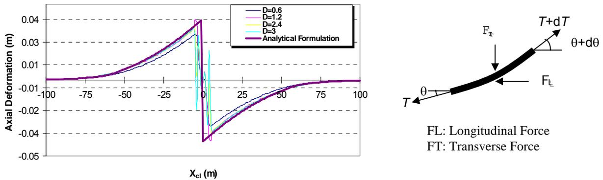
Figure 8. Verification of the proposed formula to predict the axial deformation development in the buried cable (left), and the forces acted on the small portion of the cable(right)
