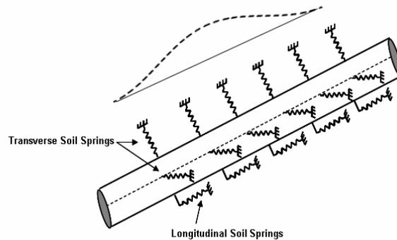
Figure 4. The idealized soil/cable interaction representation at the buried cable interface
