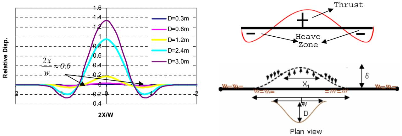
Figure 9. The relative deformation of the ground and the buried cables and the formation of the “thrust” and “heave”
