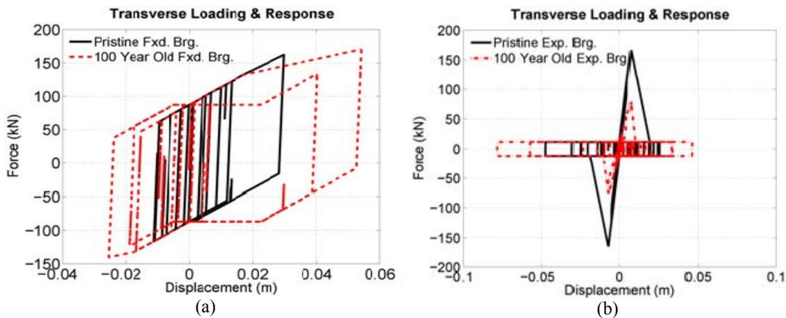
Figure 3 Transverse loading and response of a) corroded fixed bearings and b) corroded expansion bearings along the service life of the bridge.
