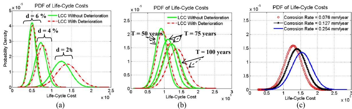
Figure 5 Sensitivity of seismic LCC estimation with a) different discount ratios ( $T=100$  years), b) different service lives of the deteriorating bridge ( $d=2\%$ ) and c) different corrosion rates ( $d=2\%$ ,  $T=100$  years)
