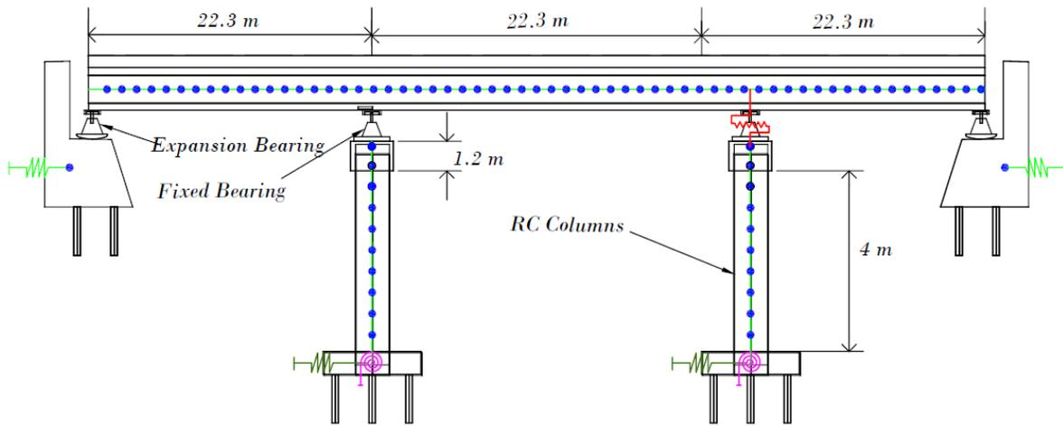
Figure 1 Case study MSC steel bridge showing components under deterioration consideration
