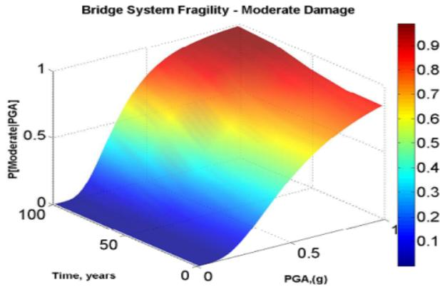
Figure 4 Deteriorating bridge fragility surface for moderate damage state.
