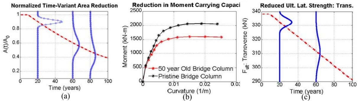
Figure 2 a) Area reduction of reinforcing steel in concrete columns b) reduced moment resisting capacity of corroded column and c) reduction in the ultimate lateral strength of fixed bearings in the transverse direction.
