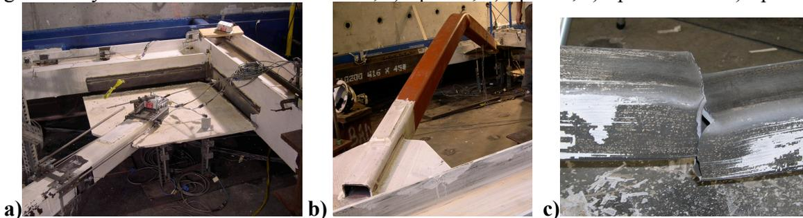
Figure 7. Photographs; a) Weld fracture, b) Out-of-plane buckling, c) Brace fracture
