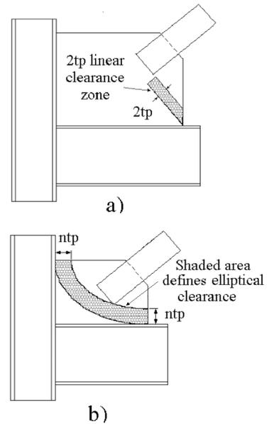
Figure 2. Gusset clearance models
