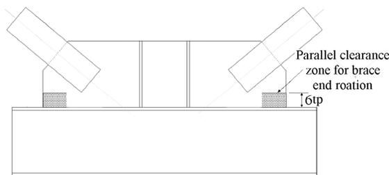
Figure 8. Parallel  $6t_p$  clearance model for midspan gusset
