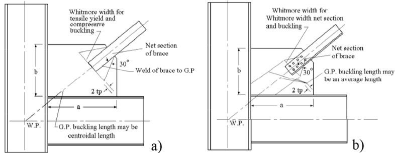
Figure 3. Typical GP design checks; a) Welded tube brace, b) Bolted angle brace
