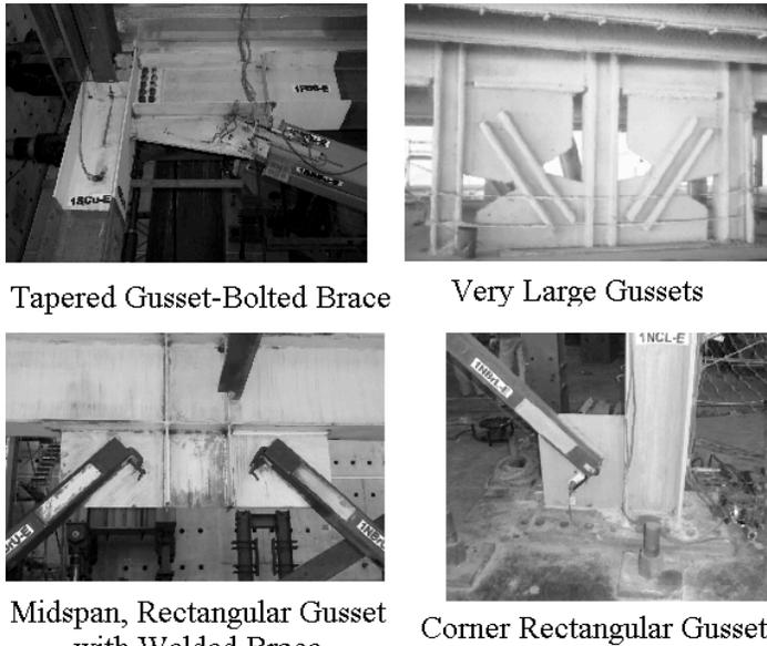
Figure 1. Typical CBF GP connections
