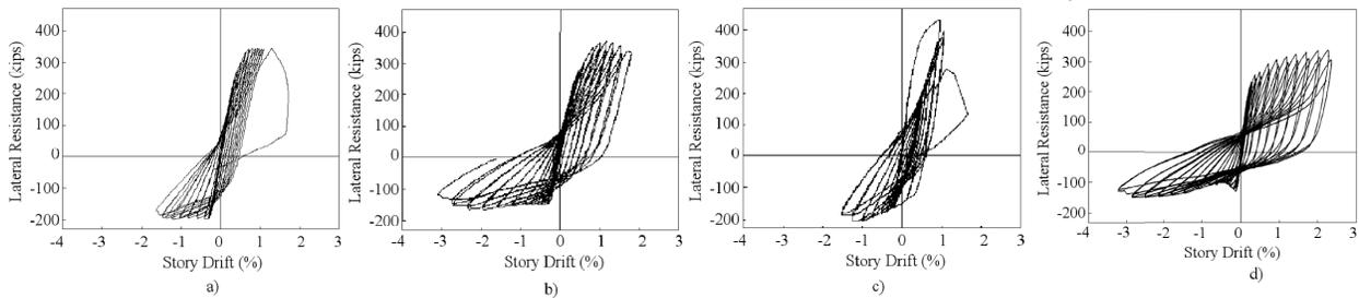
Figure 6. Cyclic force-deflection behaviors; a) Spec. 1, b) Spec. 5, c) Spec. 11 and d) Spec. 23
