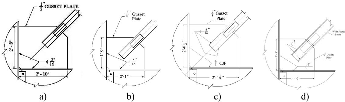
Figure 5. GP design; a) Specimen 1, b) Specimen 5, c) Specimen 11, d) Specimen 23
