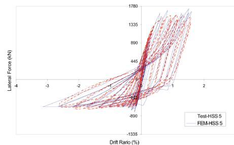
Figure 9. Comparison of measured and computed force-deflection behavior
