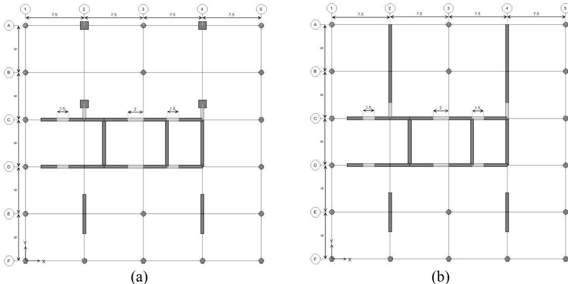
Figure 2. (a) Ground floor and (b) typical floor plan of the building
