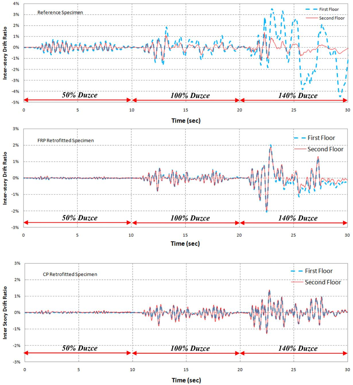
Figure 4. Drift Ratio Response of Test Specimens
