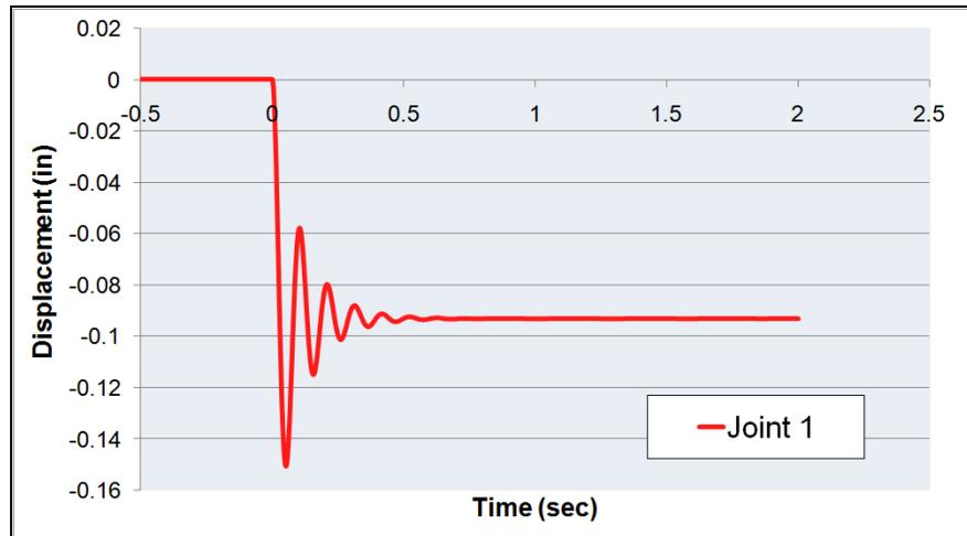
Figure 10 –Displacement above the First Removed Column (Joint 1) after First Column Removal
