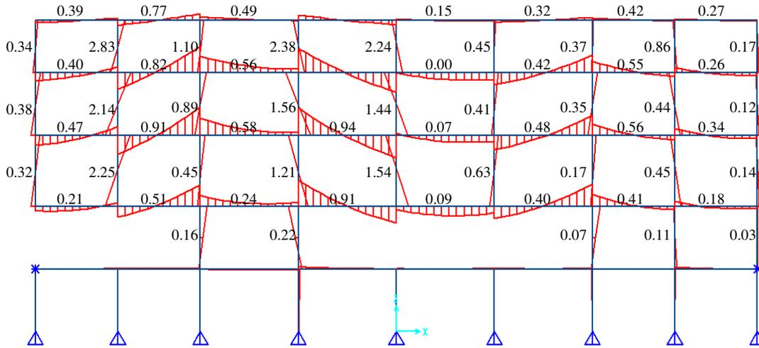
Figure 6 - DCR Values and Moment Diagram after Loss of Four Columns
