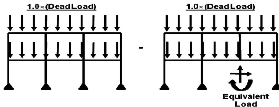
Figure 8 – Column Removal Load Representation for Nonlinear Dynamic Analysis
