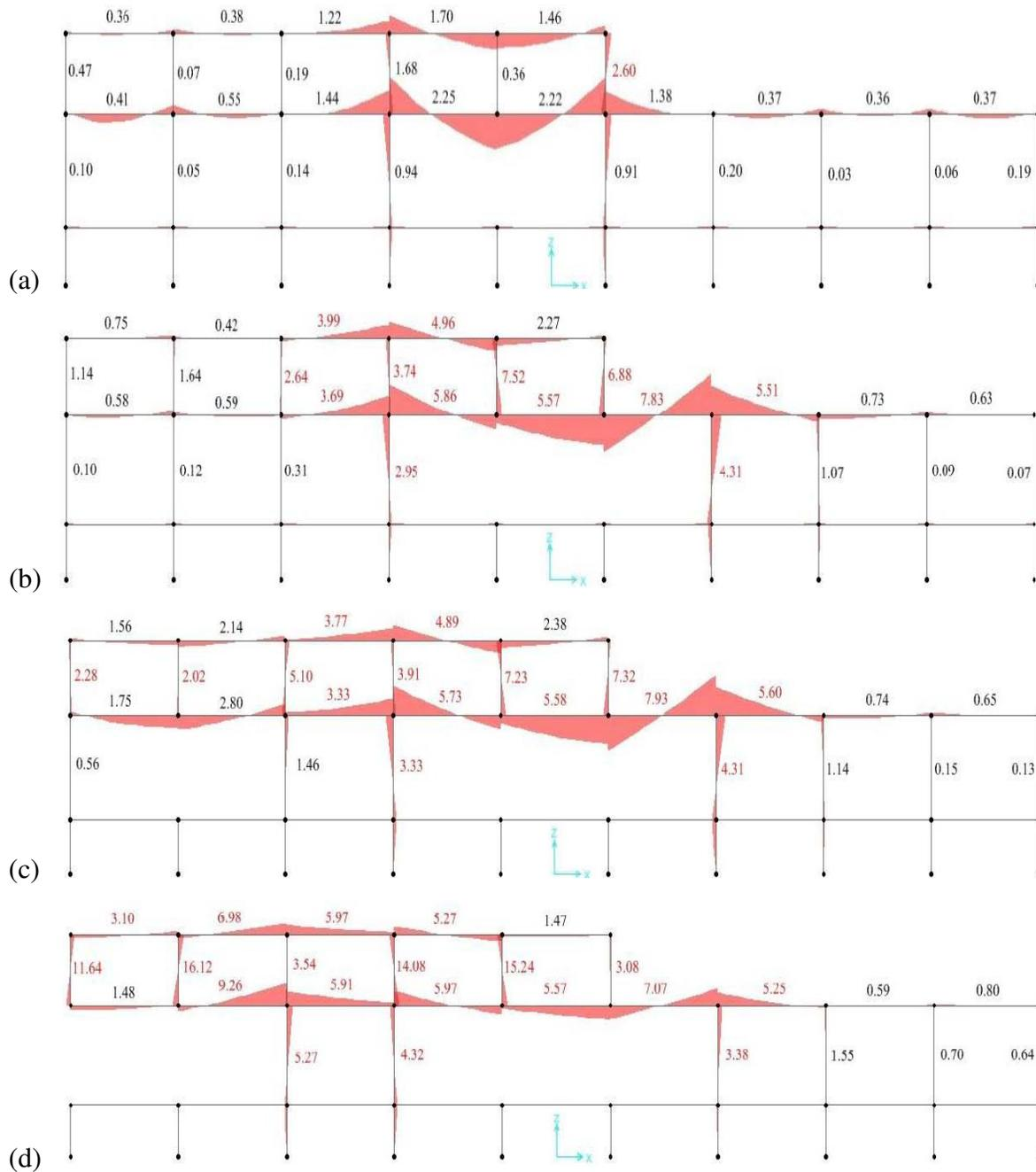
Figure 12 - Calculated Bending Moment Diagrams and DCR Values after the Removal of: (a) First Column, (b) Second Column, (c) Third Column, and (d) Fourth column
