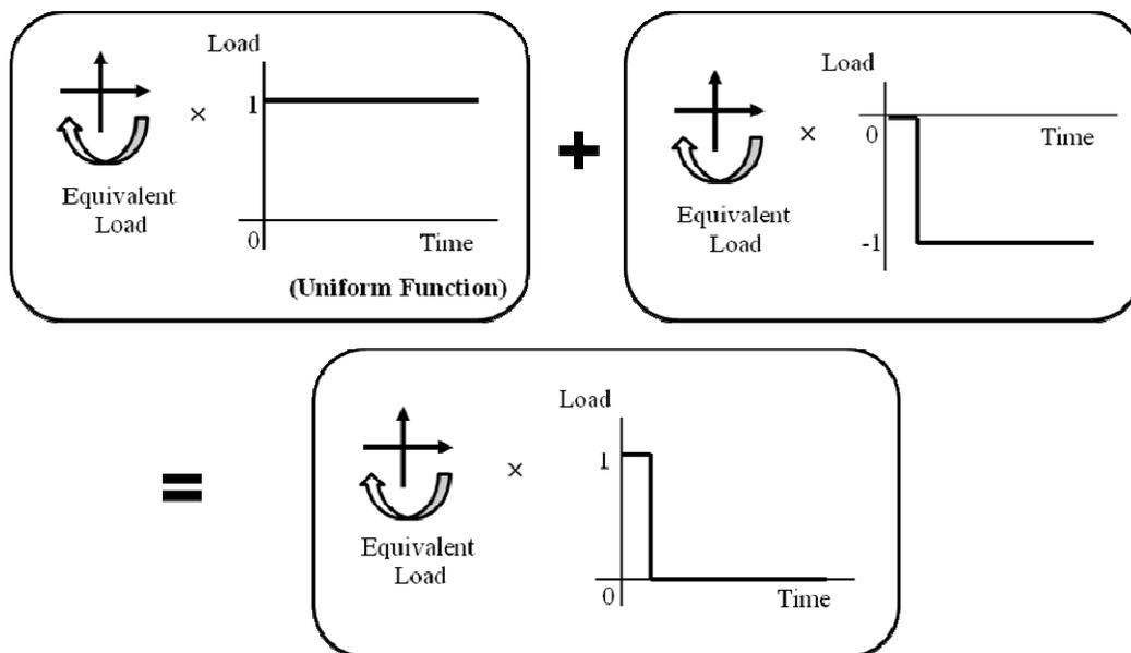
Figure 9 – Time History Function for Column Loss Simulation
