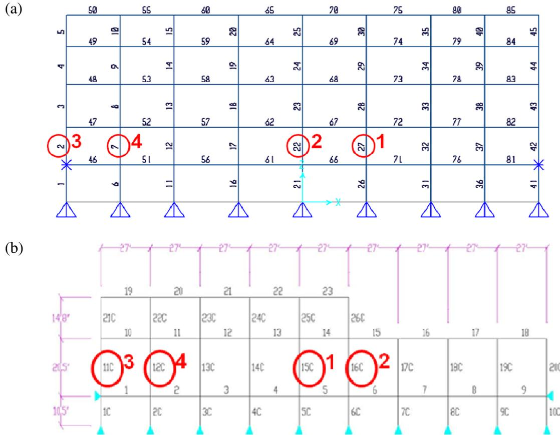
Figure 4 - Two-Dimensional Model for the Longitudinal Perimeter Frames of (a) Ohio Union Building and (b) BLCC Building (Circled Columns were Removed in the Order Shown)
