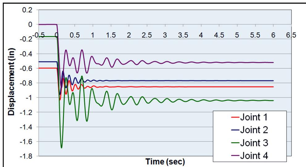
Figure 11 - Displacement of Joints above Each Removed Column after Removal of All Columns
