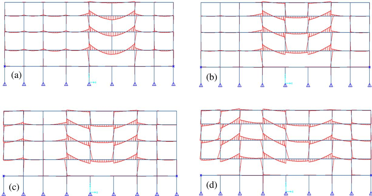
Figure 5 – Elastic Moment Diagrams After the Removal of: (a) One Column, (b) Two Columns, (c) Three Columns, and (d) Four Columns
