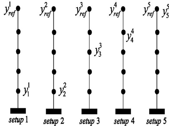
Figure 1 - Typical multi-setup test procedure
