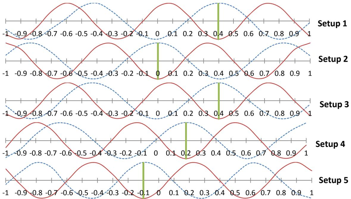
Figure 4. Phase Angle vs. Time Lag (PATL) plots for all setups, with solutions shown by vertical lines
