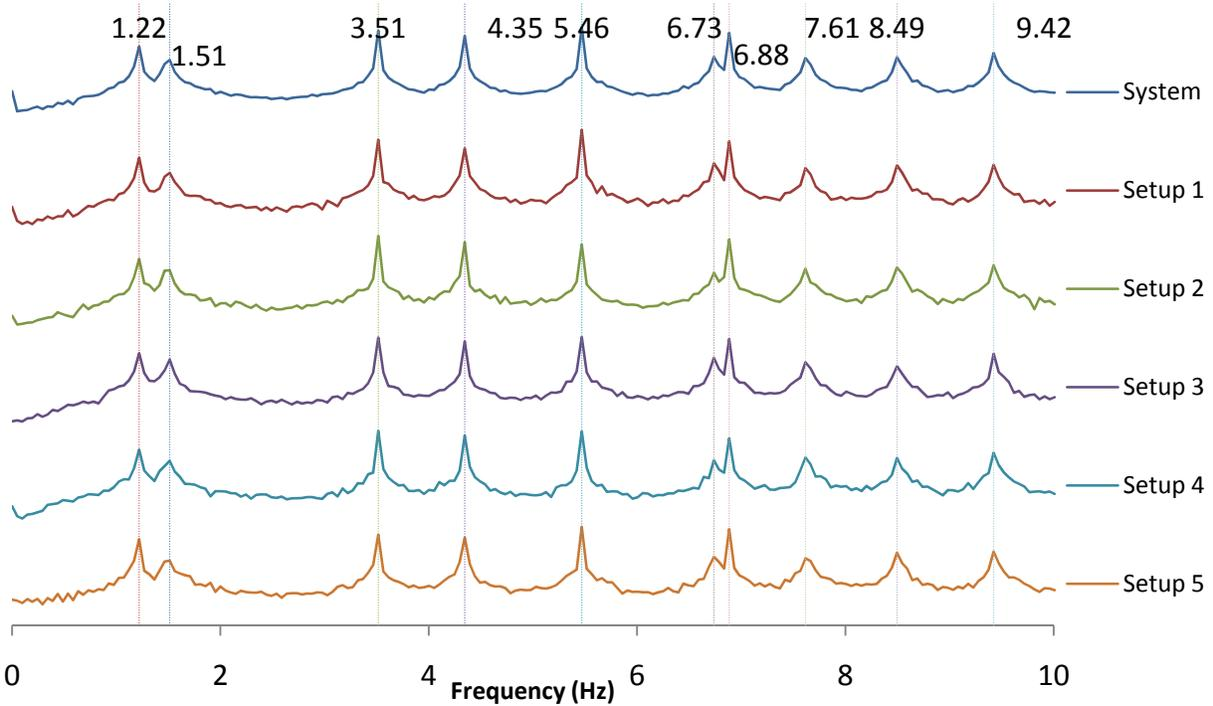
Figure 3. First singular values vs. frequency for the assembled system and for each setup – Un-synchronized data.
