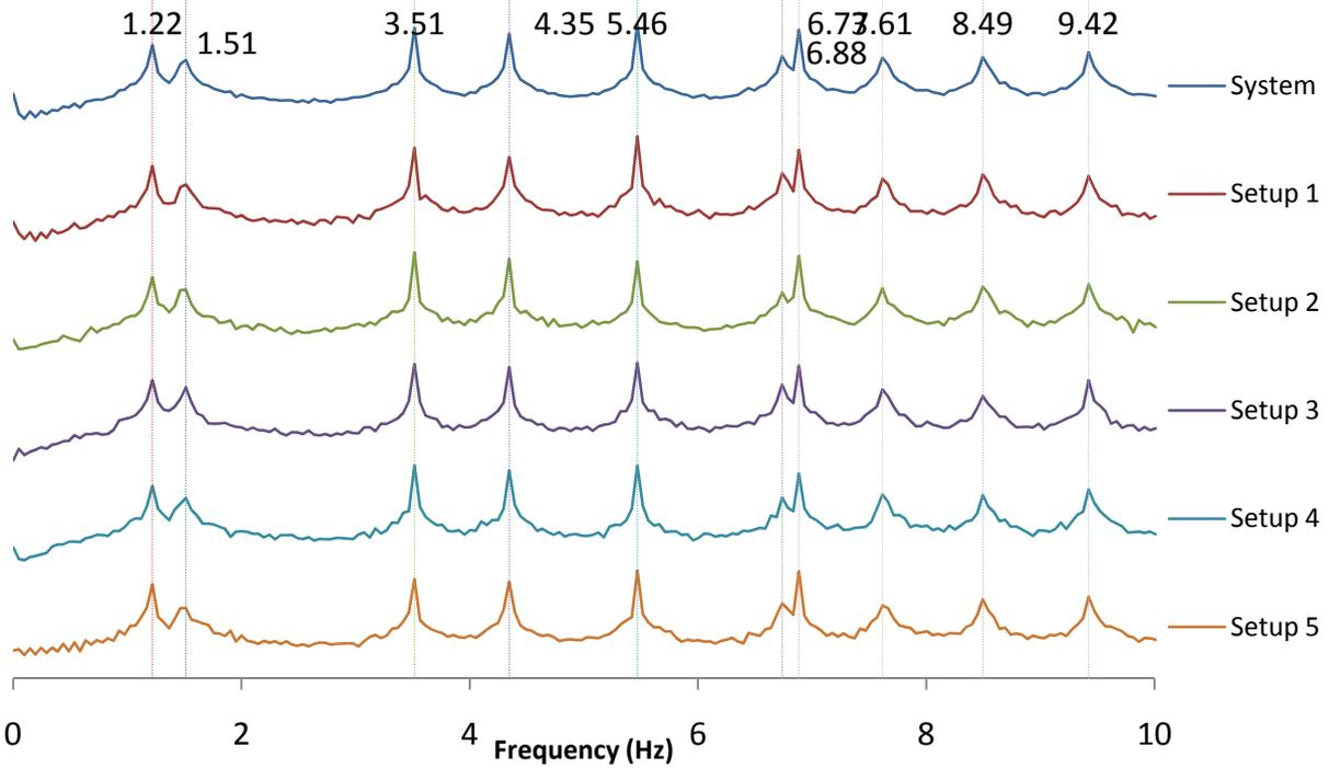
Figure 2. First singular values vs. frequency for the assembled system and for each setup, Synchronized Data
