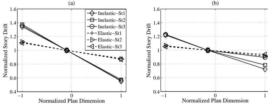
Figure 4: Median normalized story drift ratios for the 2/50 year event in (a) Y direction and (b) X direction
