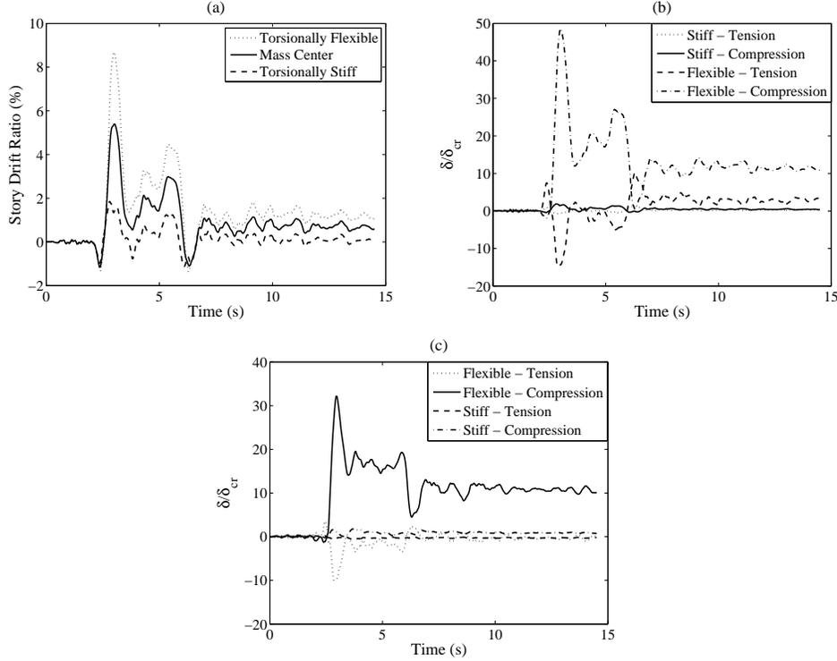
Figure 6: Time history of first story (a) Y-direction drift ratio (b) brace deformations in Y-direction, and (c) brace deformations in X-direction for the Elysian Park (SAC la35/la36) record. Compressive brace deformations are positive.
