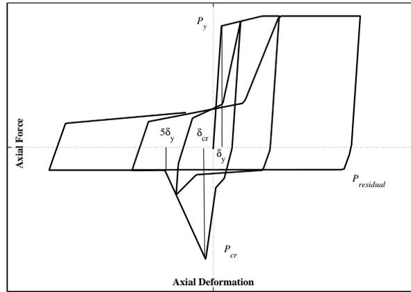
Figure 2: Cyclic constitutive force deformation relationship for axial behavior of braces
