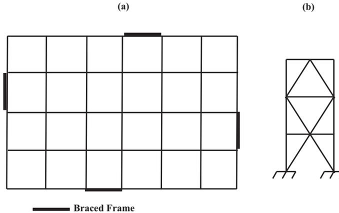
Figure 1: (a) Plan view of the building and (b) elevation view of a braced bay
