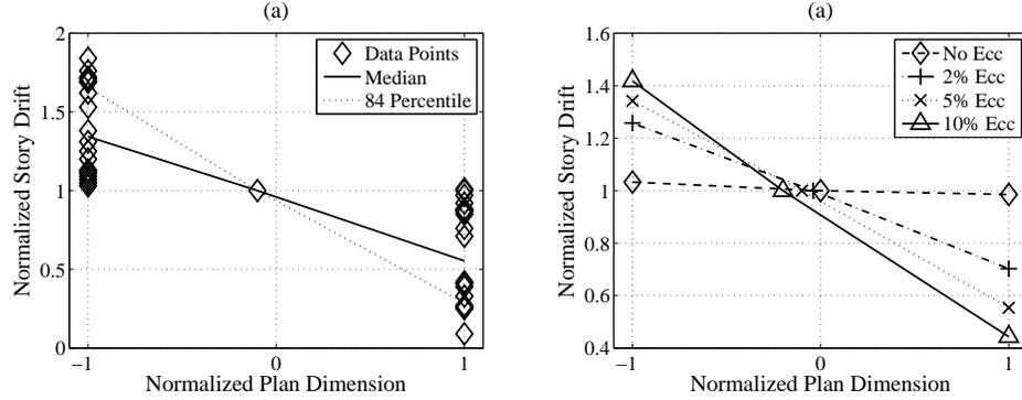
Figure 7: First story normalized story drift ratios for the 2/50 year event: (a) motion to motion to variation for 5% eccentricity (b) under various eccentricity levels
