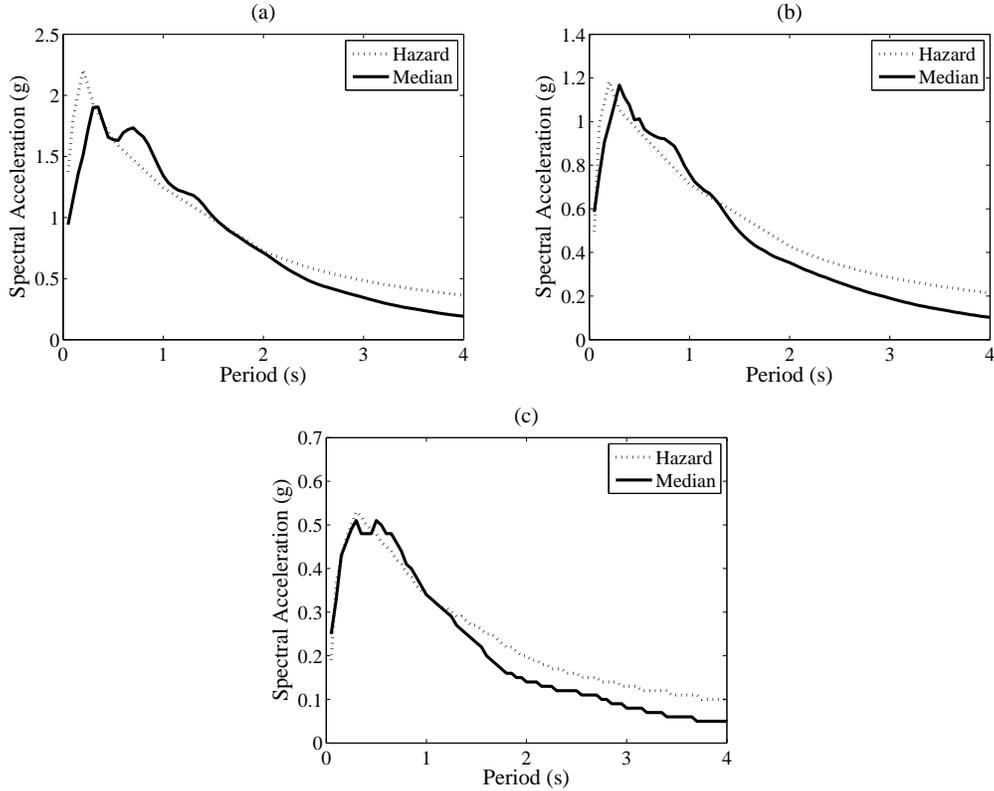
Figure 3: Target hazard spectrum and median of the response spectra of the scaled motions for (a) 2% PE in 50 years (b) 10% PE in 50 years and (c) 50% PE in 50 years hazard levels
