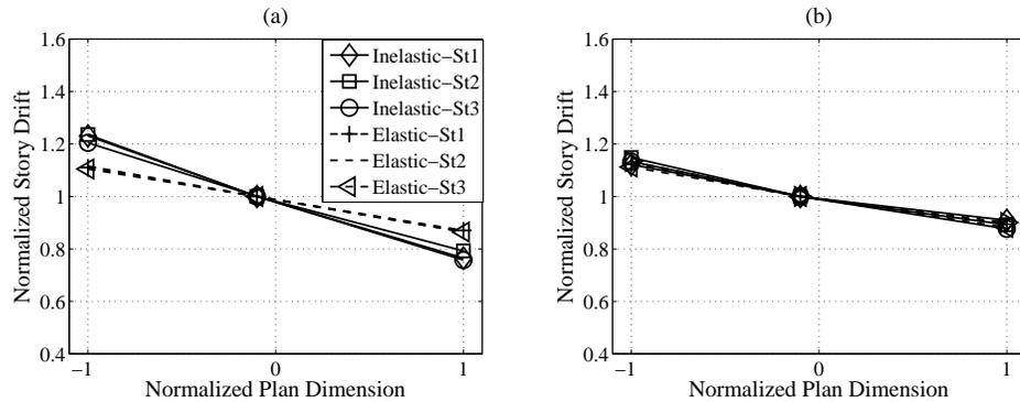
Figure 5: Median normalized story drift ratios for (a) 10/50 and (b) 50/50 year events in the Y direction
