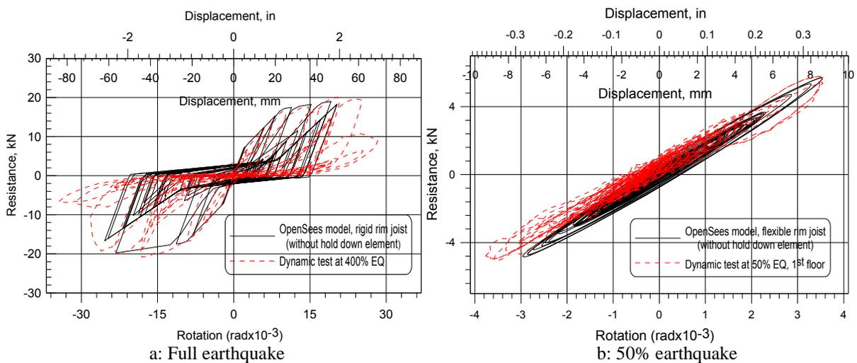
Figure 9. Shear resistance-deformation hysteresses: a) ST1-2 b) ST2-1 (1<sup>st</sup> floor)
