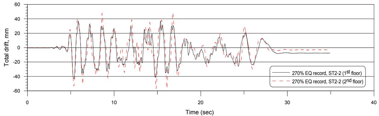
Figure 6. Comparison of total drifts of ST2-2 test specimen (270% EQ record).
