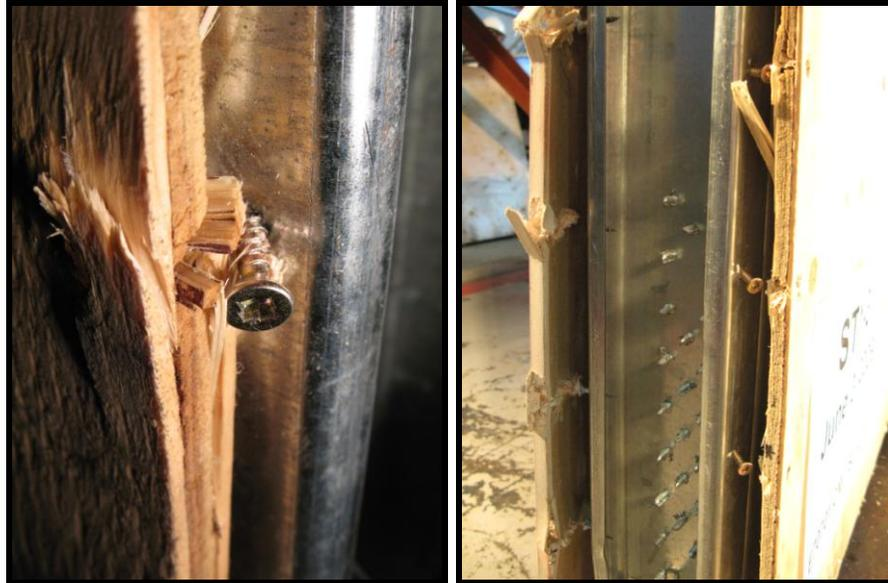
Figure 5. Typical connection based shear wall failure.
