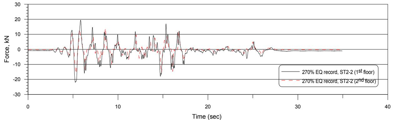
Figure 7. Comparison of inertia forces of ST2-2 test specimen (270% EQ record).
