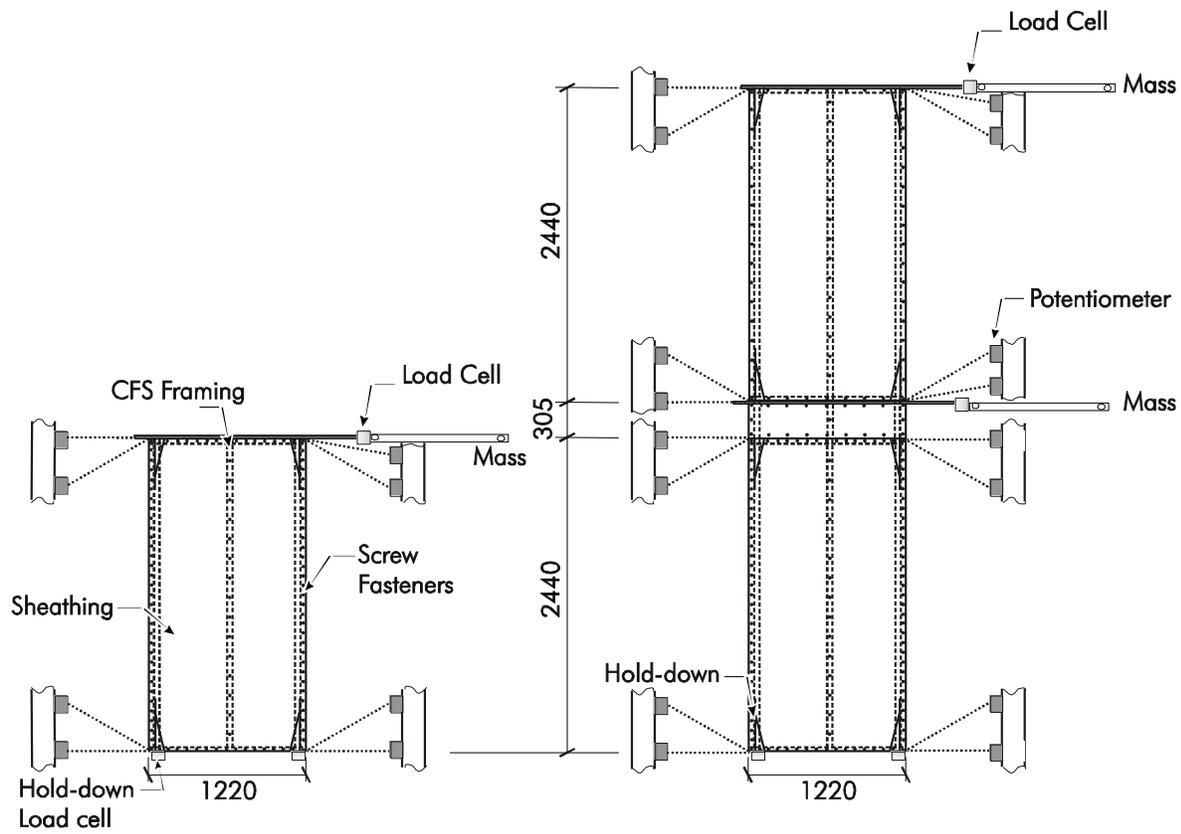
Figure 1. Single and double storey shear wall test specimens (mm).
