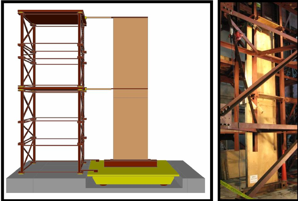
Figure 3. Two storey wood sheathed / CFS framed shear wall dynamic test assembly.
