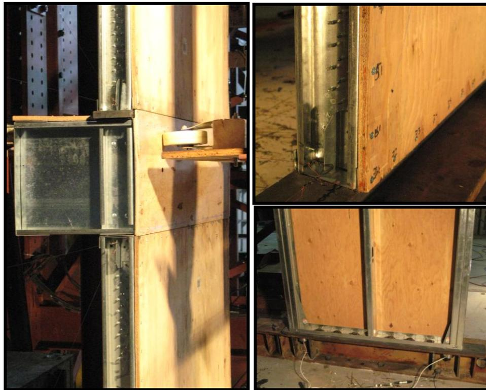
Figure 2. Typical details of shear wall construction.
