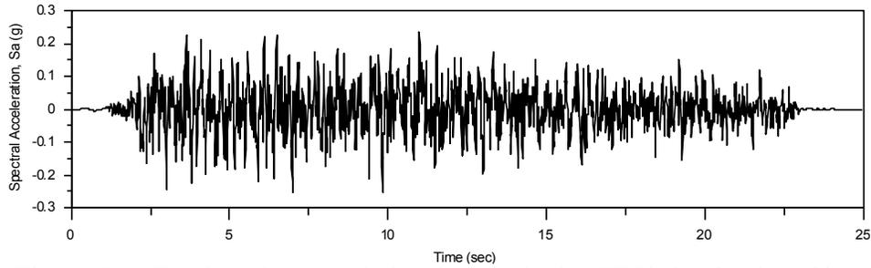
Figure 4. Earthquake record closely matched to UHS for Quebec City.
