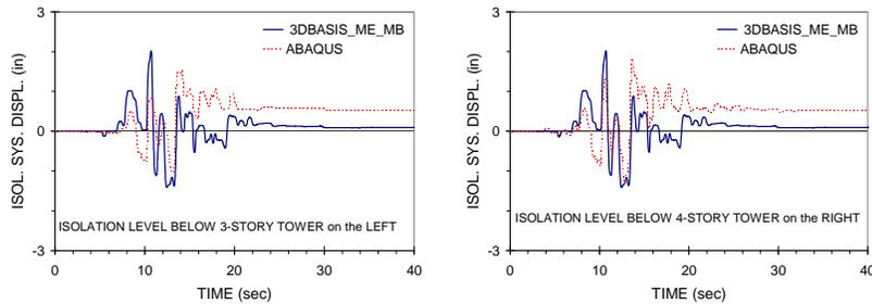
Figure 7. Isolation system displacement histories.
