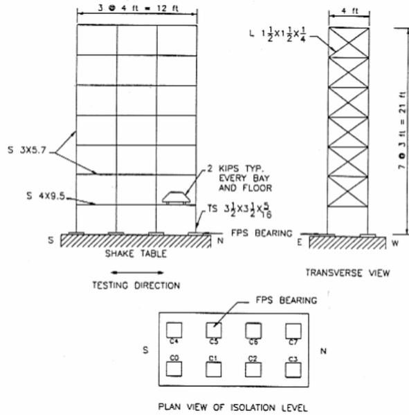
Figure 2. Schematic of seven-story model tested on shake table (Al Hussaini et al, 1994)
