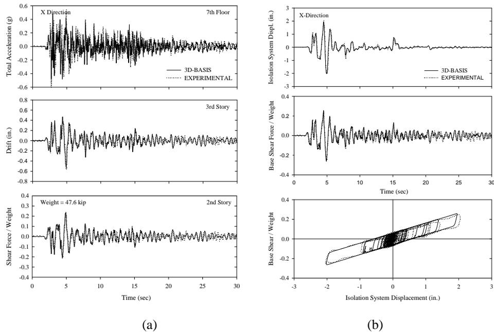
Figure 3. Comparison of experimental and 3D-BASIS-ME-MB results: (a) superstructure and (b) isolation system response in El Centro S00E 200%.
