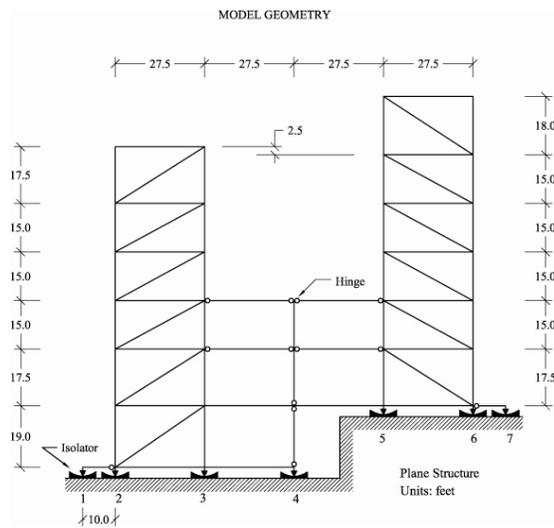
Figure 5. Schematic of two-tower split-level isolated structure
