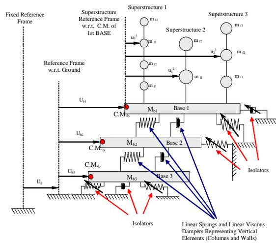
Figure 1. Degrees of freedom and reference frames in 3D-BASIS-ME-MB.
