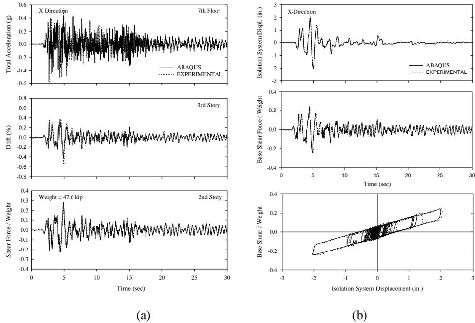
Figure 4. Comparison of experimental and ABAQUS results: (a) superstructure and (b) isolation system response in El Centro S00E 200%.
