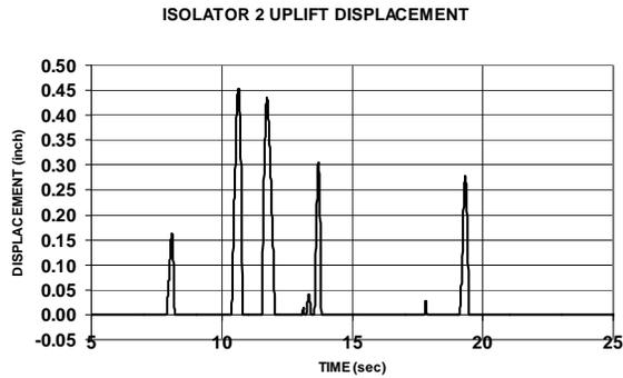
Figure 6. Uplift displacement history of isolator 2 as predicted in ABAQUS.
