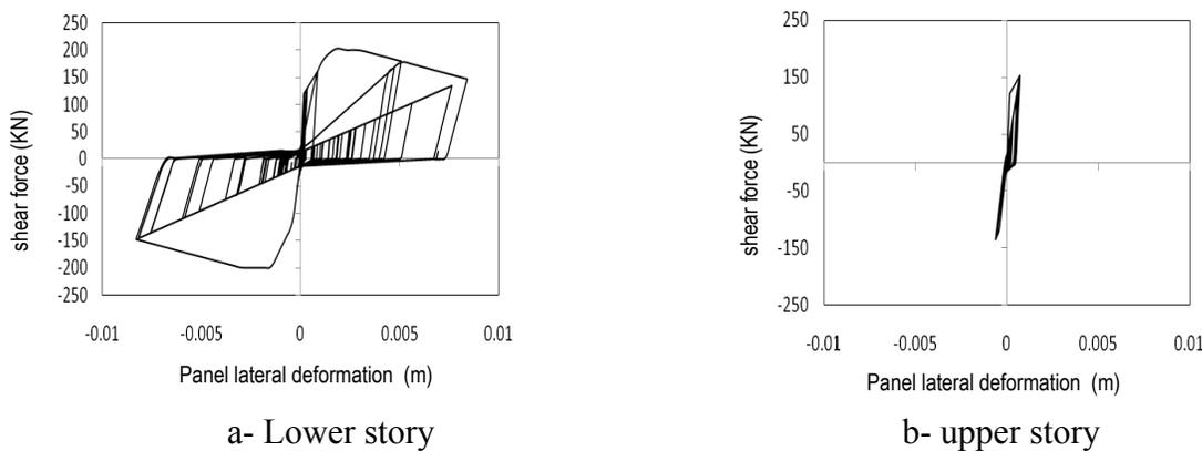
Figure 10. Shear-deformation curves of the shear walls
