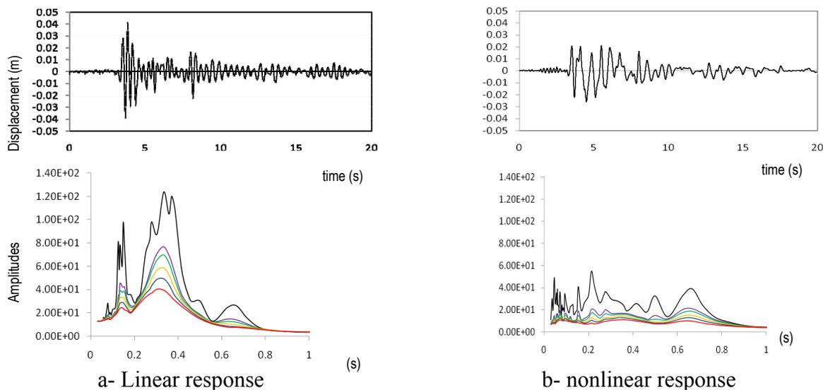
Figure 8. Top floor displacement time history and spectra responses
