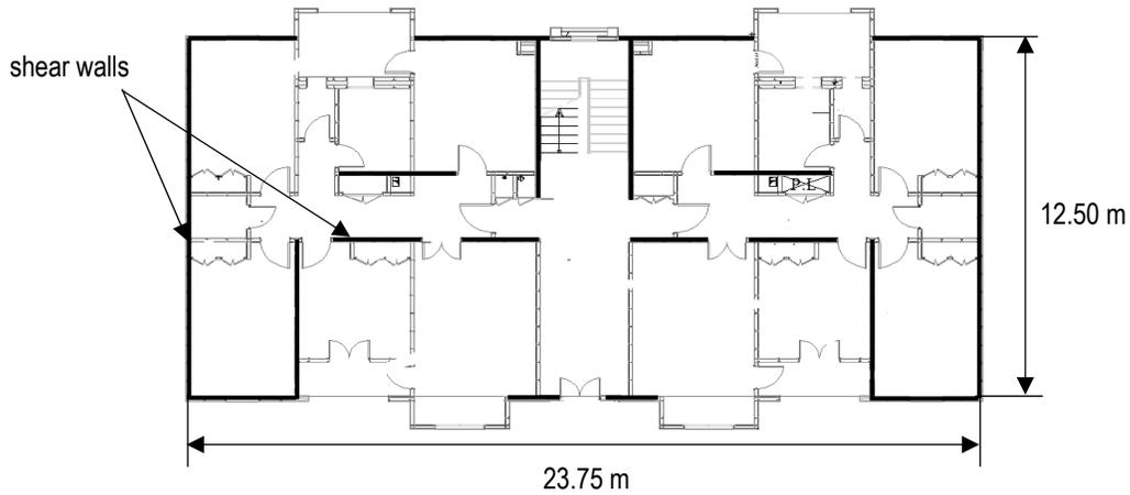
Figure 1. Building plan layout and shear walls locations
