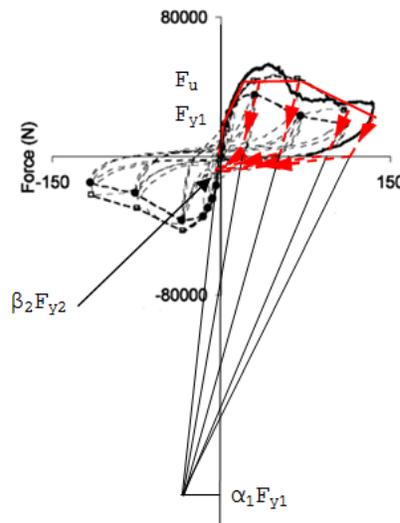
Figure 5. Typical experimental loops capture by a multilinear plastic pivot hysteresis model (CSI 2004) and (Fulop 2004)
