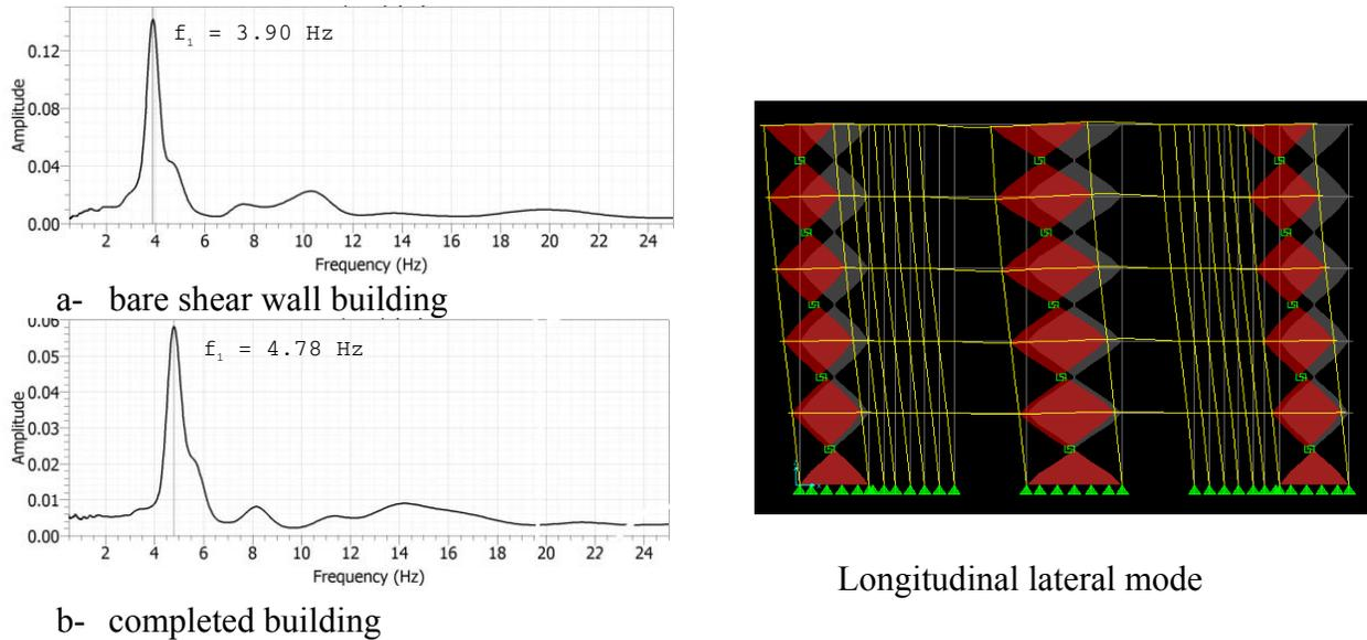
Figure 7. The measured FRF curves and the corresponding numerical longitudinal mode shape
