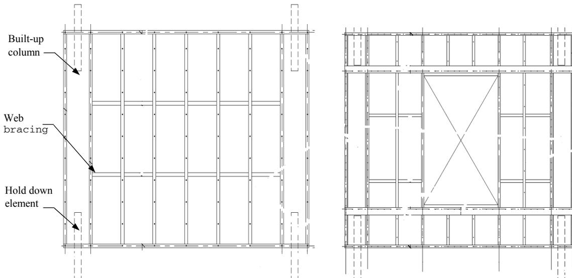
Figure 2. Typical shear wall panels with and without opening
