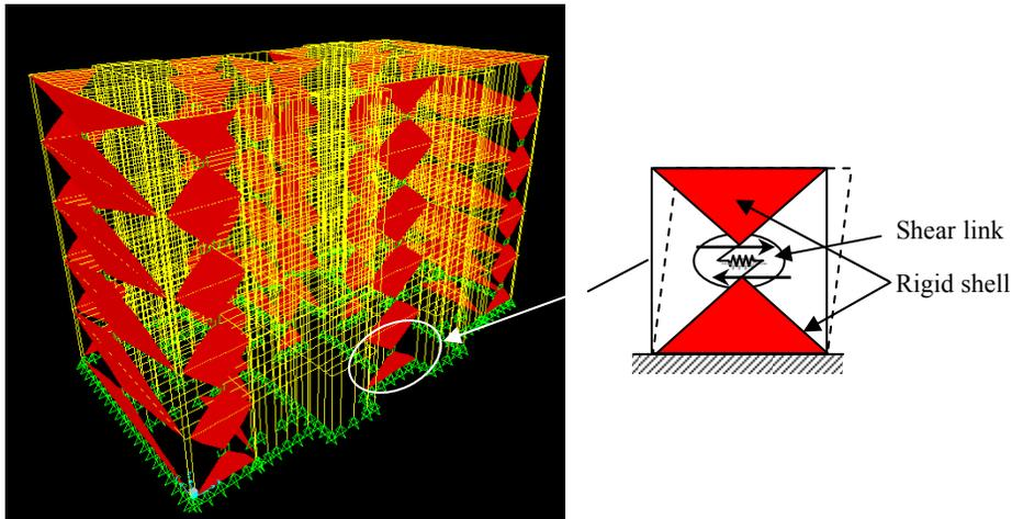
Figure 4. The 3-D model with an illustration of the shear link model of a panel
