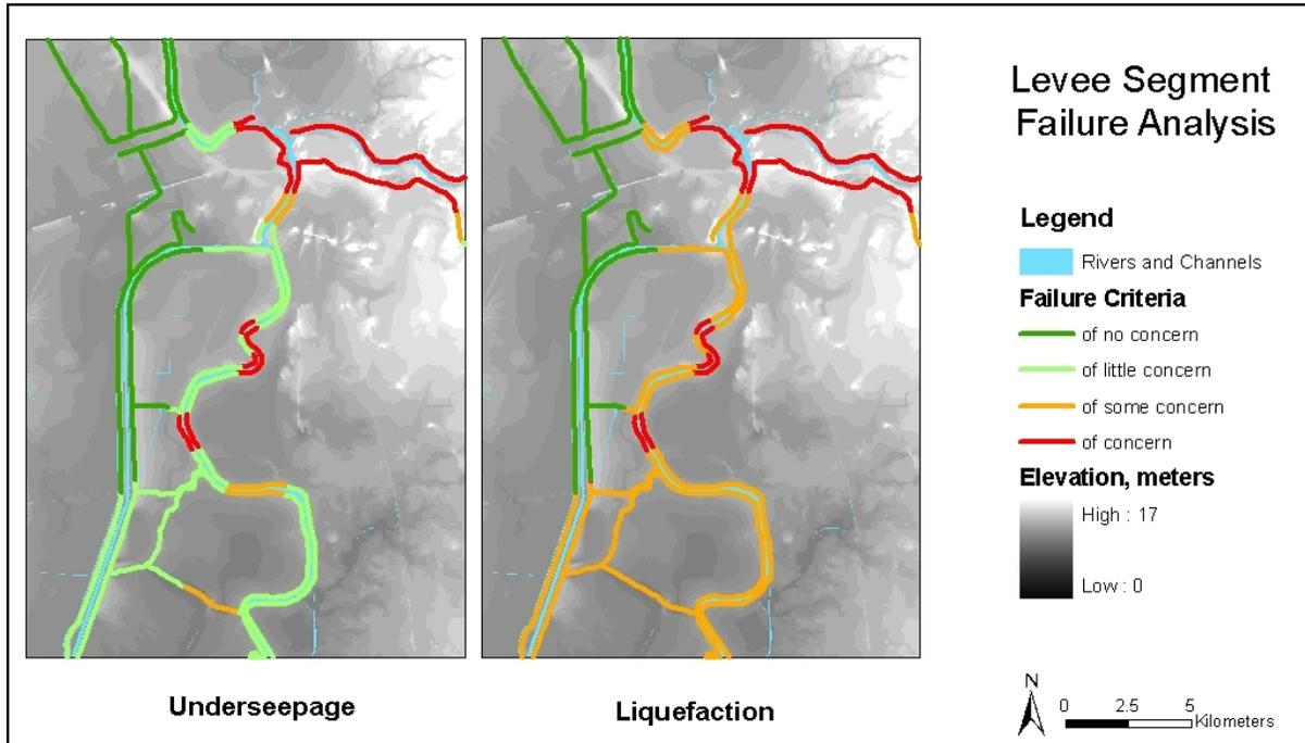
Figure 5. Results for failure analysis due to underseepage and liquefaction.
