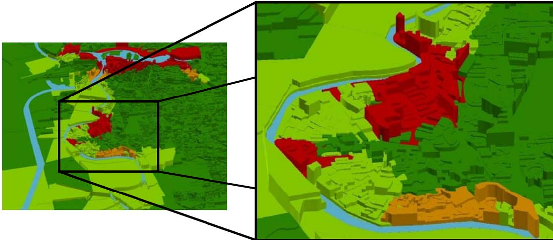
Figure 7. A 3D representation of population density (different heights) at the census block level, with flooded scenarios from underseepage levee failure (different colors)
