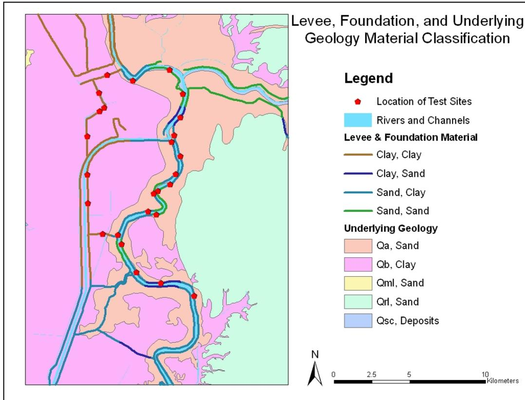
Figure 4. Levee and foundation material classification with underlying geology of the study area.
