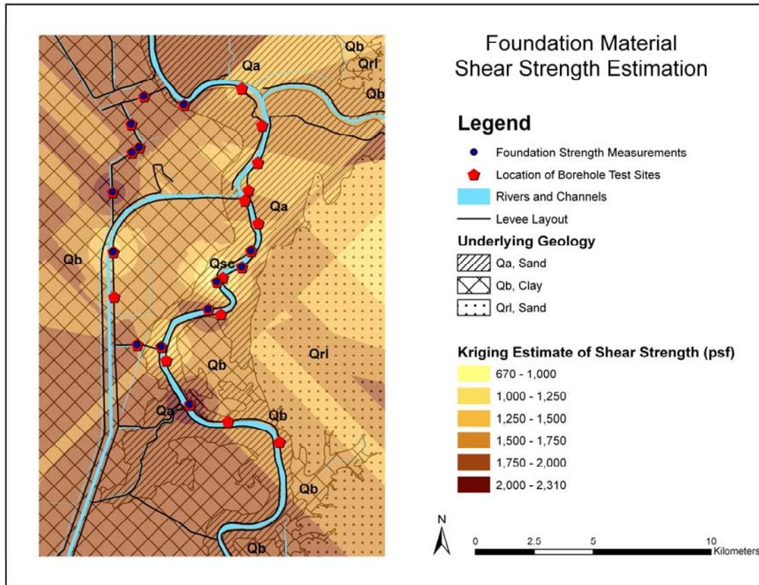
Figure 3. Kriging estimation of shear strength of the foundation layer along levee segments
