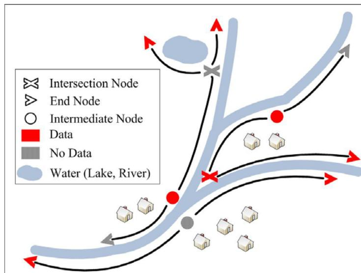
Figure 1. Proposed node classification and levee segmentation.
