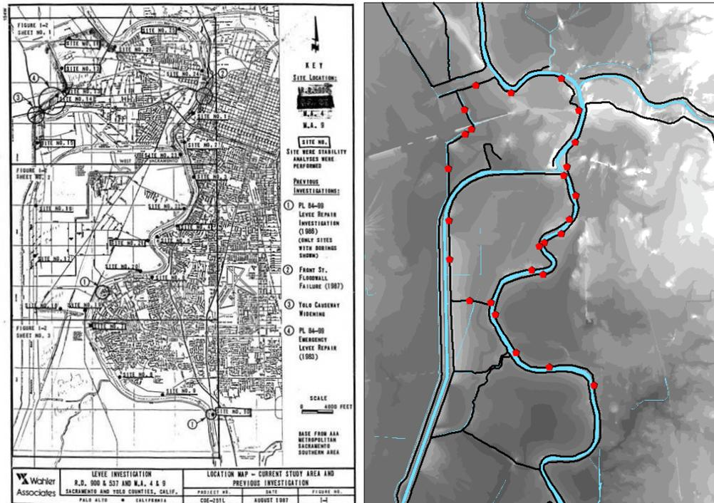
Figure 2. Levees (bold black lines) and soil test locations (red dots) represented in ArcGIS software environment with corresponding boring investigation data.
