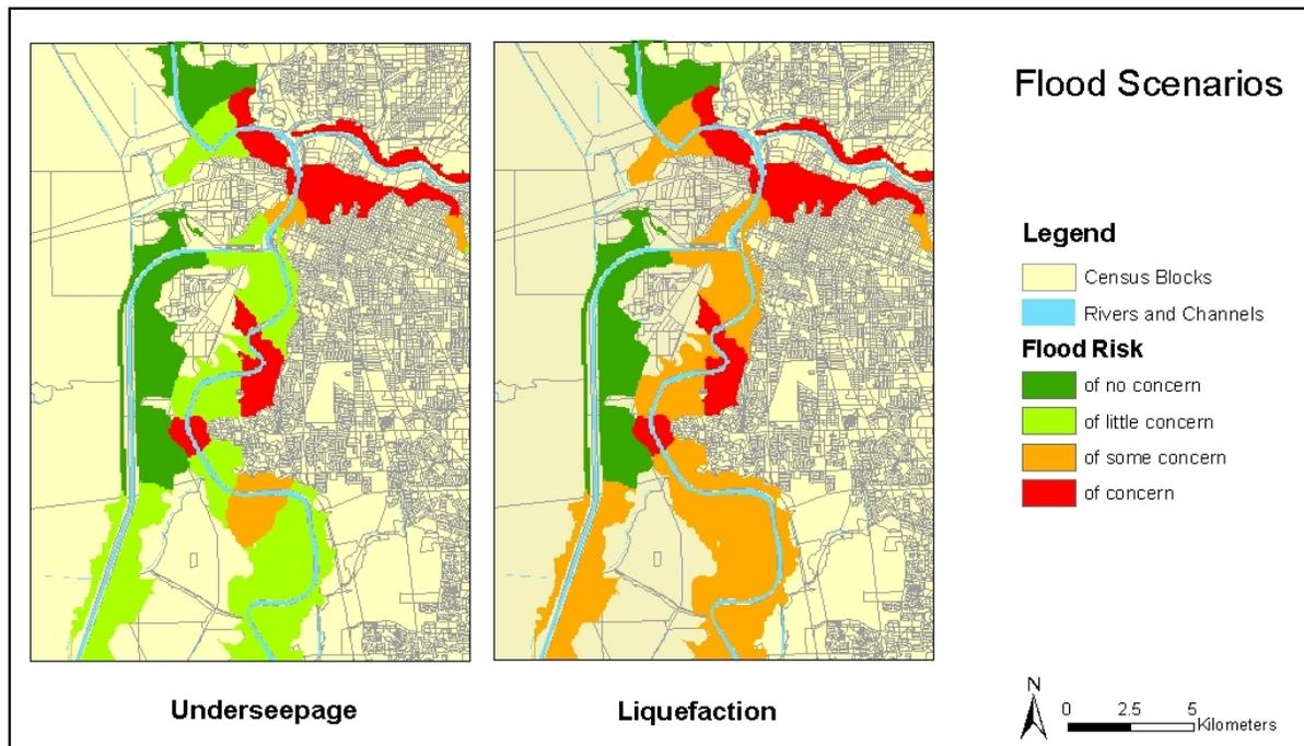
Figure 6. Flood scenarios from underseepage and liquefaction failures for all levee segments.
