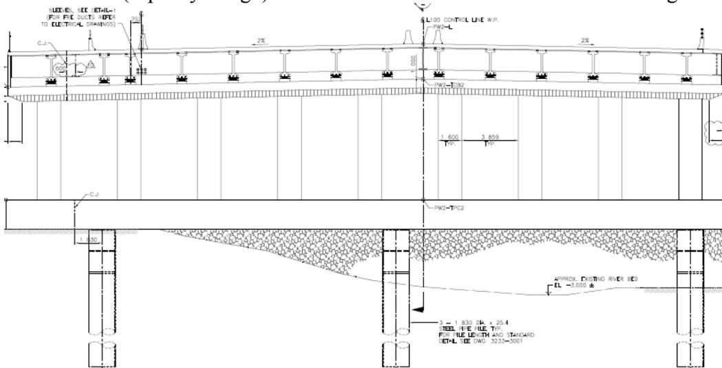
Figure 9. W2 pier arrangement
