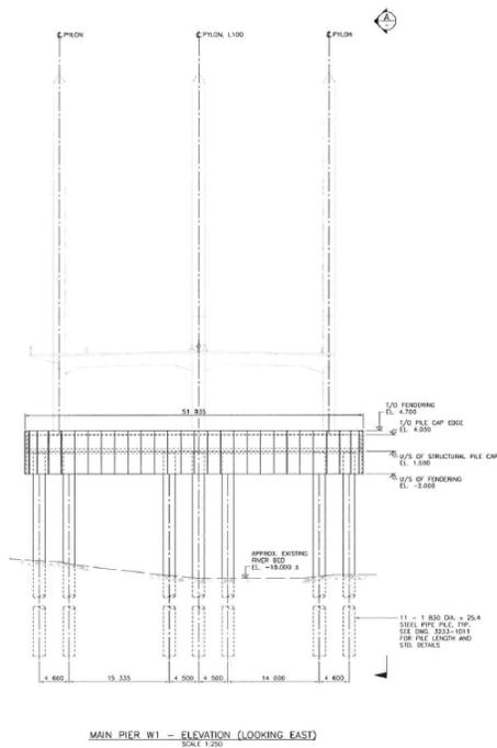
Figure 7. W1 Pier Arrangement
