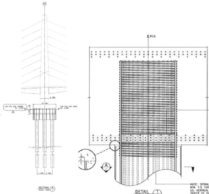
Figure 8. E1 Pile / Pile Cap Connection
