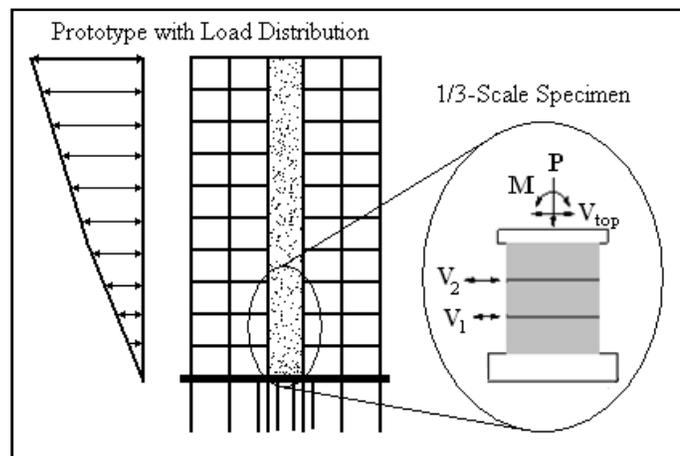
Figure 3. Extraction of test specimen loading from prototype structure loading.
