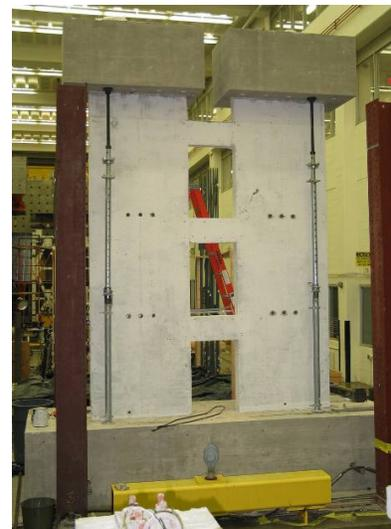
Figure 5. Coupled wall specimen.
