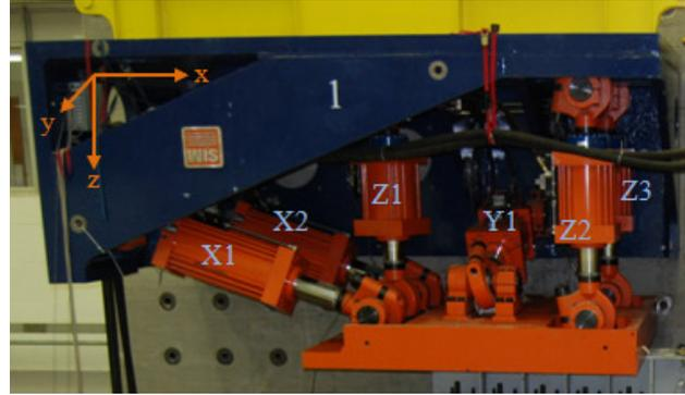
Figure 2. Typical LBCB with Cartesian axis and actuator names.
