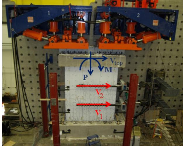
Figure 4. Representative test specimen with loading methods indicated.
