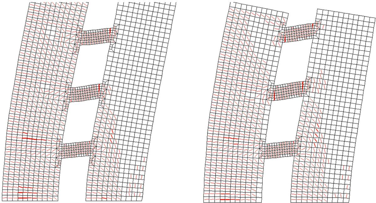
Figure 8. Crack maps for prototype (left) and test specimen (right) finite element analyses at peak load level. Note that thicker lines indicate larger cracks and that these regions of large deformation are common to both analyses.
