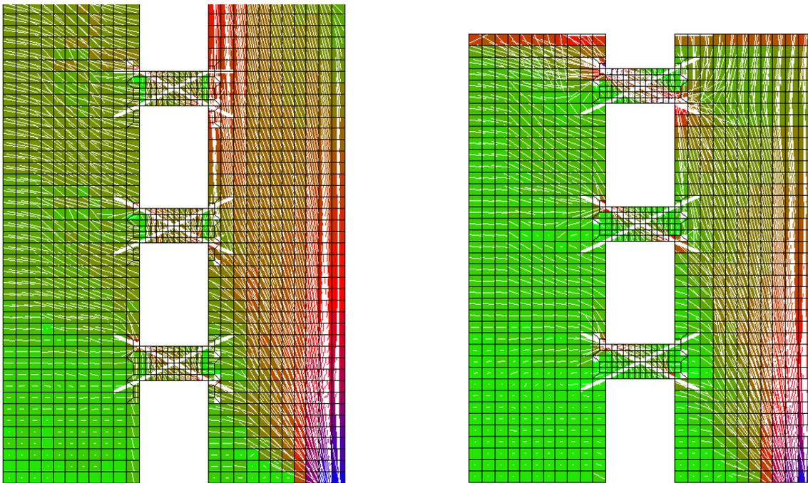
Figure 9. Principal compression stress trajectories for the prototype (left) and test specimen (right) finite element analyses at peak load level. Color gradients are not the same between models.
