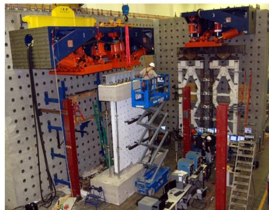
Figure 1. MUST-SIM reaction wall, LBCBs, and test specimens.
