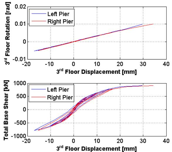
Figure 10. Displacement-rotation agreement and overall structural response.
