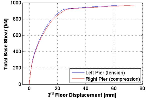
Figure 7. Load-displacement results for prototype pushover analysis.
