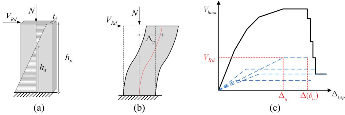
Figure 1. Procedure for determining the total capacity curve. (a) A wall in the bottom level under normal and lateral forces with the diagram of moments. (b) In-plane deformation of the wall. (c) Parameters of capacity curve for the walls (dashed) and the building (solid), where  $V_{base}$  is the base shear of the building.
