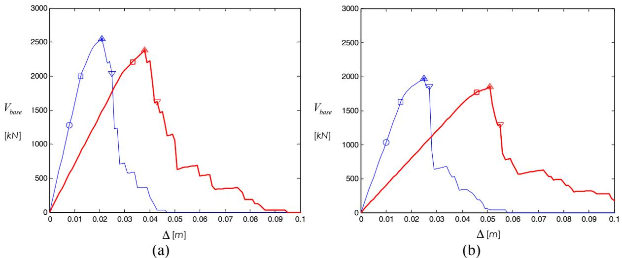
Figure 4. Capacity curves considering Lang method (blue) and proposed approach (red) over the X and Y directions. The damage grades are also showed: DG1  $\circ$ , DG2  $\square$ , DG3  $*$ , DG4  $\Delta$ , DG5  $\nabla$ . (a) X direction (b) Y direction.
