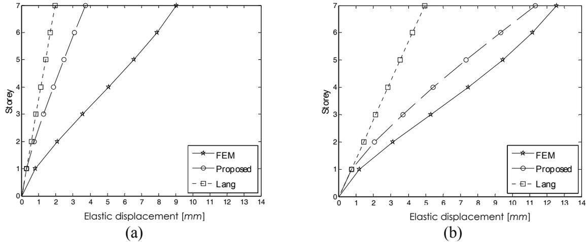
Figure 3. Elastic displacement following the X and Y directions of the studied building (Delémont). (a) Elastic displacement for the X-direction. (b) Elastic displacement for the Y-direction.
