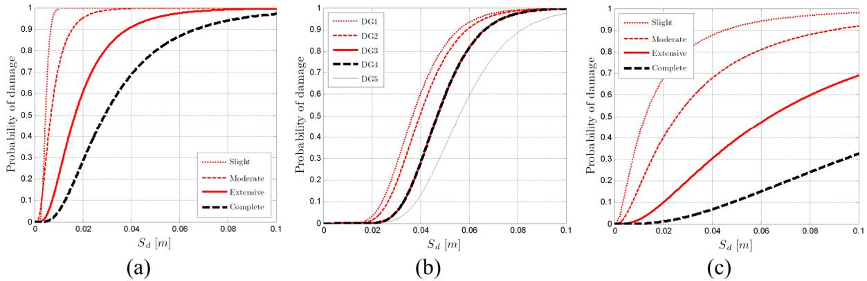
Figure 5. Fragility curves. (a) Using data from Risk-UE (class M3.3H). (b) Computed with proposed methodology. (c) Using data from HAZUS (class URMM).
