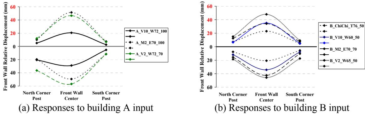
Figure 9. Response displacements of MOP-2R front wall
