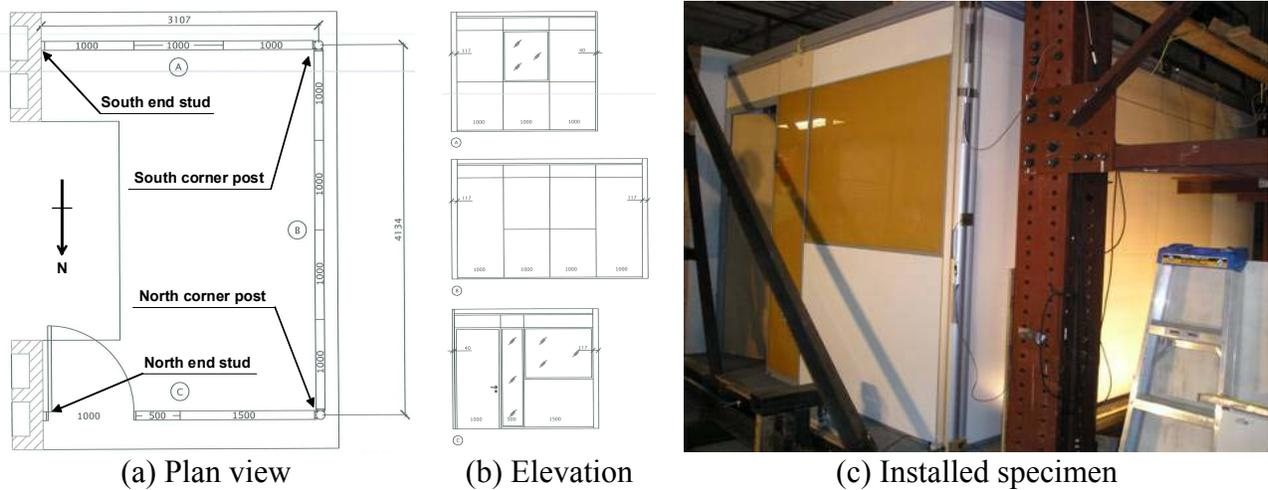
Figure 4. MOP test specimen (A and C are defined as the side walls, and B is the front wall)
