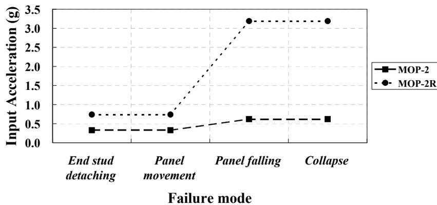
Figure 10. Evolution of the failure modes of the specimens during the tests
