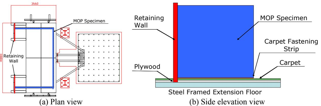
Figure 3. Testing setup
