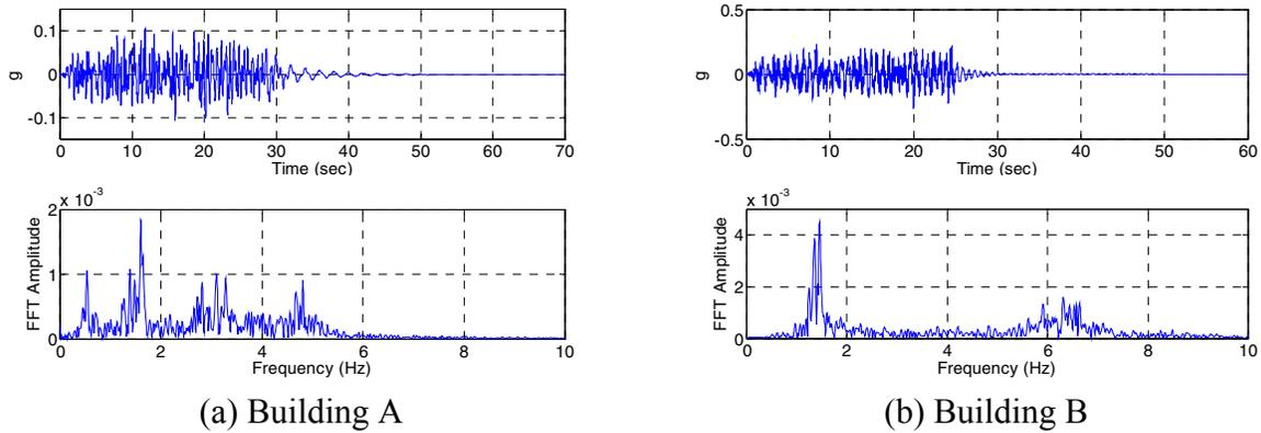
Figure 2. Top floor responses of two building models and their FFT spectra to the Eastern Canadian (Montréal 10%) design earthquakes
