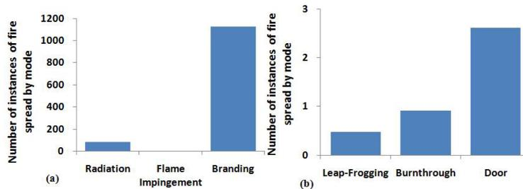
Figure 4. Spread by mode in Run 8: (a) building-to-building spread, (b) room-to-room spread, averaged over all simulations that spread beyond ignition building.
