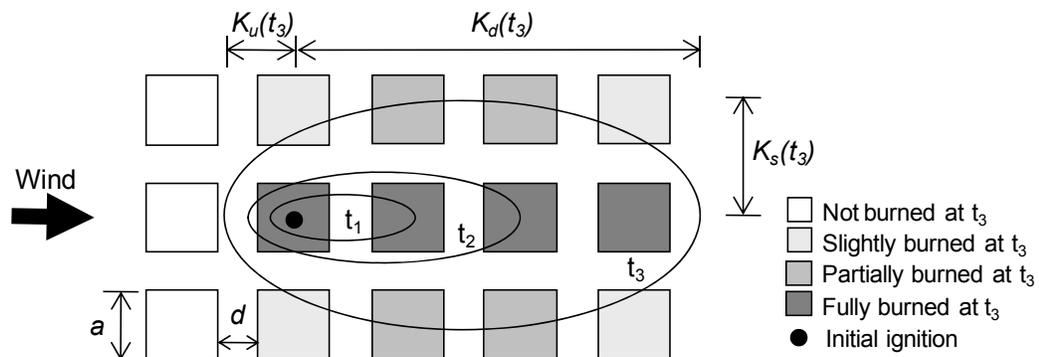
Figure 1. Hamada post-earthquake fire spread model (figure based on Scawthorn et al. 2005)
