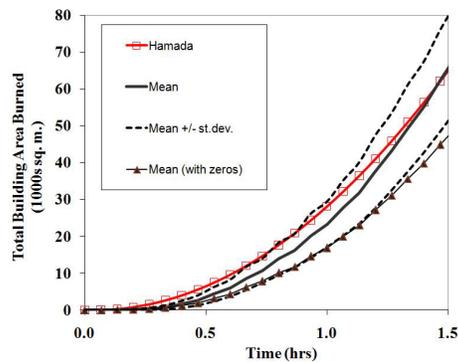
Figure 2. Total building area burned vs. time, for Run 8 with the Hamada model and the new model, mean +/- one standard deviation over only simulations that spread beyond the ignition building and over all 50 simulations.
