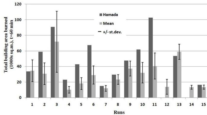
Figure 5. Building area burned at 60 minutes post-earthquake for all runs defined in Table 2. In each case, left column is Hamada model and right shows mean of new model averaged over all simulations that spread beyond ignition building, with errors bars for +/- one standard deviation.
