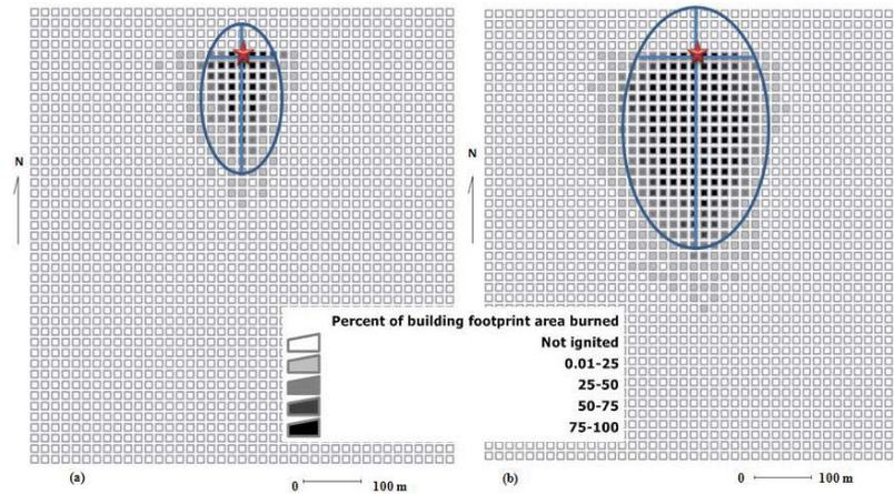
Figure 3. Spatial comparison of Run 8 results of the new model and the Hamada model (ellipses) at (a) 36 and (b) 60 minutes following ignition (star point), averaged over all simulations that spread beyond ignition building
