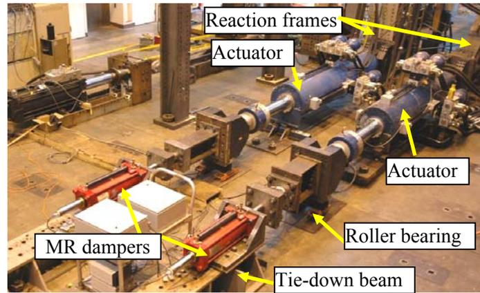
Figure 3. Experimental setup for real-time hybrid simulation
