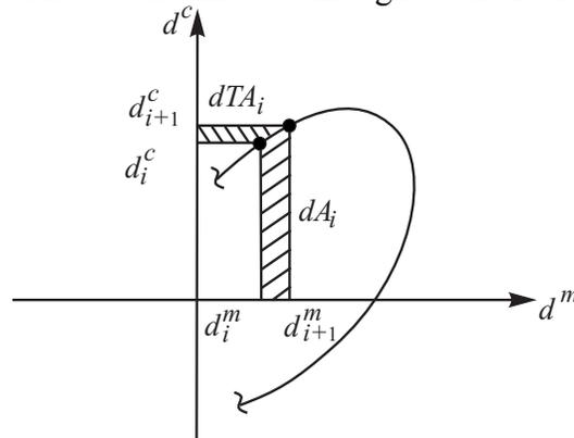
Figure 1. Hysteresis developed in synchronized subspace plot from actuator delay
