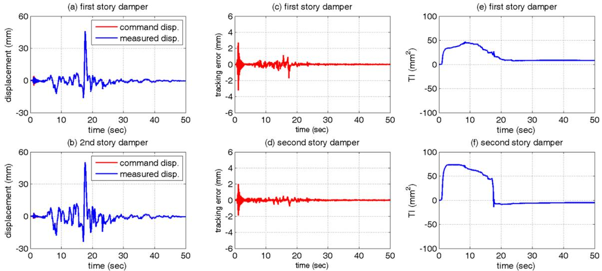
Figure 6. Real-time hybrid simulation results with  $\alpha_{es1}=0$ ,  $\alpha_{es2}=0$ ,  $k_p=0.4$ , and  $k_i=0.04$
