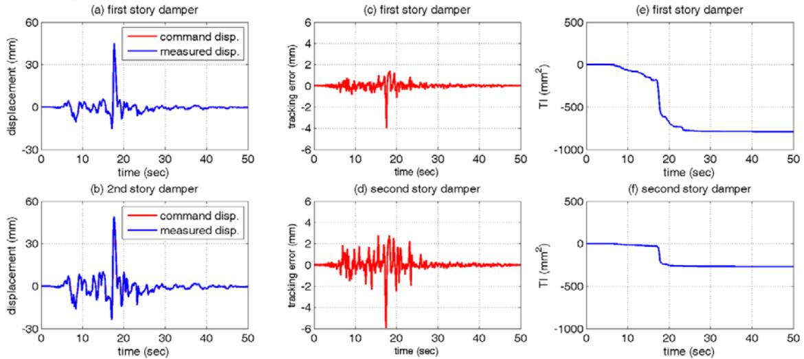
Figure 5. Real-time hybrid simulation results with  $\alpha_{es1}=60$ ,  $\alpha_{es2}=60$ ,  $k_p=0$ , and  $k_i=0$
