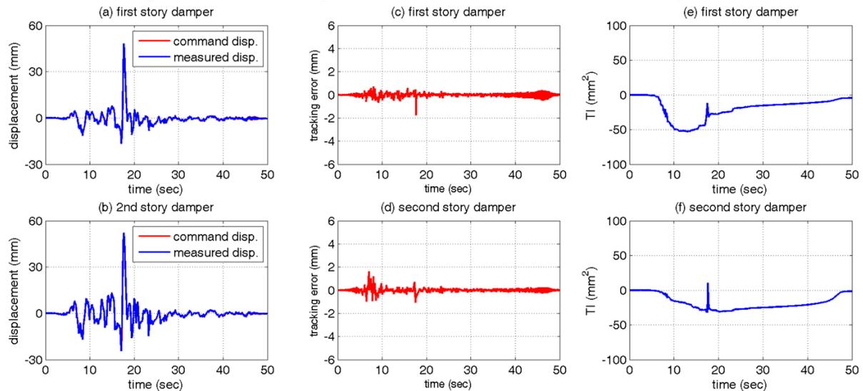
Figure 8. Real-time hybrid simulation results with  $\alpha_{es1}=60$ ,  $\alpha_{es2}=60$ ,  $k_p=0.4$ , and  $k_i=0.04$
