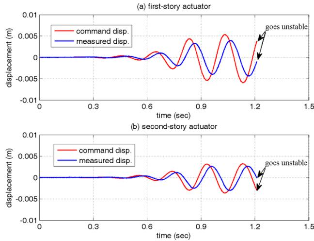
Figure 4. Real-time hybrid simulation results with  $\alpha_{es1}=0$ ,  $\alpha_{es2}=0$ ,  $k_p=0$ , and  $k_i=0$
