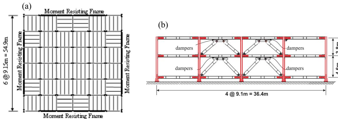
Figure 2. Prototype building (a) plan view; (b) perimeter MRF with dampers and braces
