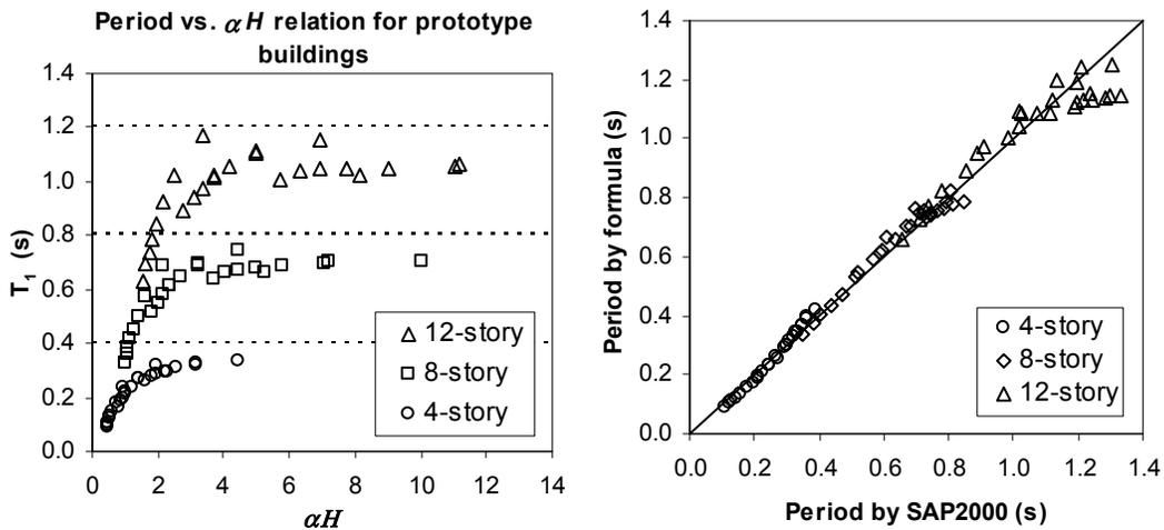
Figure 6. Fundamental period of prototype structures predicted using Eq. 14.
