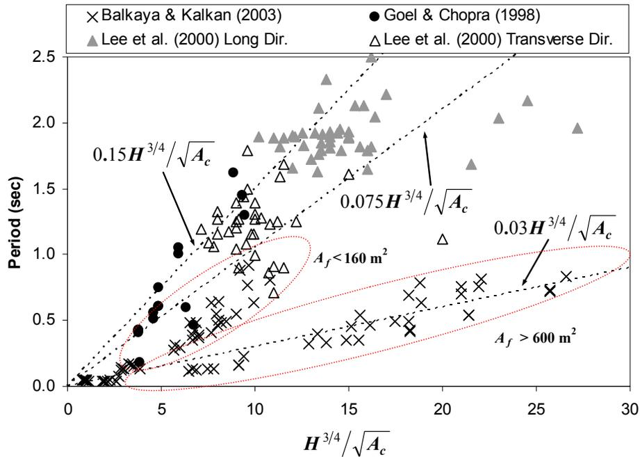
Figure 2. Comparison of measured and calculated building periods by Code formulation.
