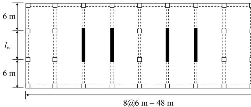
Figure 5. Plan view of bare frame configuration of the prototype frame wall structure
