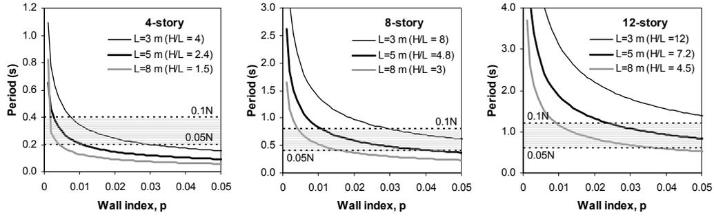
Figure 4. Periods calculated for range of wall indexes as a function of wall aspect ratio.
