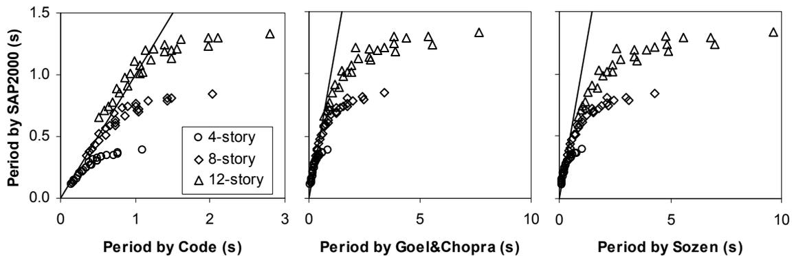
Figure 7. Estimations of existing formulas in case of frame-wall systems.
