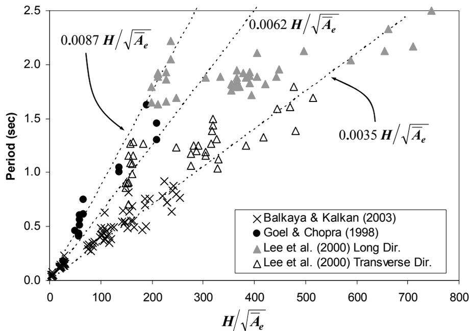
Figure 3. Comparison of measured and calculated periods by Goel and Chopra's formulation.
