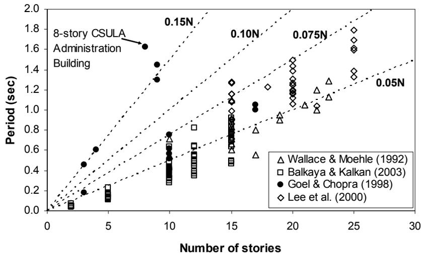
Figure 1. Period versus height relation of all shear wall buildings in the database
