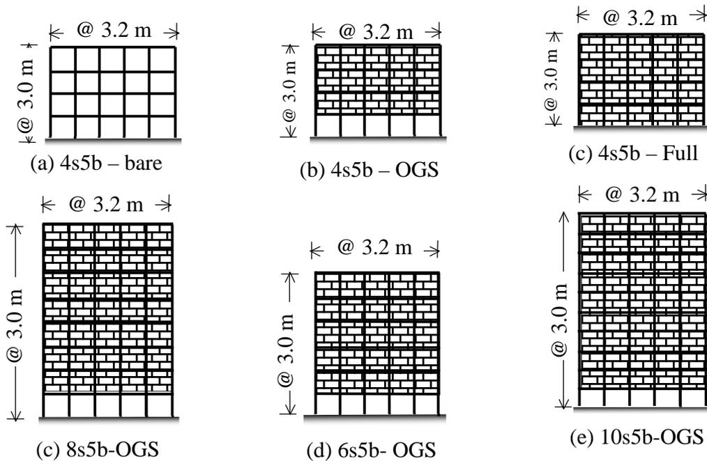
Figure 1. Details of bare frame and OGS frames considered
