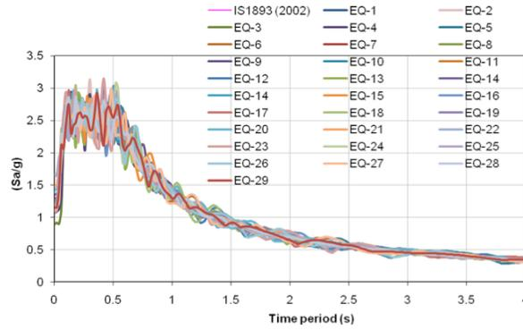
Figure 2. Response spectra generated from spectrum compatible ground motions
