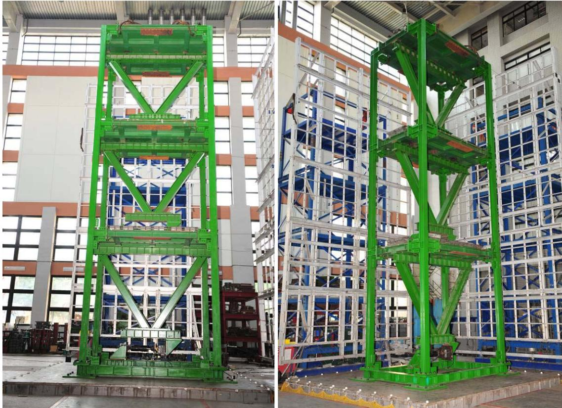
Figure 8: Photos of the three-story benchmark structure with passive damper in the first story.
