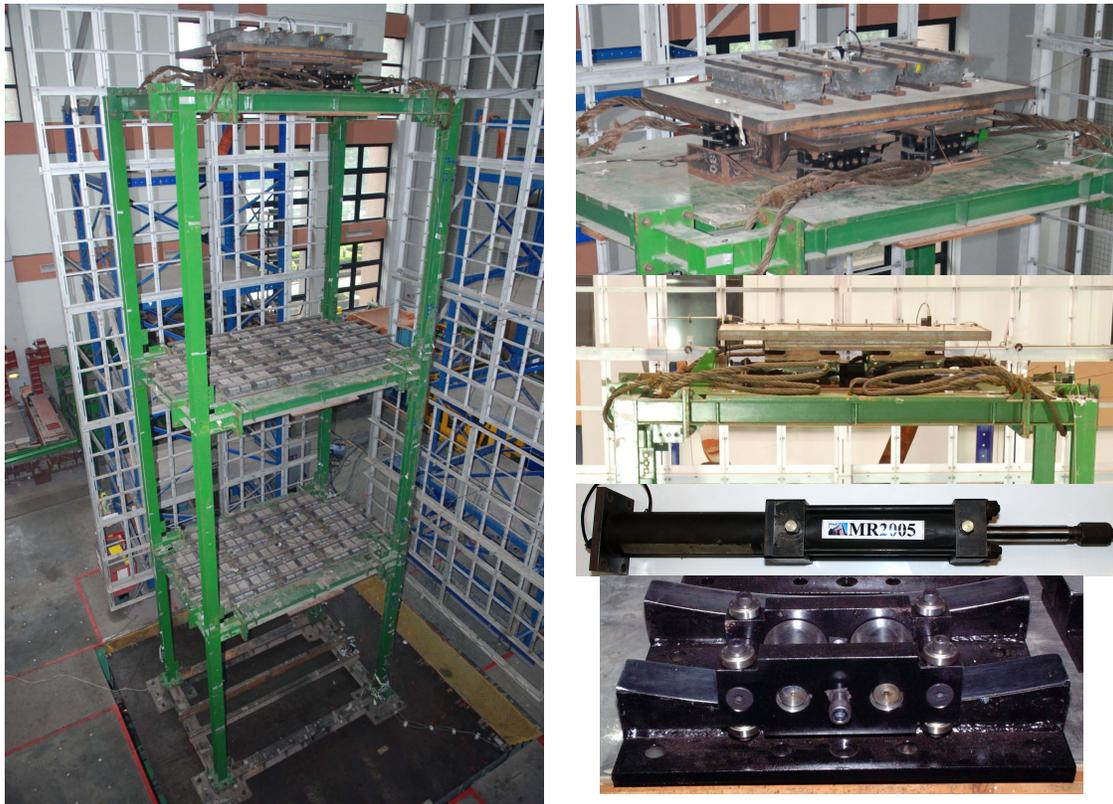
Figure 4: Set-up of the three-story benchmark structure
