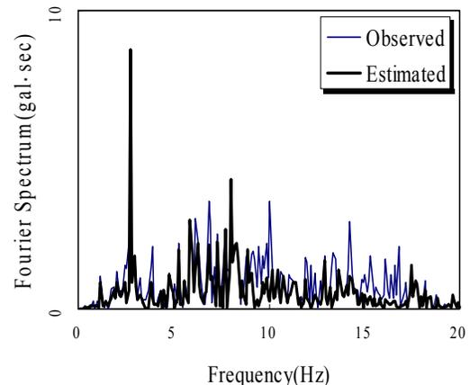
Figure 12. Target Fourier spectrum and its estimation calculated with the ground model identified in the 2nd stage.
