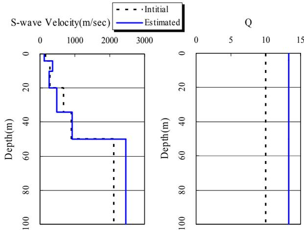
Figure 9. Identified shear wave velocity and quality factor in the first stage of identification
