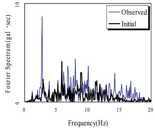
Figure 10. Target Fourier spectrum and its estimation calculated with the initial ground model
