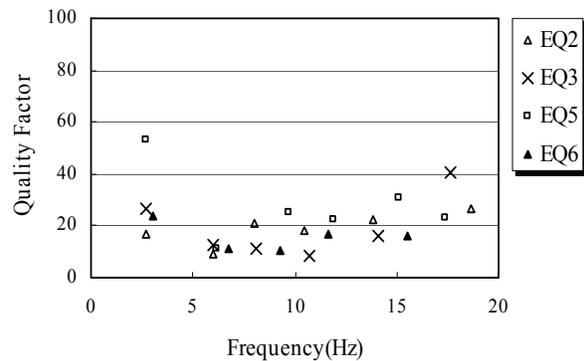
Figure 16. Estimated values of quality factor at IWTH08 in the third-stage identification using 4 events of earthquake
