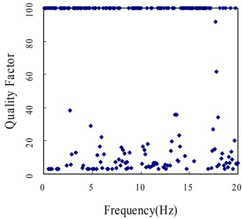
Figure 13. Quality factor estimated in the 2nd stage identification.
