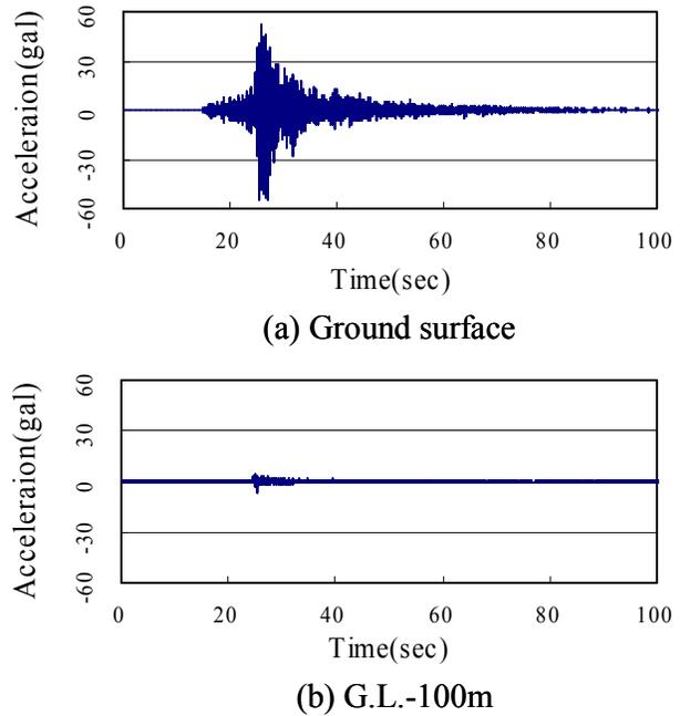
Figure 8. Acceleration of ground motions recorded at IWTH08 in the event EQ3
