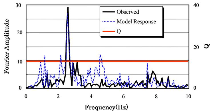
Figure 6. Comparison of observed Fourier spectrum and response of model identified in the 1<sup>st</sup> stage with identified quality factor
