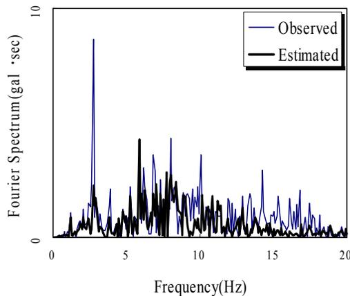
Figure 11. Target Fourier spectrum and its estimation calculated with the ground model identified in the 1st stage
