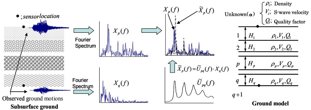
Figure 2. Schematic diagram of identification problem
