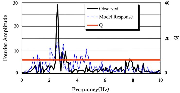
Figure 5. Comparison of observed Fourier spectrum and response of initial model with initially given quality factor
