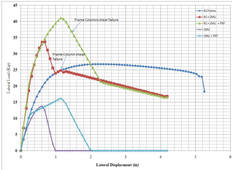
Figure 5. Pushover curve: in-plane loads versus lateral displacement
