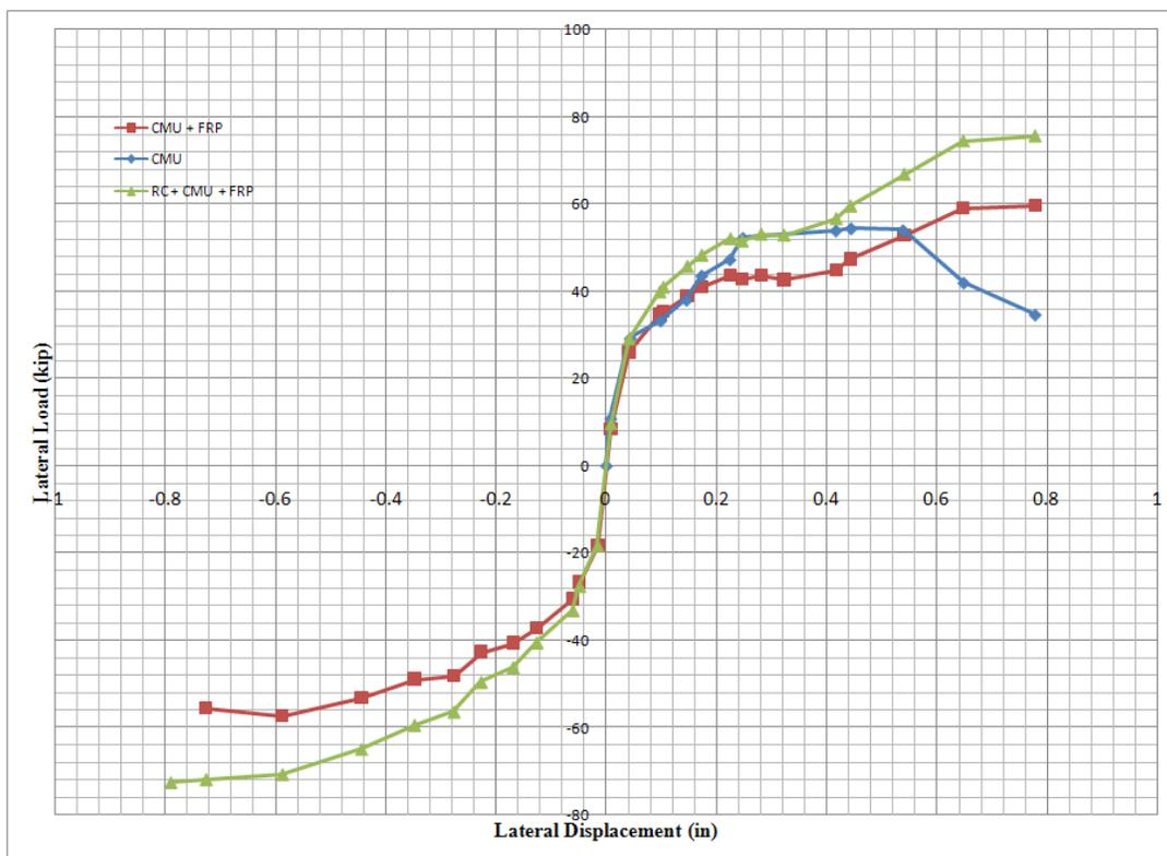
Figure 4. Masonry infill system laboratory test results by (Gustavo et. al. 2001)
