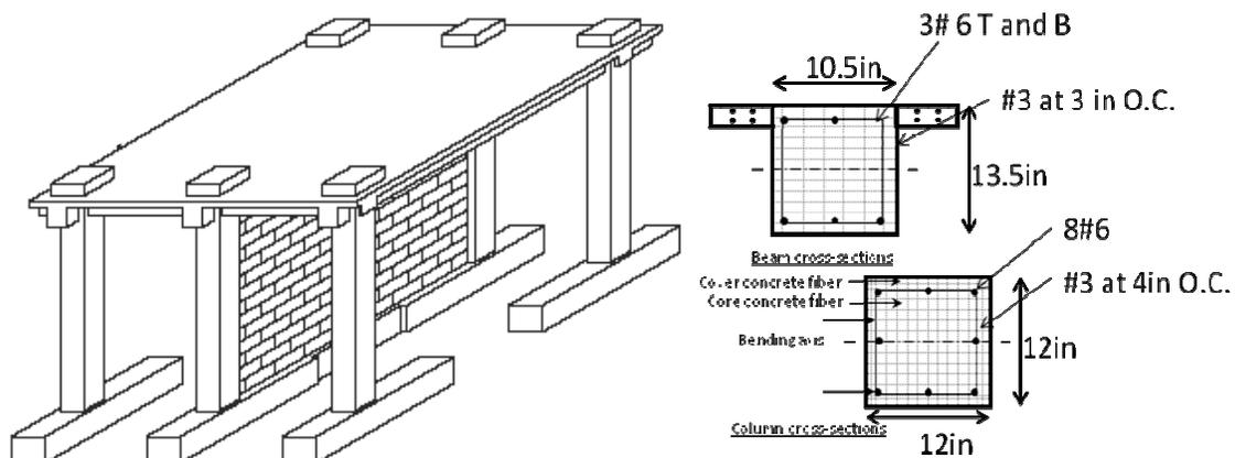
Figure 1. Specimen geometry and RC frame cross-section (FE discretization)
