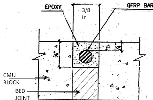
Figure 3. NSM GFRP bars in CMU bed joints
