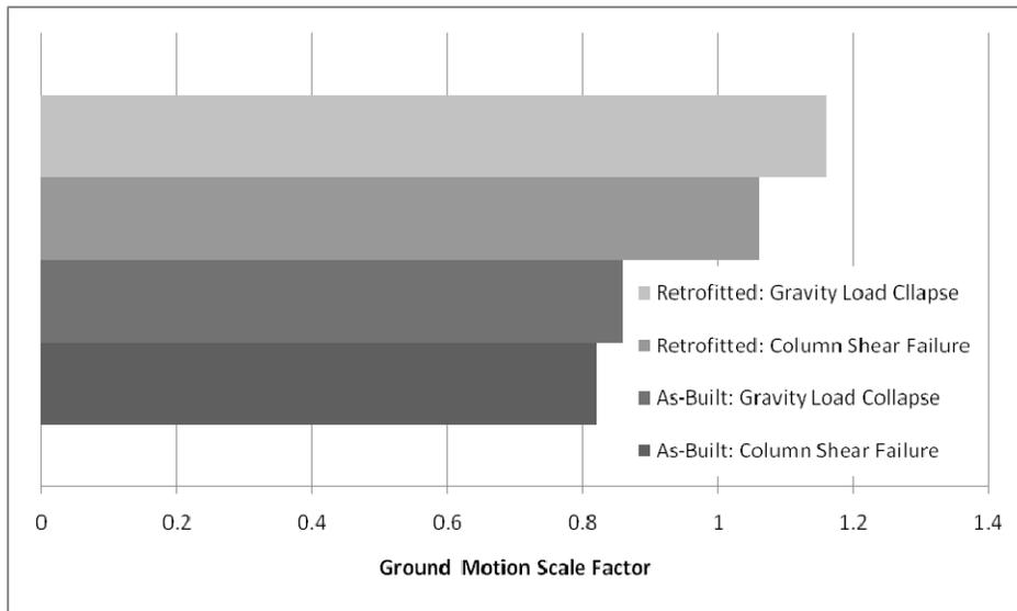
Figure 6. Ground motion scale factors at shear failure and gravity load collapse
