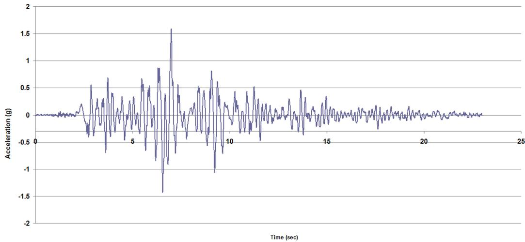
Figure 2. Northridge(1994) ground acceleration record (Tarzana, 90°)
