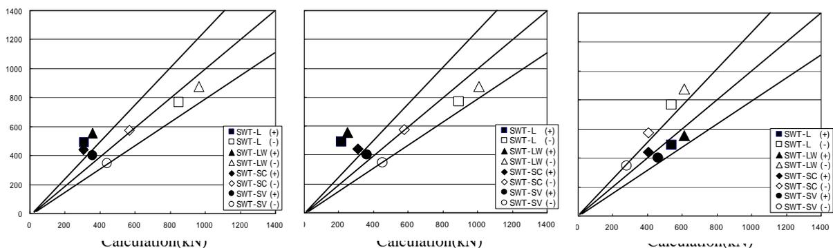
Figure 4. Comparison of observed and calculated shear strengths
