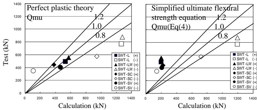
Figure 5. Comparison of calculated and observed flexural strengths
