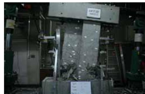
Figure 3. Hysteretic relations and collapsed specimens
