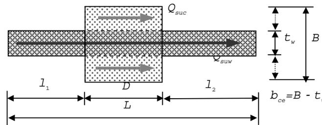
Figure 2. Dividing the column section with wing wall
