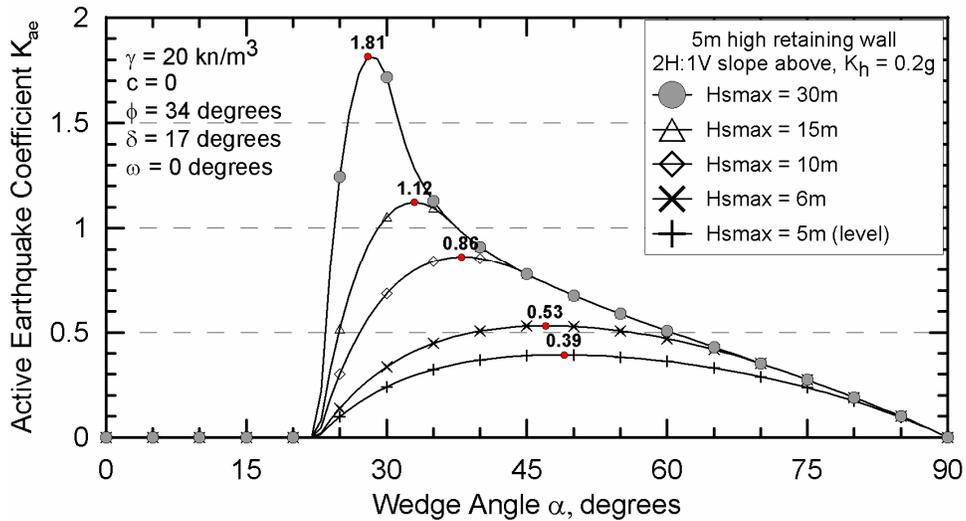
Figure 5. Variation of active seismic pressure coefficient with maximum slope height and wedge angle
