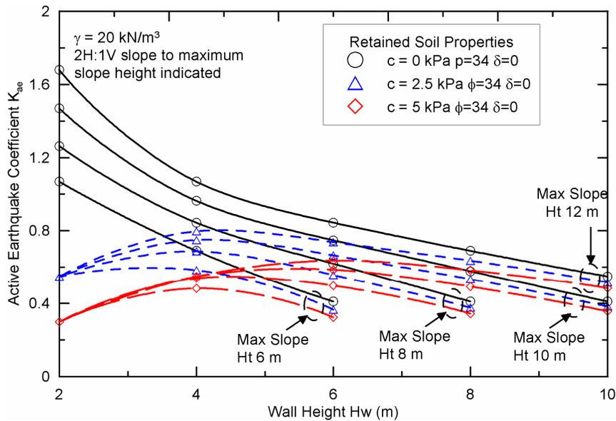
**Figure 4. Typical results for variable wall height and cohesion (constant embankment height, soil properties, and horizontal coefficient)**
