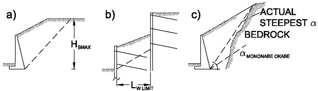
Figure 2. Practical retaining wall geometries for which M-O equation is conservative a) wall with limited slope height, b) wall with limited length of failure wedge, and c) wall with restricted failure angle.
