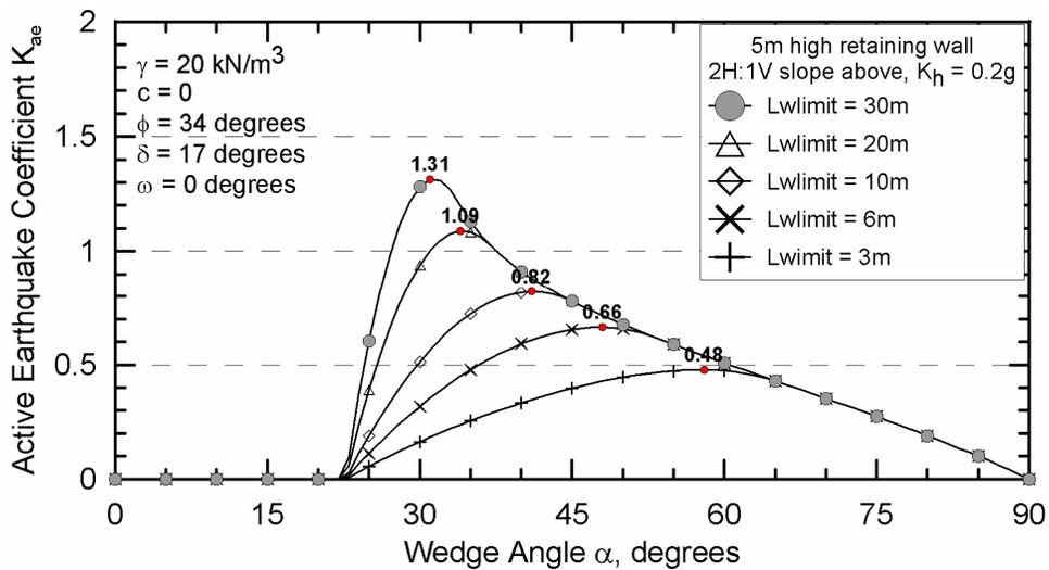
Figure 6. Variation of active seismic pressure coefficient with horizontal limit and wedge angle
