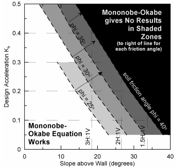
Figure 1. Design conditions for which the Mononobe-Okabe equation does not work
