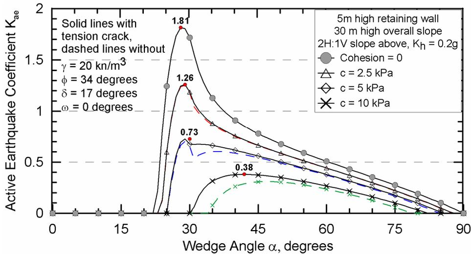
Figure 7. Variation of active seismic pressure coefficient with cohesion and wedge angle
