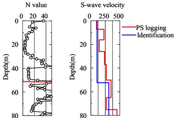
Figure 6. N value and shear wave velocity estimated by PS logging and identification at site A in Tokushima city
