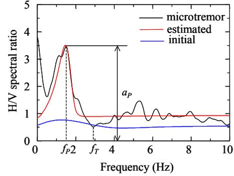
Figure 2. H/V spectral ratios of microtremors and theoretical Rayleigh wave
