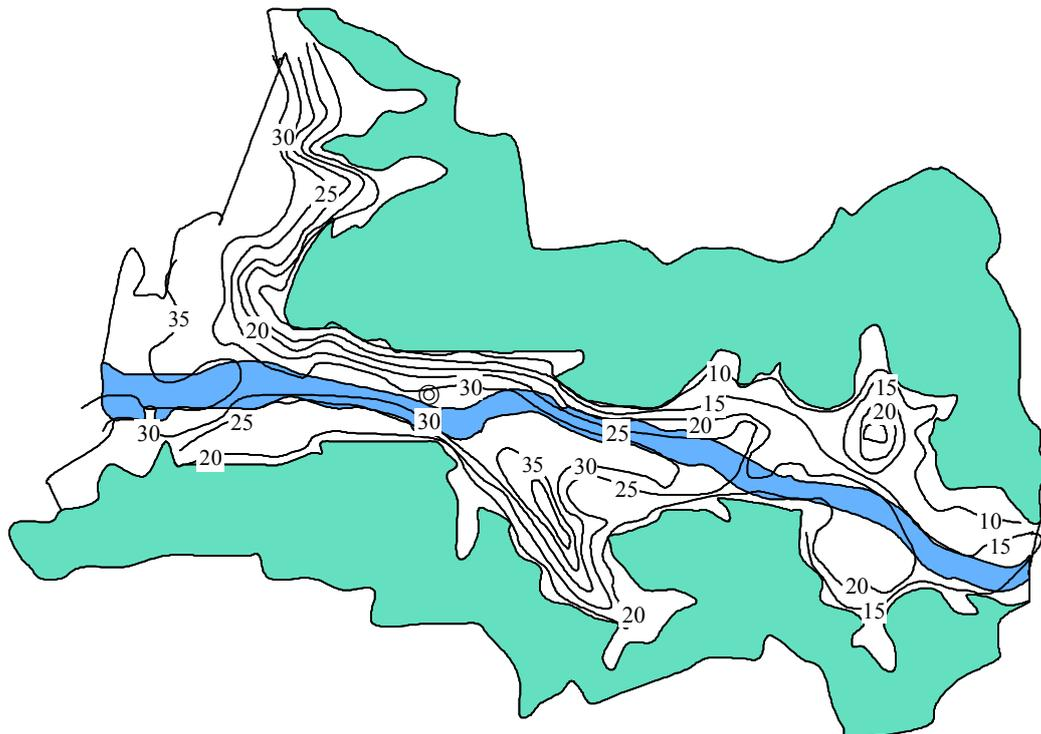
Figure 13. Conventional study on the depth of top of engineering bedrock estimated in Arida city [Tsujiyama et al (2003)]
