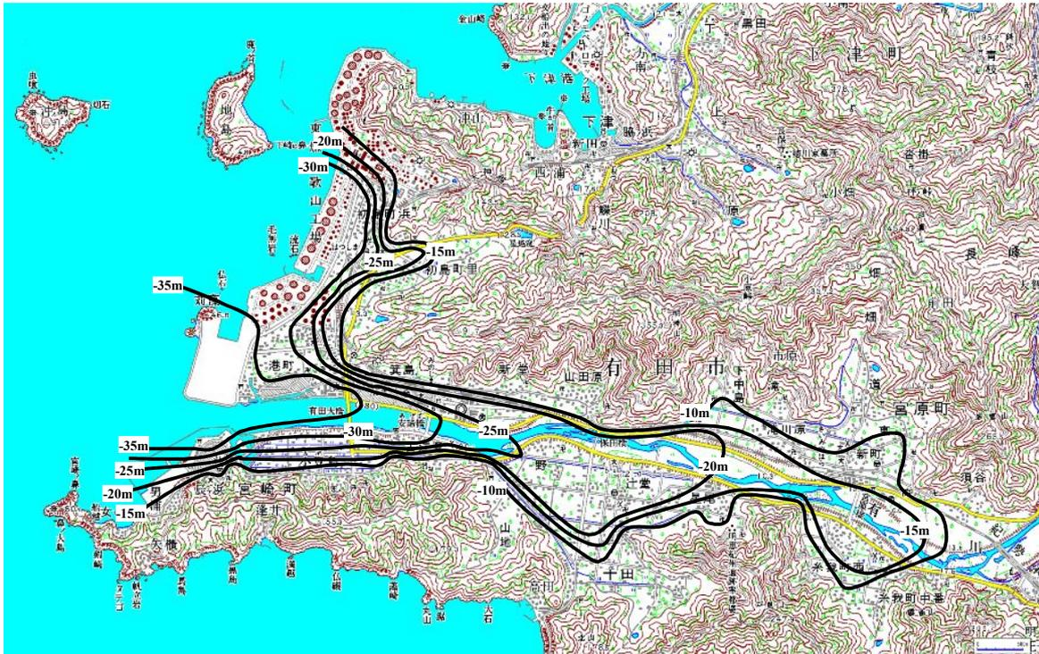
Figure 12. Contour map of depth of top of engineering bedrock estimated with microtremors in Arida city
