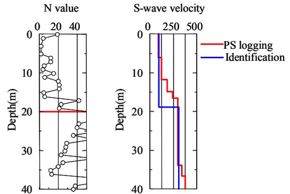
Figure 7. N value and shear wave velocity estimated by PS logging and identification at site B in Tokushima city
