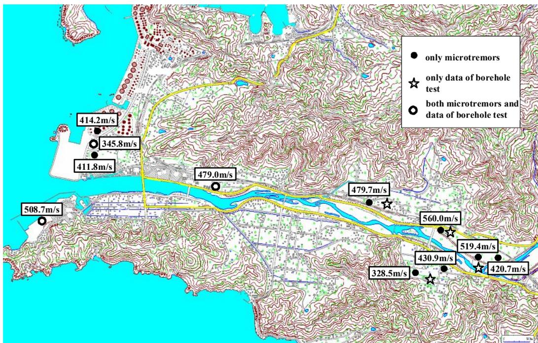
Figure 9. Shear wave velocity estimated in the first-stage identification in Arida city
