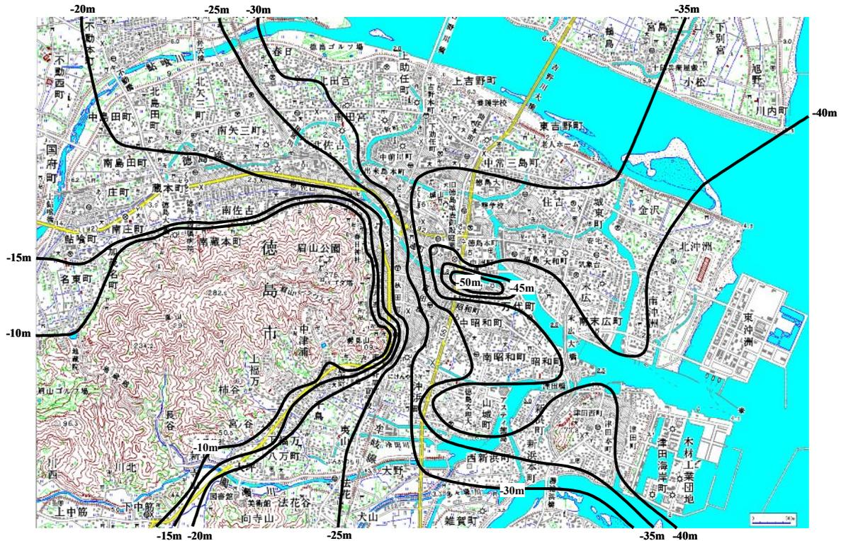
Figure 8. Contour map of depth of top of engineering bedrock estimated with microtremors in Tokushima city
