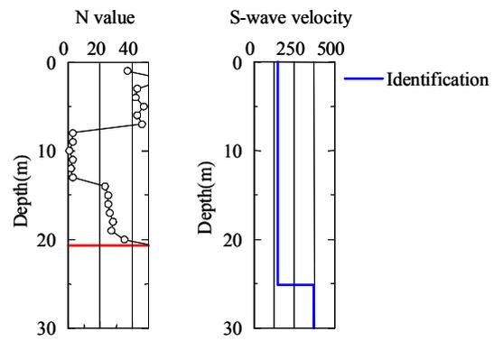
Figure 11. N value and shear wave velocity estimated by PS logging and identification at site D in Arida city
