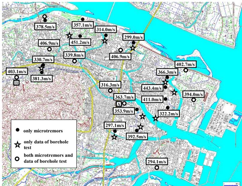
Figure 5. Shear wave velocity estimated in the first-stage identification in Tokushima city
