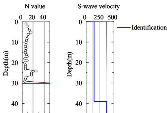
Figure 10. N value and shear wave velocity estimated by PS logging and identification at site C in Arida city
