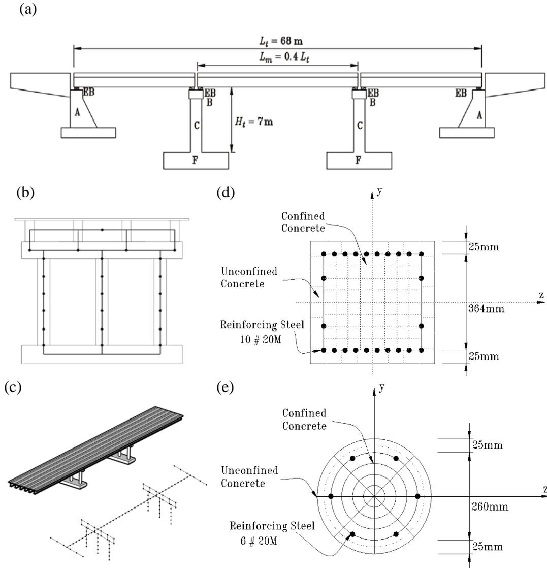
Figure 2. MSSS Concrete Geometric Description. (a) Mean Bridge Elevation, where A = abutments, EB = elastomeric bearings, B = transverse beams, C = columns, F foundations. (b) Bridge Bent Cross Section and Model Representation, (c) 3D FE Model, (d) Transverse Beam Fiber Section and (e) Column Fiber Section.
