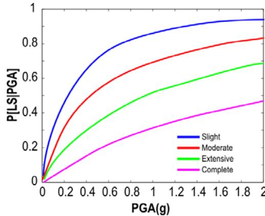
Figure 5. Fragility Curve for the MSSS Concrete Girder.
