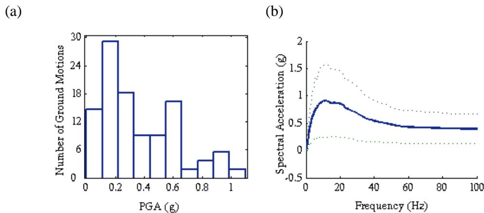
Figure 3. GMTHs Series. (a) PGA distribution of ground motions and (b) Mean and Standard Deviation Response Spectrum.
