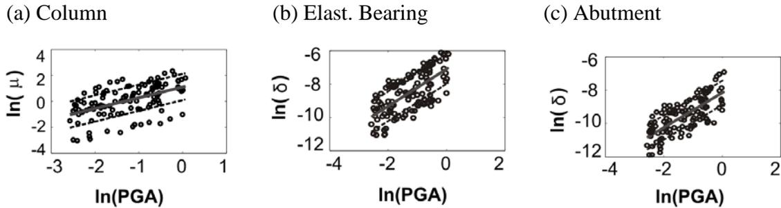
Figure 4. Regression of the probabilistic seismic demand models of the MSSS Concrete Girder for: (a) Columns, (b) Elastomeric Bearing and (c) Abutment.
