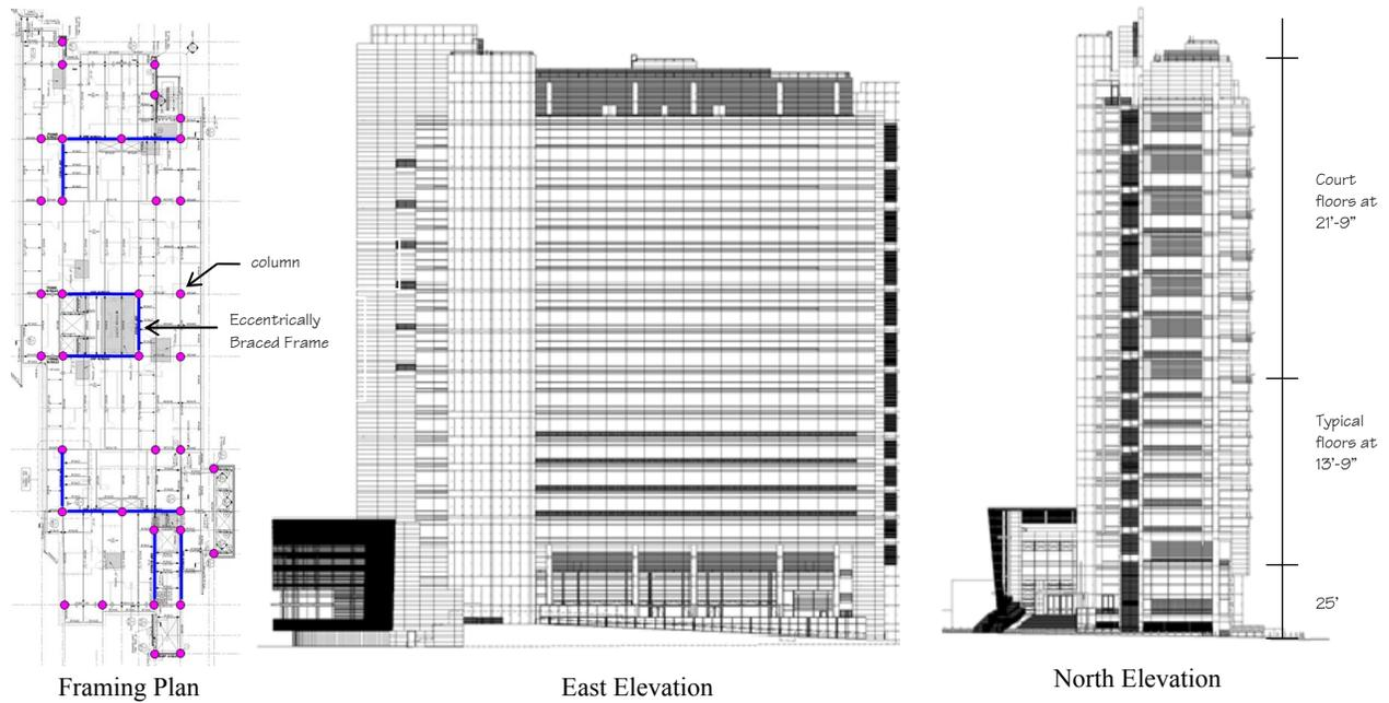
**Figure 1.** Framing plan and elevations
