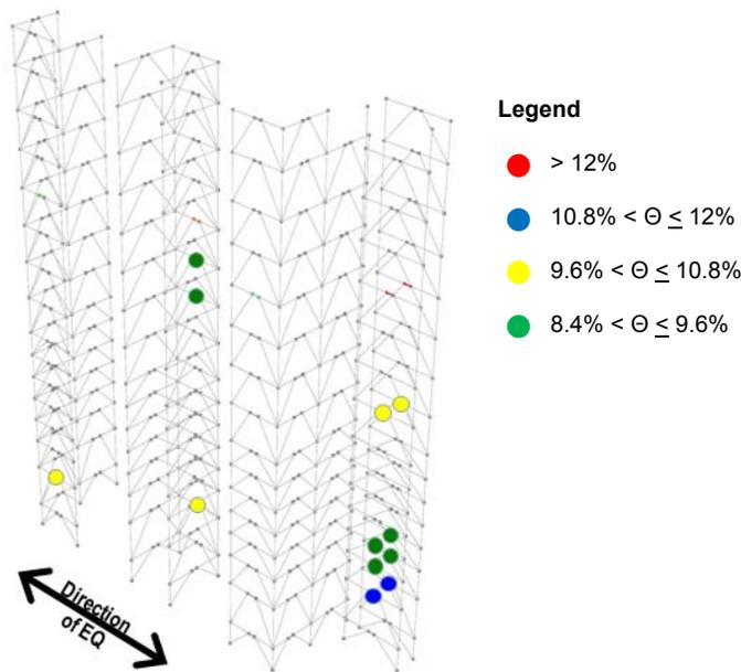
**Figure 2.** Link beam limit state for Sylmar Earthquake
