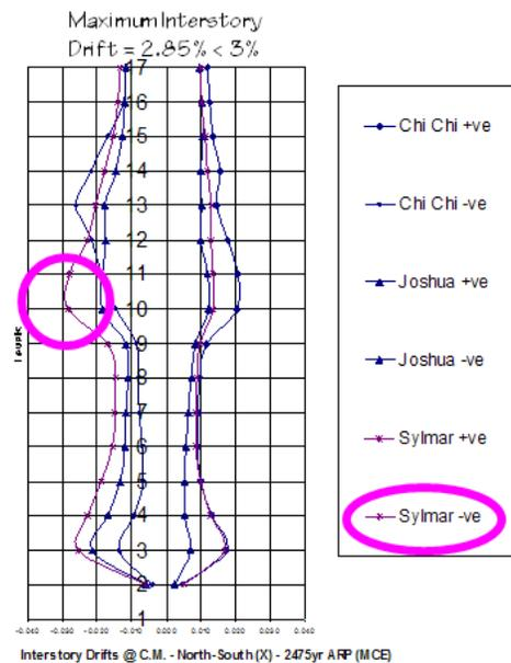
**Figure 3.** Interstory drift in north-south direction
