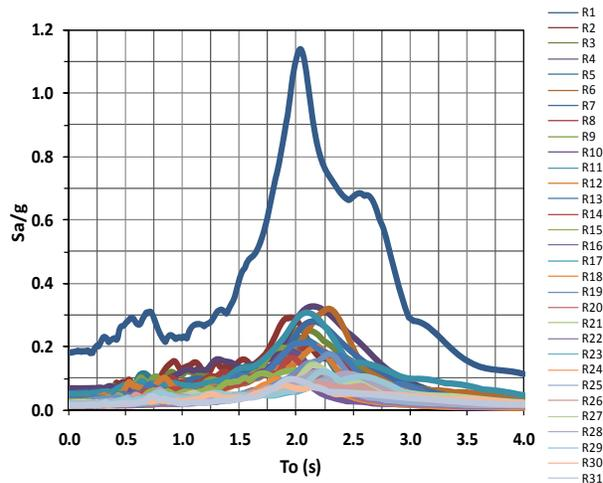
Figure 4. Elastic pseudo-acceleration spectra for  $\xi = 0.05$ .
