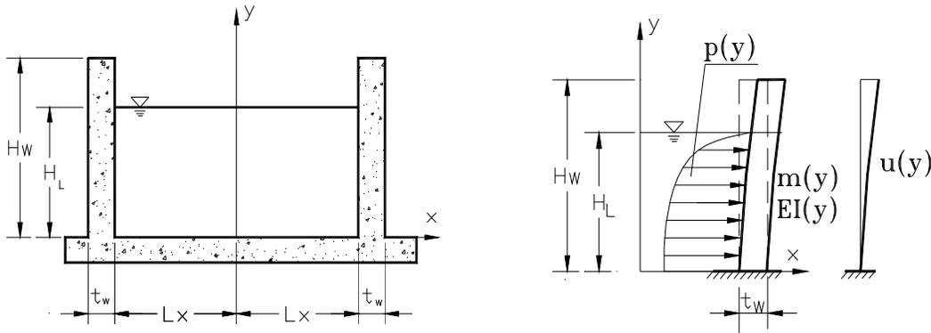
(a) 2-D model of rectangular tank (b) Analysis model using generalized SDOF system
