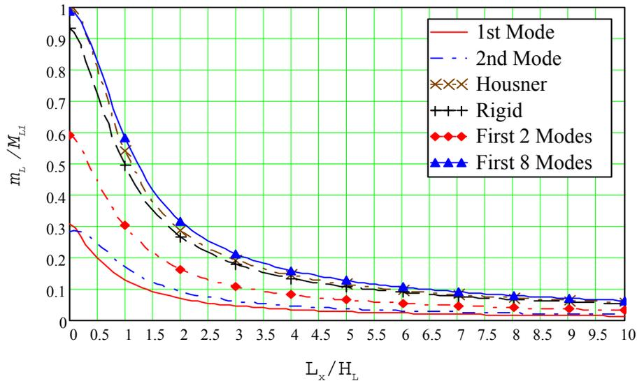
Figure 3 Ratio of Added Mass of Liquid due to Impulsive Hydrodynamic Pressure vs.  $L_x / H_L$
