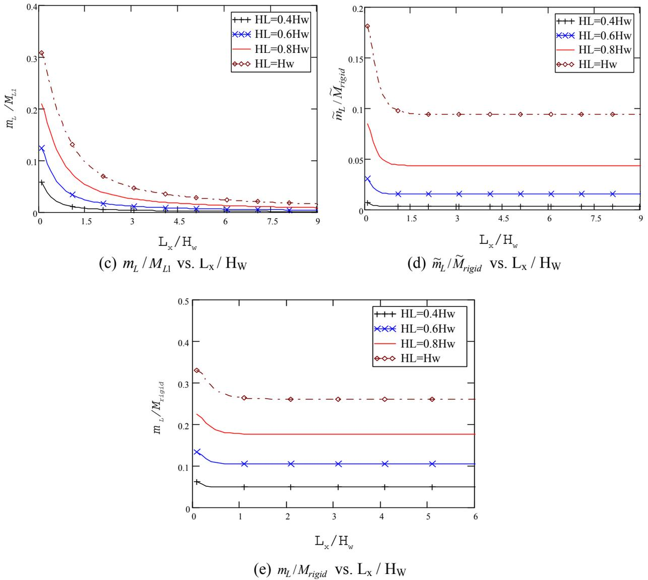
Figure 2 Effect of Liquid Level on Added Mass of Liquid
