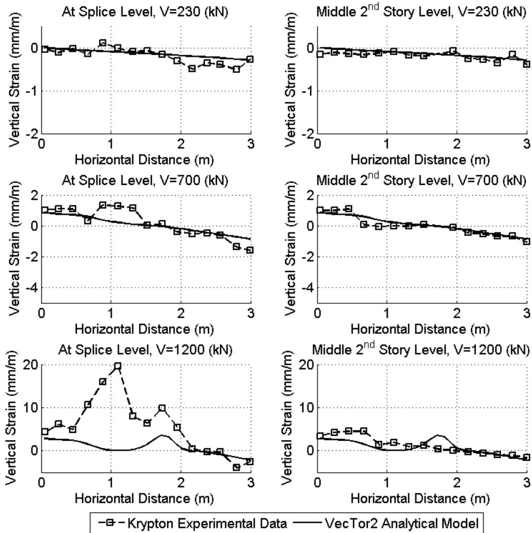
Figure 6. Vertical strain distribution comparison across the width of the wall.
