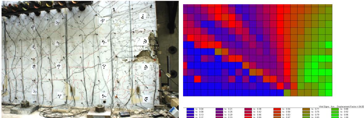
Figure 4. Comparison of distressed regions at failure.
