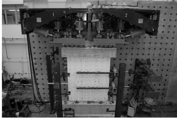
Figure 1. Planar wall test with two LBCBs and two side-mounted actuators
