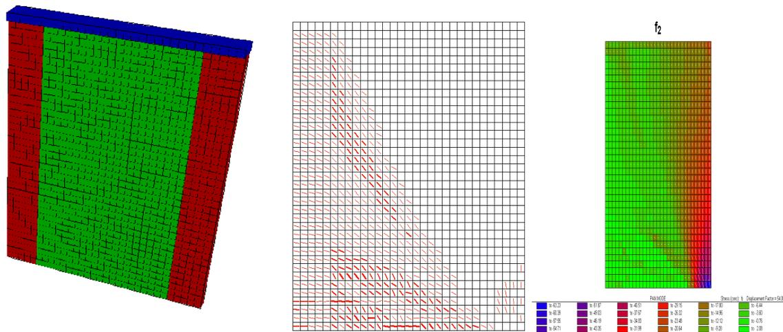
Figure 3. VecTor2 FEM model of planar RC wall. Cracked pattern at failure. Principal compression contour map.
