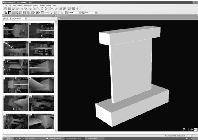
Figure 2. As built 3D rendering of wall specimen constructed with close-range photogrammetry
