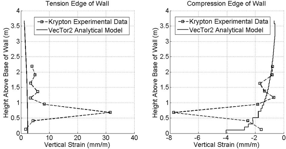
Figure 5. Comparison of region under high straining on compression and tension edge of wall ( $V = 1180$  kN)
