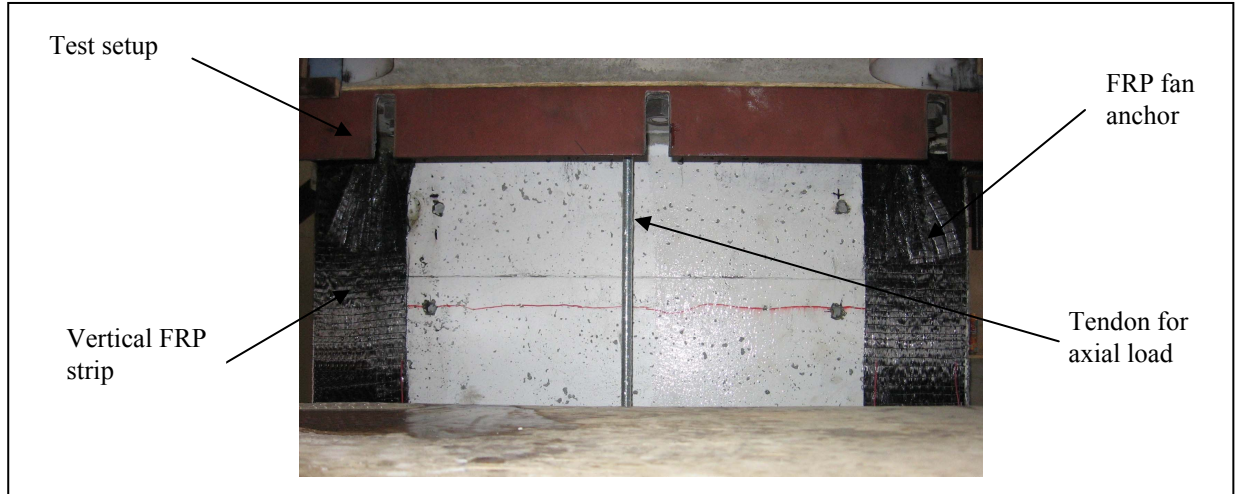
Figure 4. Vertical FRP strips and their FRP anchors at the 6 th floor panel before applying the horizontal CFP sheets.
