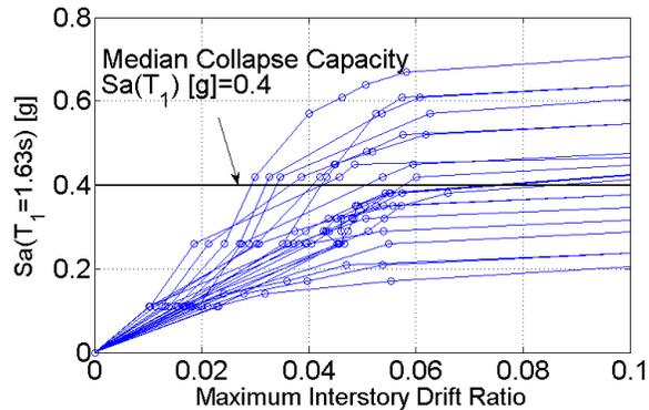
Figure 5. IDA results for 4-story partially-infilled RC frame.
