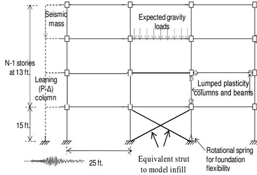
Figure 2. Nonlinear analysis model for RC frame building with masonry infill walls.
